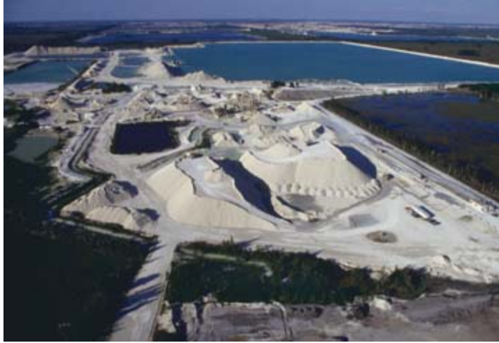
Stockpile of Limestone Materials from Adjacent Quarried Lakes
