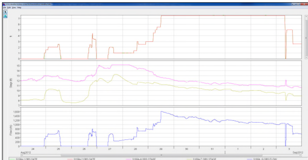
Figure 25. Observed Gate Openings, HW, TW and Flow at Structure S-155A
