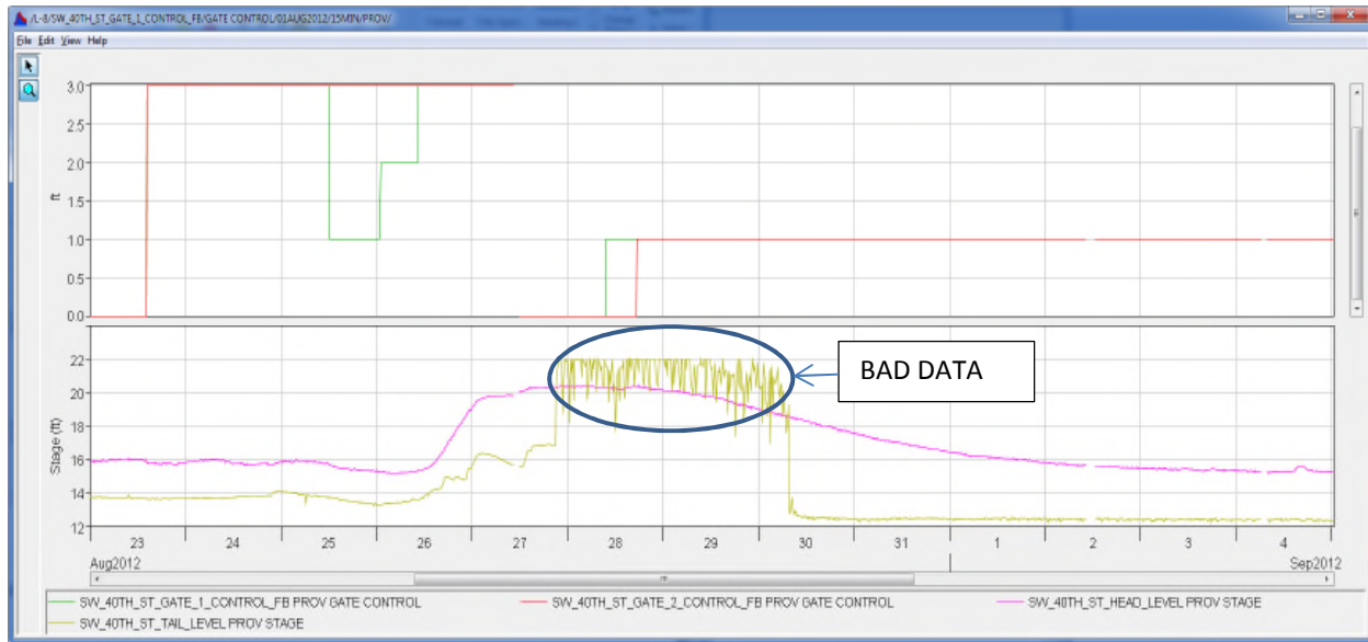
Figure 30. Observed Gate Openings, HW and TW Stage at ITID 40 th Street Structure
