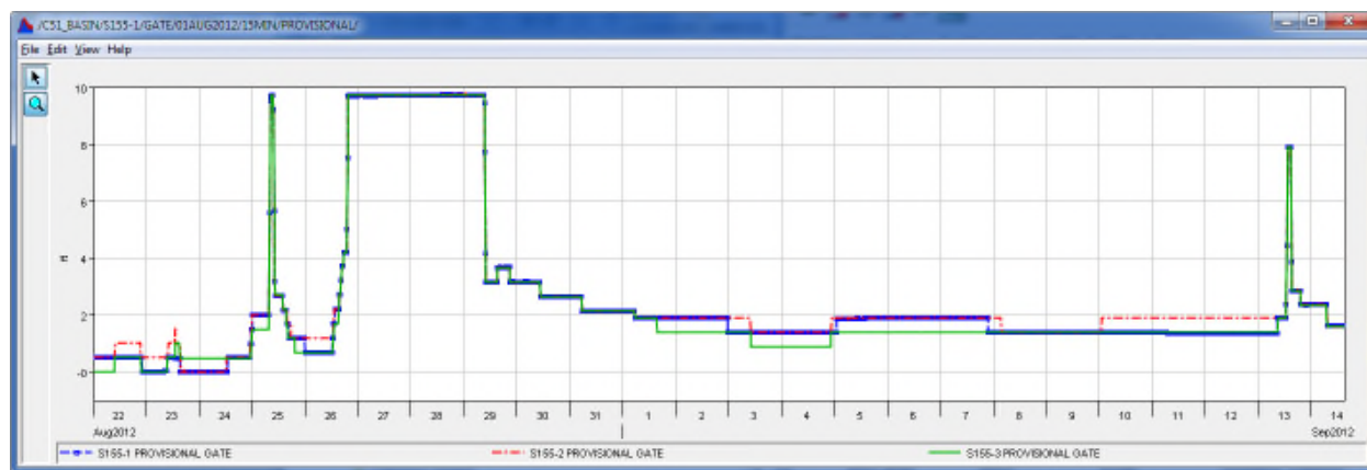
Figure 54. Observed Gate Openings for Structure S-155 during Tropical Storm Isaac
