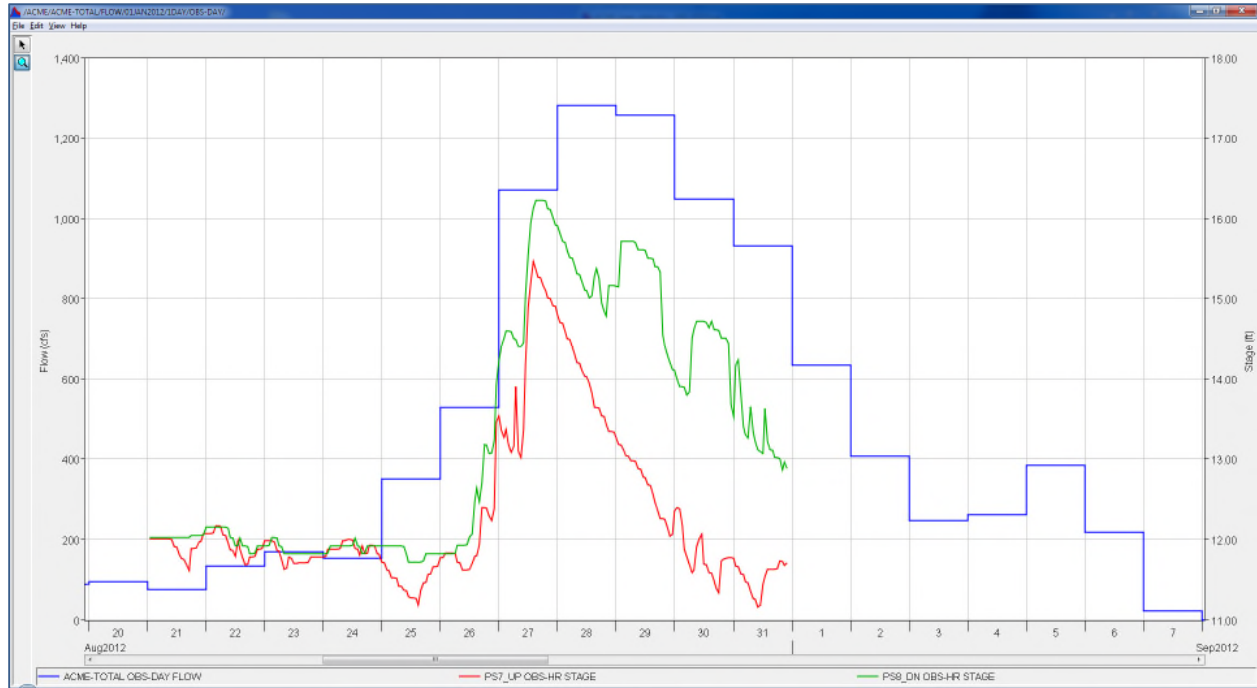
Figure 46. HW Stage of PS7 (red line), TW Stage of PS8 (green line) and Total ACME Pumpage (blue line) into the C-51 canal
