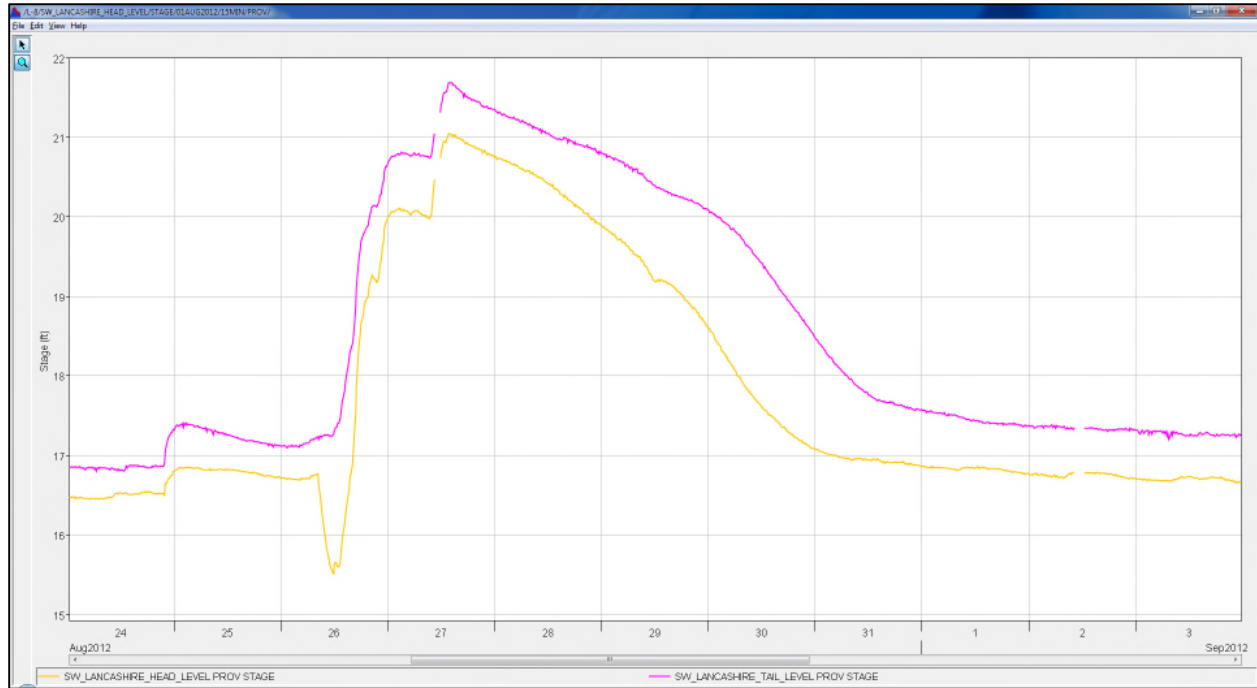
Figure 34. Observed HW and TW Stages at Lancashire Gauge
