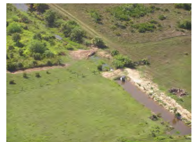
Culverts with risers for water management and with mud boards for sediment control
