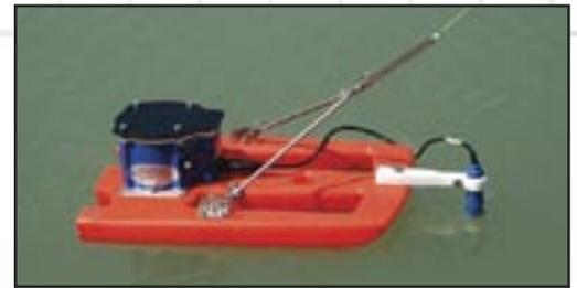
**Save time and money:** RDI's new **StreamPro ADCP** represents a revolutionary advancement in velocity and discharge measurement. Now you can accurately measure discharge in shallow streams in a matter of minutes—a fraction of the time required using traditional handheld devices. With StreamPro there's no need to move from station to station to obtain single-point velocity data or compute the discharge by hand; discharge measurements are obtained in real time.
