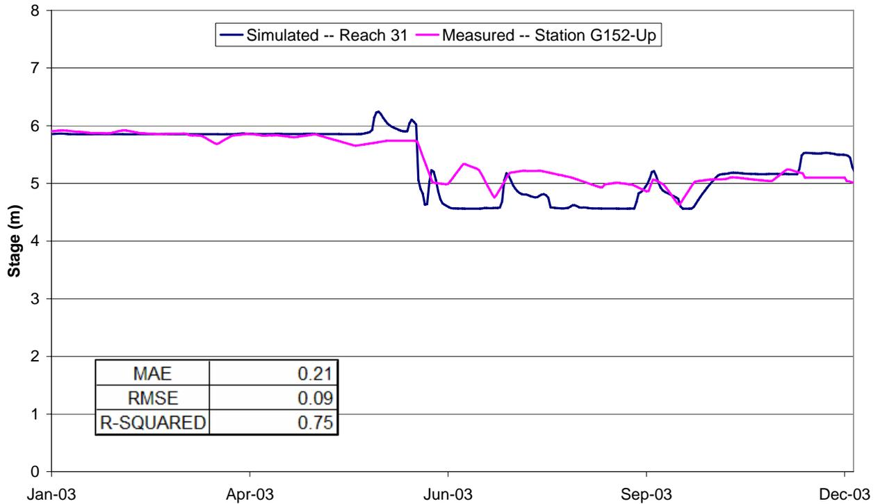
**Figure 4.100: Validation stages upstream of G-152 (west) for 2003**
