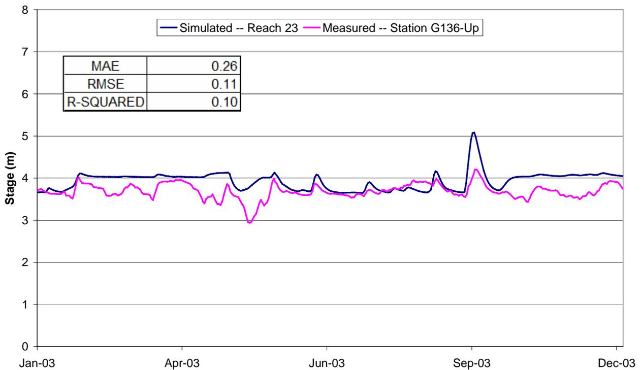
**Figure 4.89: Validation stages upstream of G-136 (west) for 2003**
