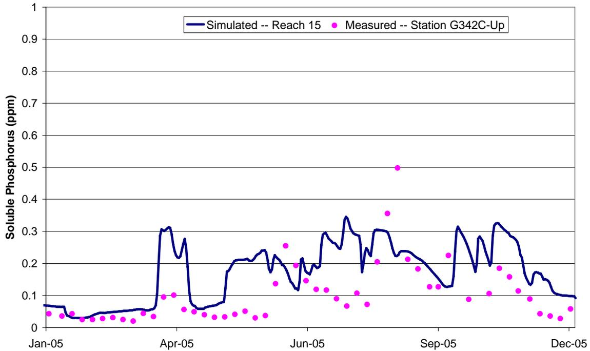
**Figure 4.81: Calibration Soluble P concentration for G-342C in 2005**
