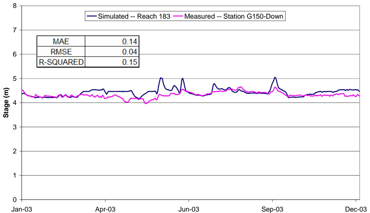
**Figure 4.95: Validation stages downstream of G-150 (south) for 2003**
