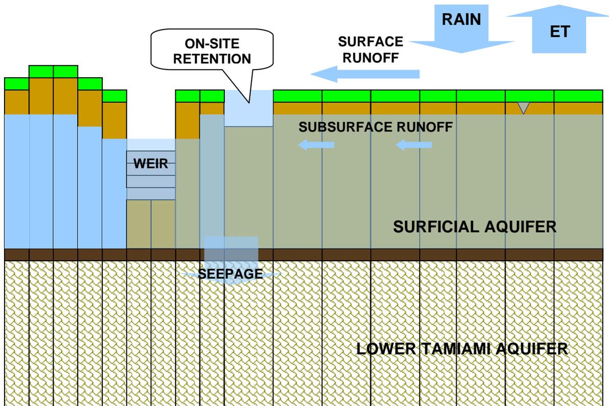
**Figure 3.25: Conceptual application of a retention BMP**
