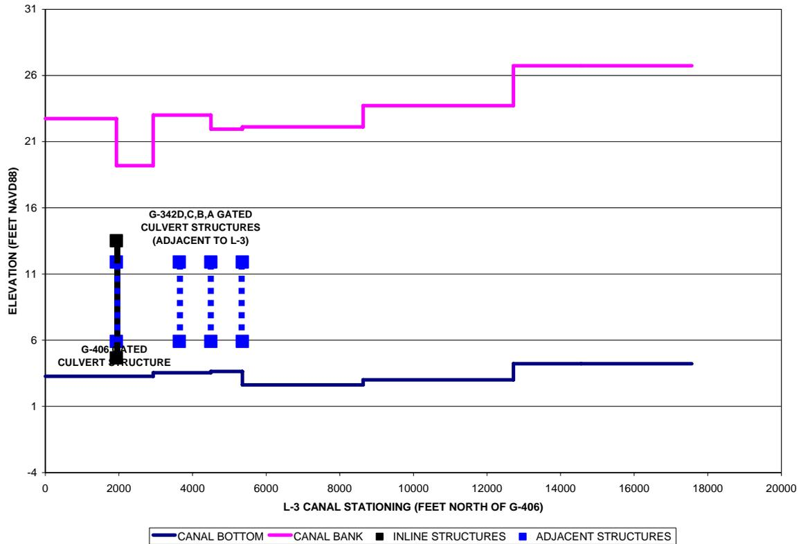
Figure 3.16: L-3 Canal Bottom and Bank Profile
