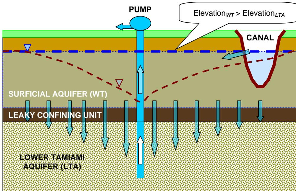
Figure 3.19: Transitional subsurface conditions during the dry season
