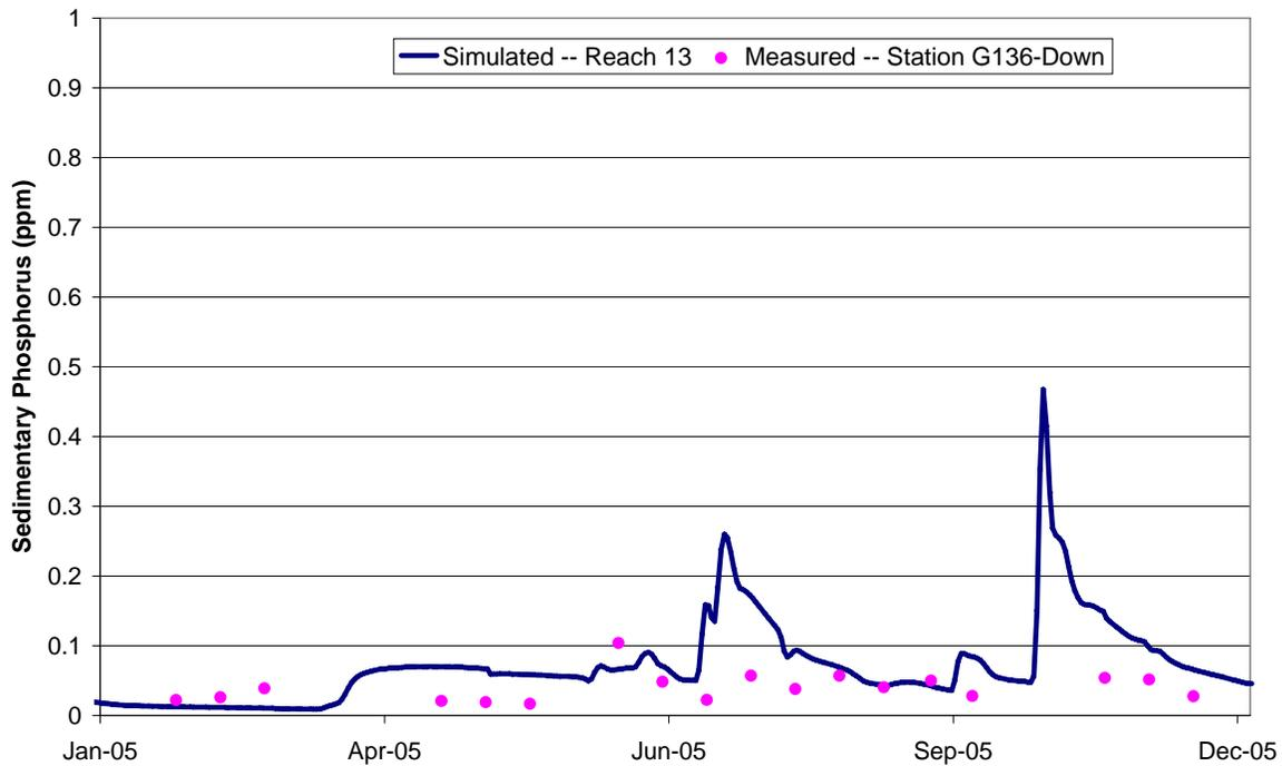
**Figure 4.78: Calibration Sedimentary P concentration for G-136 in 2005**
