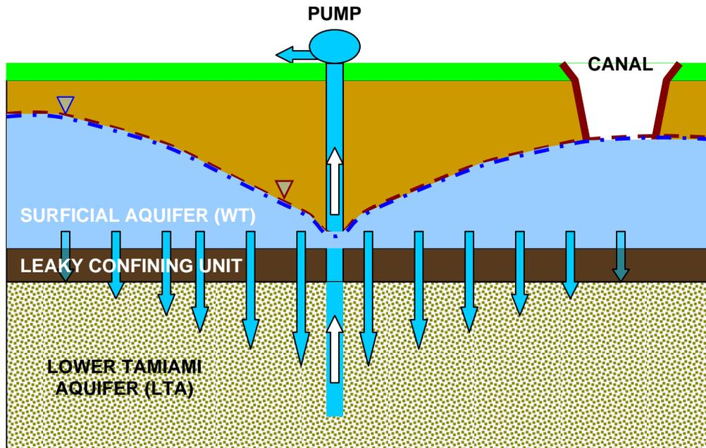
Figure 3.20: Potential impacts of steady-state pumping during the dry season
