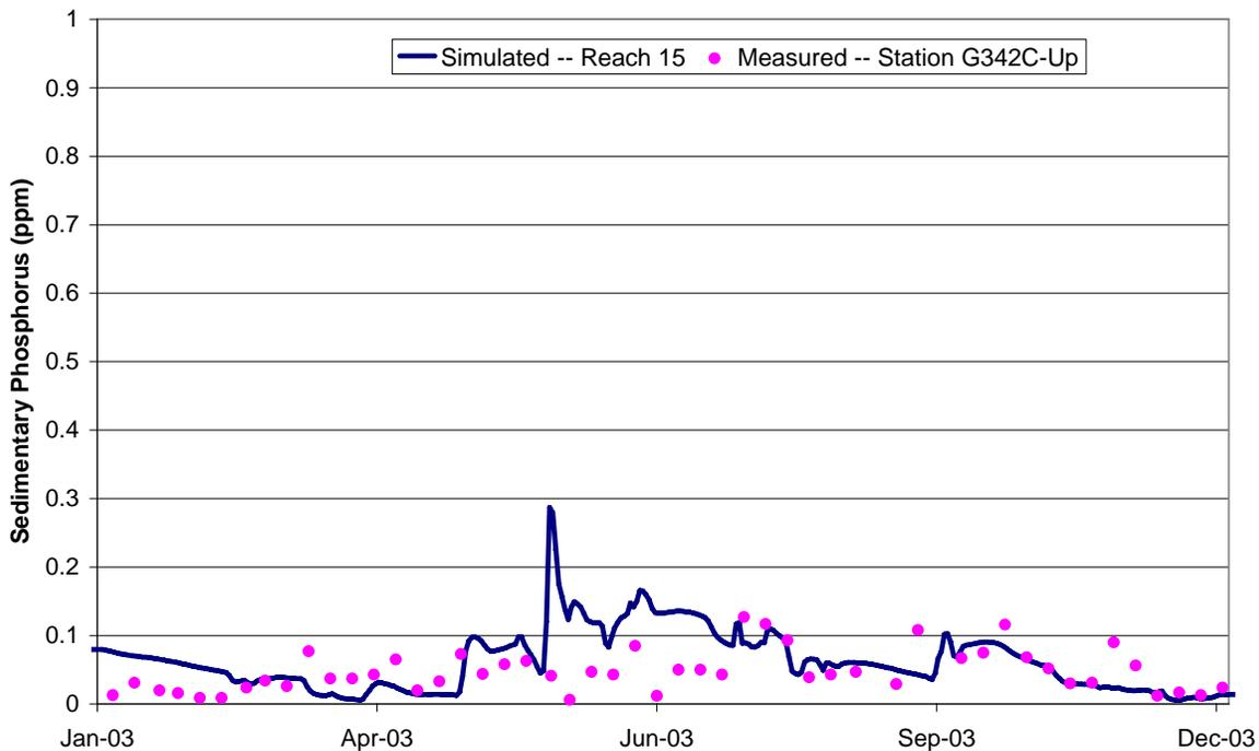
**Figure 4.111: Validation Sedimentary P concentration for G-342C in 2003**
