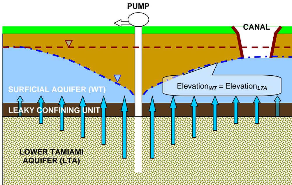
Figure 3.21: Transitional subsurface conditions after dry season pumping
