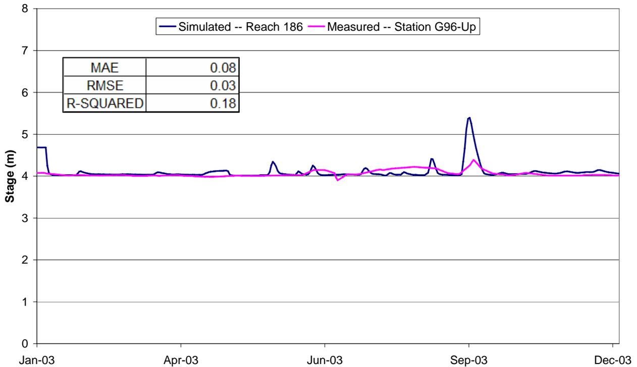
**Figure 4.91: Validation stages upstream of G-96 (west) for 2003**
