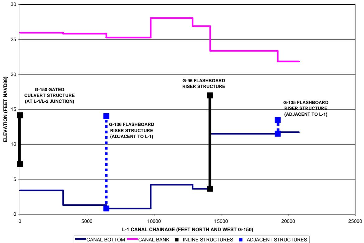
**Figure 3.10: L-1 Canal Bottom and Bank Profile**
