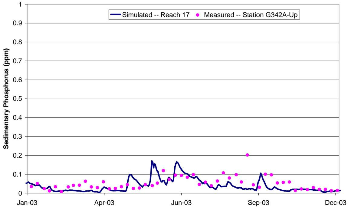
**Figure 4.109: Validation Sedimentary P concentration for G-342A in 2003**
