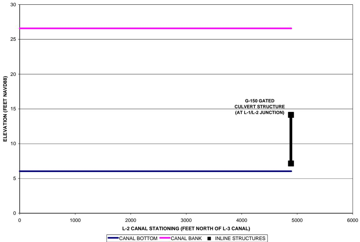
**Figure 3.12: L-2 Canal Bottom and Bank Profile**
