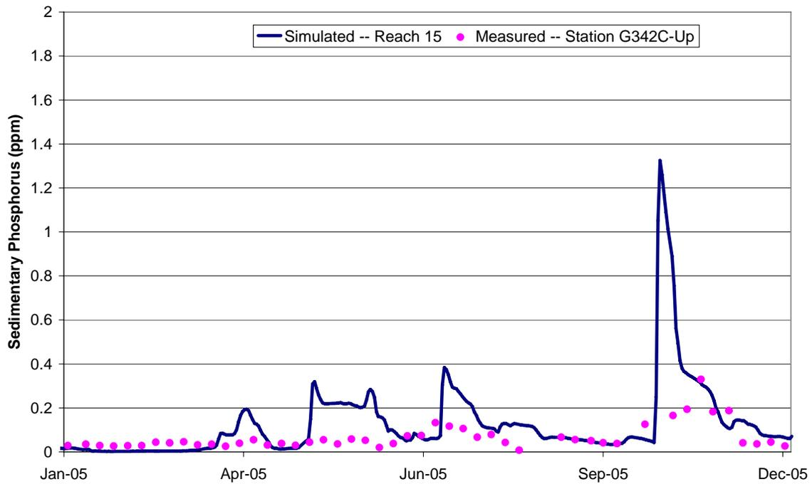
**Figure 4.82: Calibration Sedimentary P concentration for G-342C in 2005**
