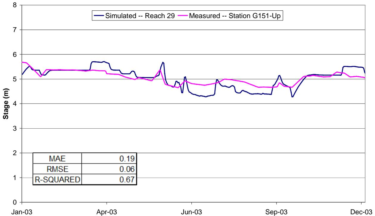
**Figure 4.97: Validation stages upstream of G-151 (west) for 2003**
