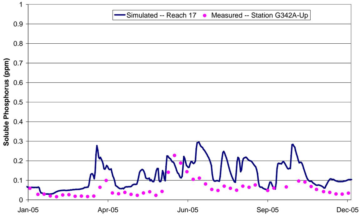
**Figure 4.79: Calibration Soluble P concentration for G-342A in 2005**
