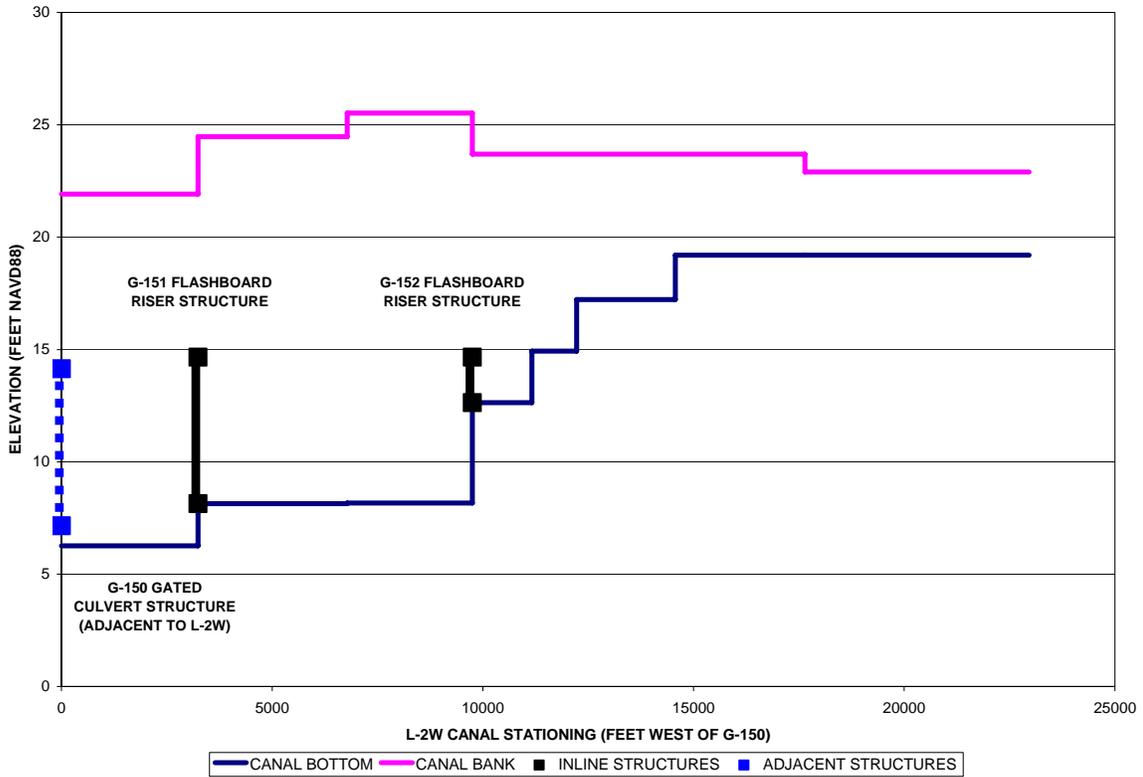
Figure 3.14: L-2W Canal Bottom and Bank Profile
