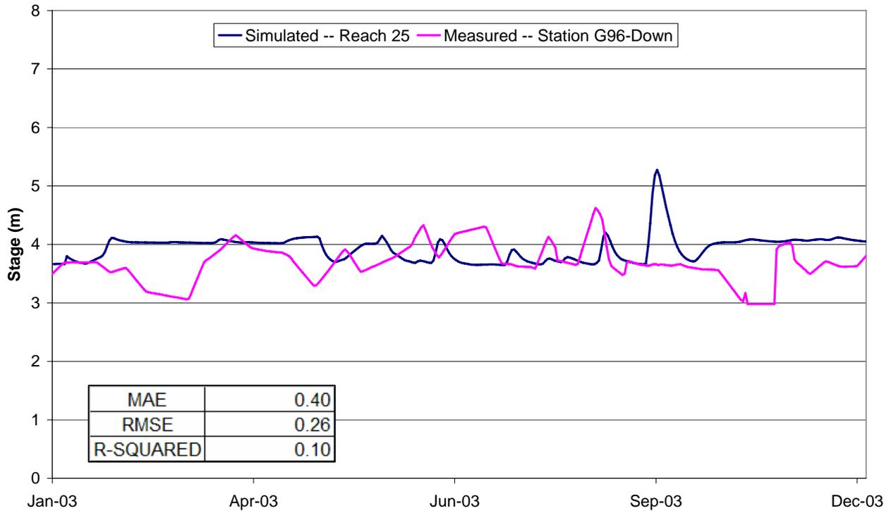
**Figure 4.92: Validation stages downstream of G-96 (east) for 2003**
