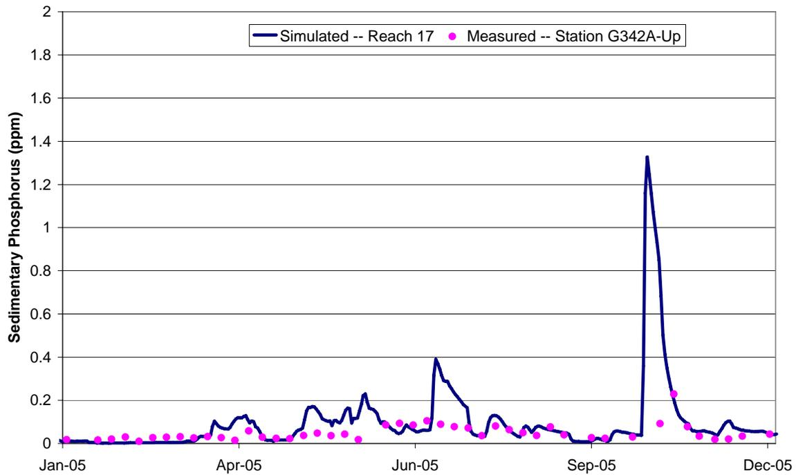
**Figure 4.80: Calibration Sedimentary P concentration for G-342A in 2005**
