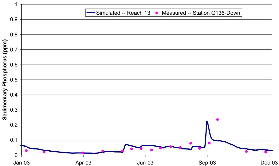
**Figure 4.107: Validation Sedimentary P concentration for G-136 in 2003**
