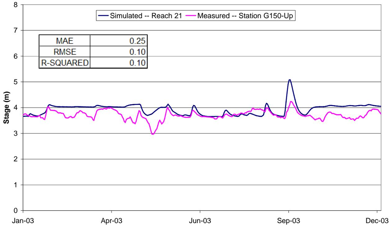
**Figure 4.94: Validation stages upstream of G-150 (north) for 2003**
