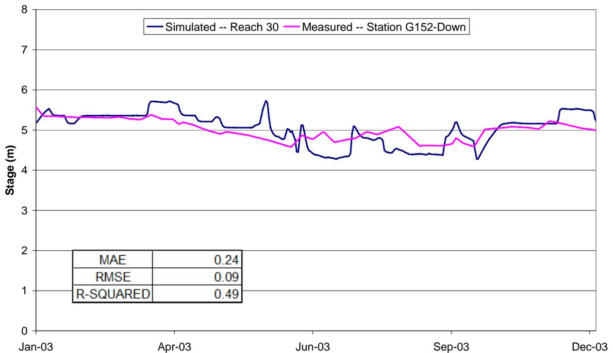
**Figure 4.101: Validation stages downstream of G-152 (east) for 2003**
