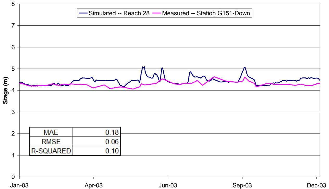
**Figure 4.98: Validation stages downstream of G-151 (east) for 2003**
