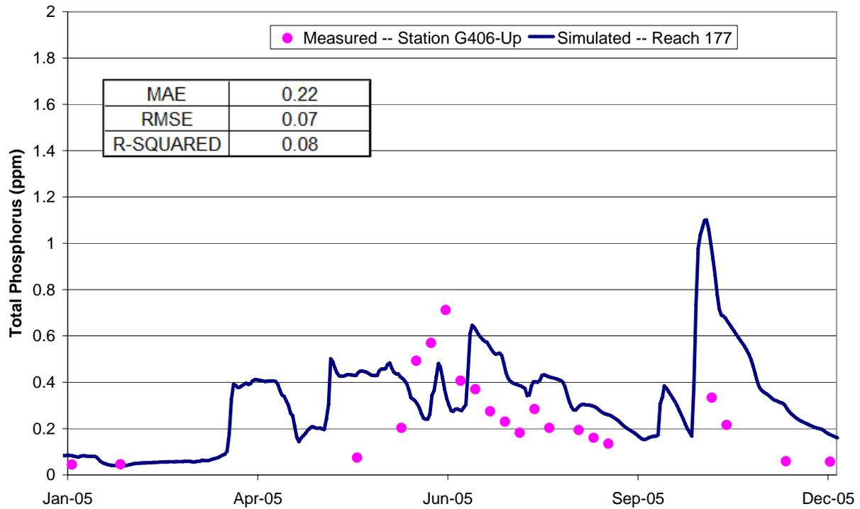
**Figure 4.76: Calibration TP concentration for G-406 in 2005**
