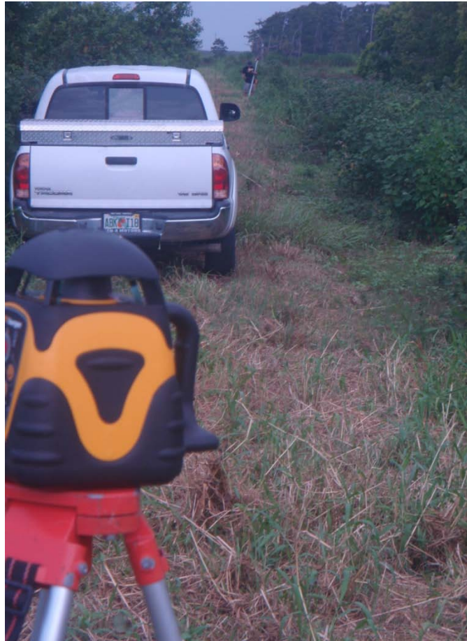
Figure 5. Survey of ground elevations on a berm bordering AGI3 on August 23, 2012. The CST Berger laser level is shown in the foreground.
