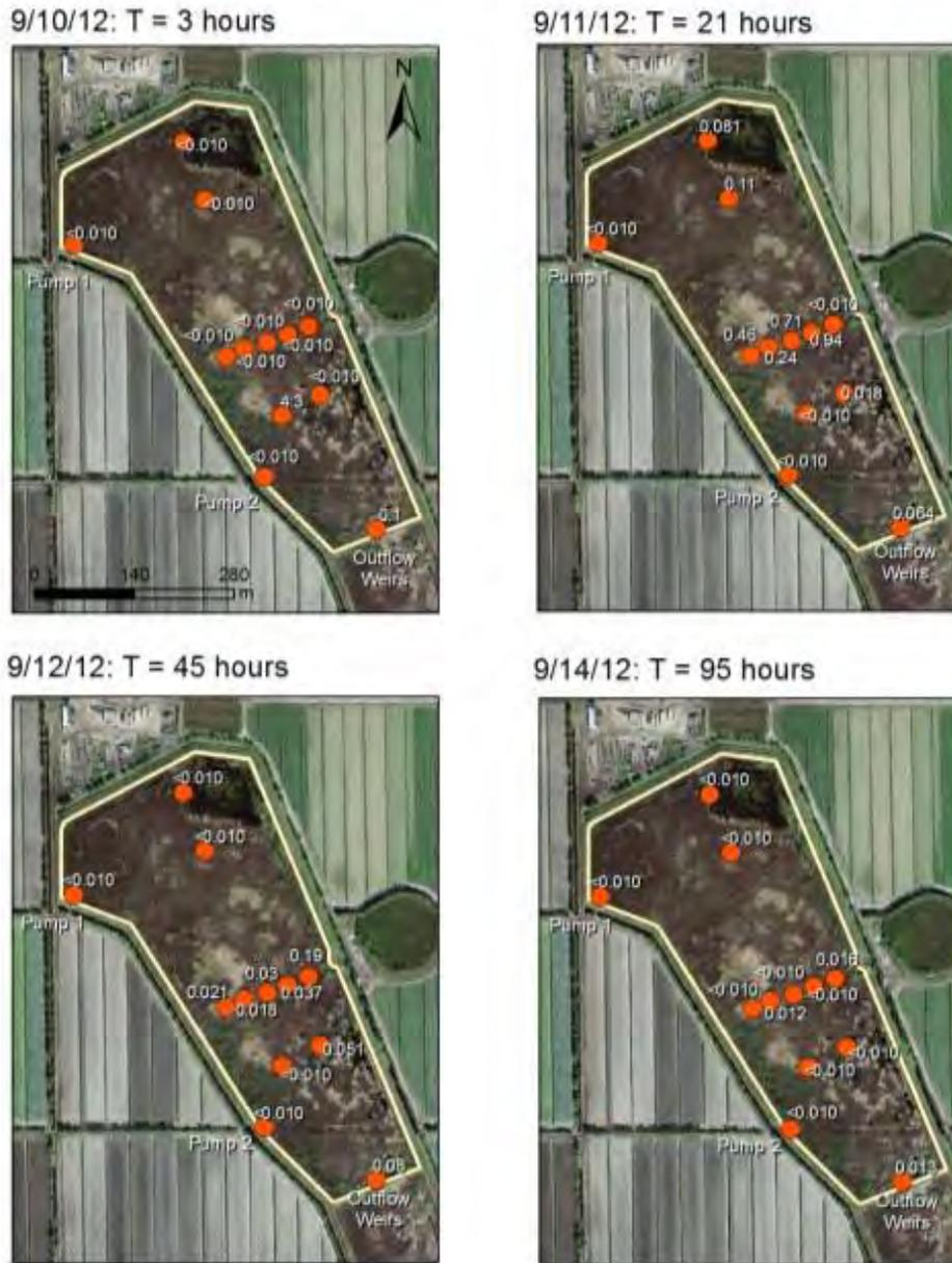
**Figure 15.** Spatial distribution of lithium (Li) concentrations (mg/L) in the surface waters of AGI1 after 3, 21, 45 and 95 hours after Li tracer injection. A value of <0.010 mg/L indicates the concentration was below the method detection limit of 0.010 mg/L.
