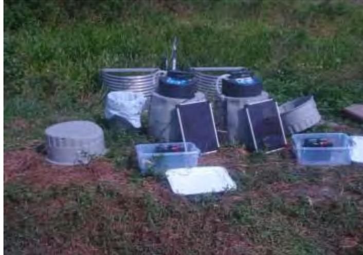
**Figure 11.** Twin ISCO portable samplers powered by batteries and solar panels were deployed at the outflow weirs (shown in the background).
