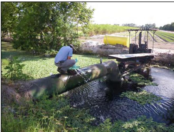
**Figure 4.** Inflow pump calibration being performed by the field personnel during the AGI1 investigation performed by Shukla et al. (2011).
