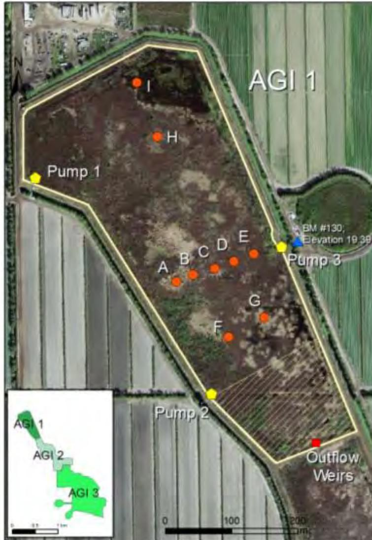
**Figure 5.** Locations of Pump Nos. 1 - 3, the outflow weir, and the internal stations (A-I) in AGI1. The pulse tracer (LiCl) injection and hydraulic loading characterization during the study were performed only at Pump Nos. 1 and 2. The cross-hatched area in the southern part of AGI1 represents the area assumed to receive discharge from Pump No. 2. The Benchmark #130, elevation 19.39 NGVD29, was used as the datum for survey points collected in AGI1 by DB Environmental, Inc.
