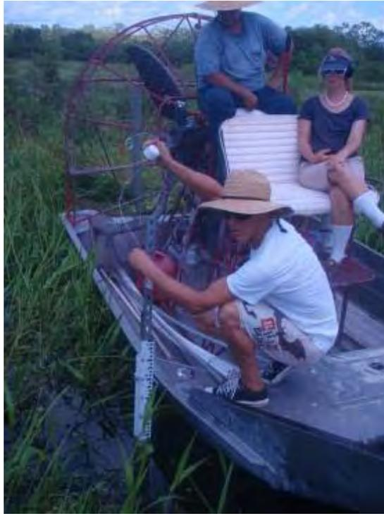
**Figure 8.** Deployment of the pressure transducer near the outflow weirs of AGI1 on September 6, 2012.
