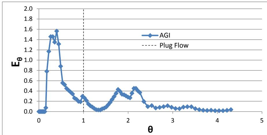
**Figure 16.** Tracer response curve at the outflow of AGI1 where  $\theta$  (dimensionless) is the time after tracer injection normalized to the nominal retention time (0.94 day) and  $E_\theta$  (also dimensionless) is the tracer concentration normalized to the mass of tracer injected (22.41 kg Li). A  $\theta$  of 1 is equal to one nominal HRT.
