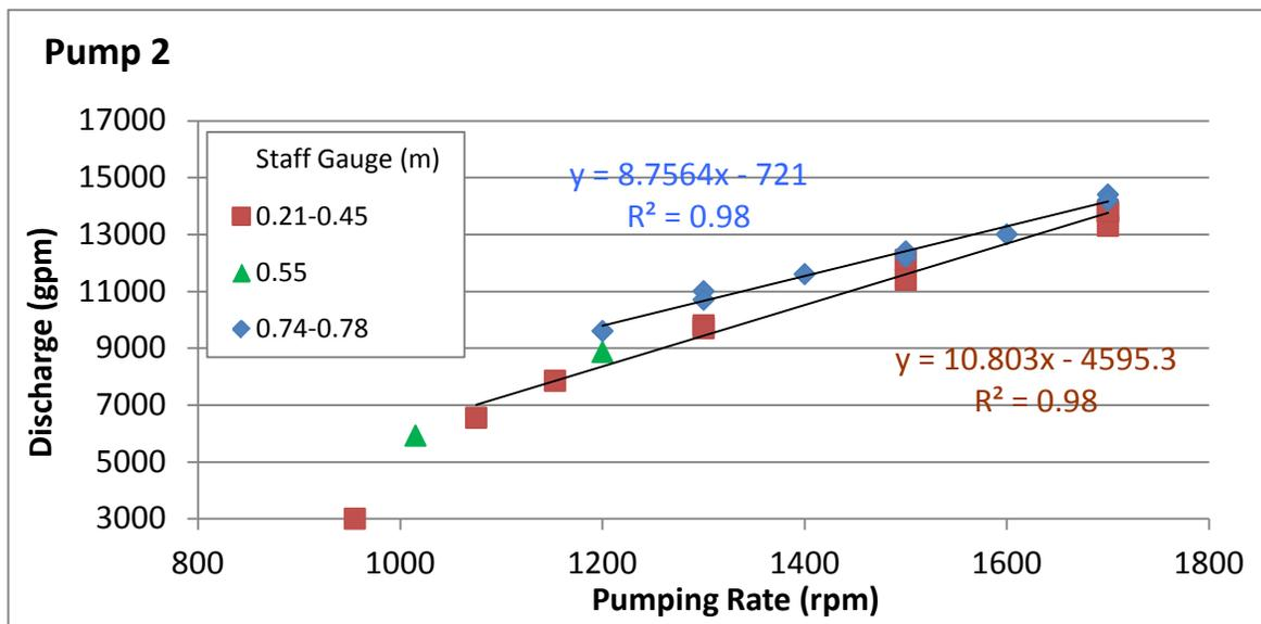
**Figure 12.** Pump regression equations predicting discharge volume (gallons per minute (gpm)) as a function of pump revolutions per minute (rpm) and stage for Pump Nos. 1 and 2 at AGI1. The two regression lines shown for each pump represent the relationship between pumping rate and discharge for water elevations of 0.74-0.78 m (2.43-2.56 ft) (upper line) and 0.20-0.57 m (0.66-1.87 ft) (lower line) in the supply canal.
