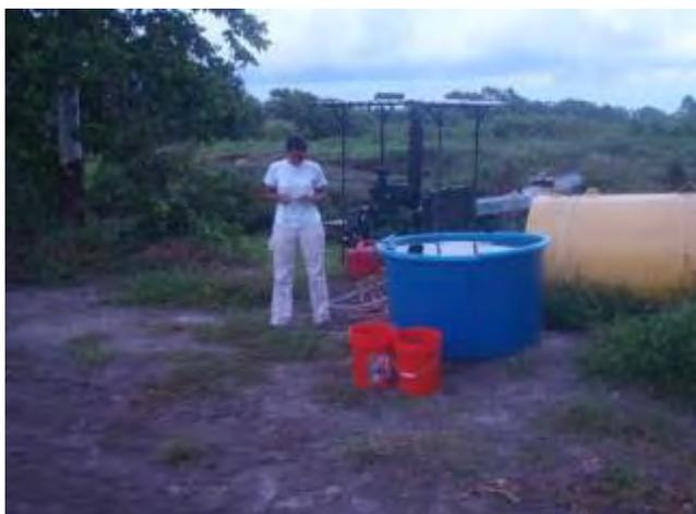
**Figure 9.** Infrastructure for delivering the LiCl tracer to the pipe in Pump No. 1. The blue tub contained 220 gallons of diluted (1:8) concentrated LiCl solution. The 5-gal orange buckets contained supply canal water used for rinsing the blue tub of residual LiCl after nearly all of it was pumped to the inflow pipe.
