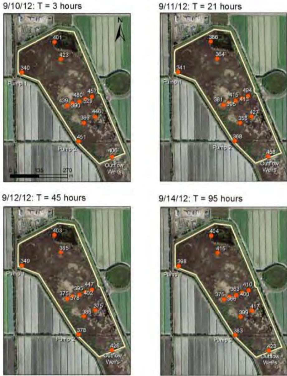
**Figure 17.** Spatial distribution of total phosphorus concentrations ( $\mu\text{g/L}$ ) in the surface waters of the basic impoundment (AGI1) 3, 21, 45 and 95 hours after lithium tracer injection.
