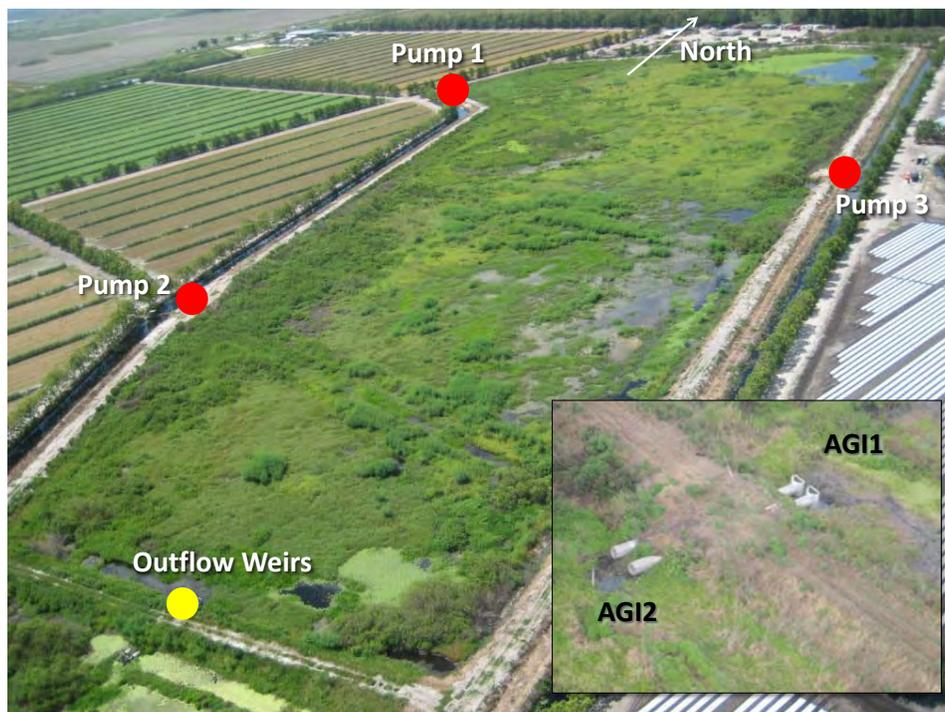
**Figure 3.** Aerial photo of AGI1 showing the three inflow pump stations and the outflow weirs. The inset is a photo of the outflow weirs. The pulse tracer (lithium chloride) injection and hydraulic loading characterization during the study were performed only at Pump Nos. 1 and 2. Tracer and total phosphorus concentrations were monitored in the surface waters at the inflow pumps, outflow weirs and at internal stations (Figure 5).
