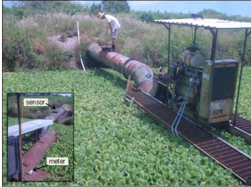
**Figure 6.** Flow calibration at Pump 2 on August 3, 2012. The inset shows the flow sensor inserted into the pipe of Pump 1 and the meter indicating flow in gallons per minute.
