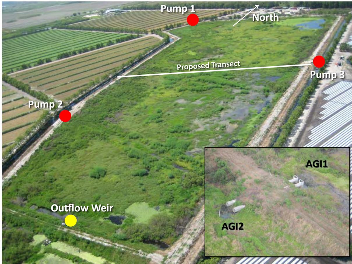
**Figure 3.** Aerial photo of AGI1 showing the three inflow pump stations, the outflow weirs, and the proposed internal sampling transect. Inset is of the outflow weirs. Tracer injection will occur only at Pumps 1 and 2, and monitored at the outflow weirs and along the proposed transect (if feasible).
