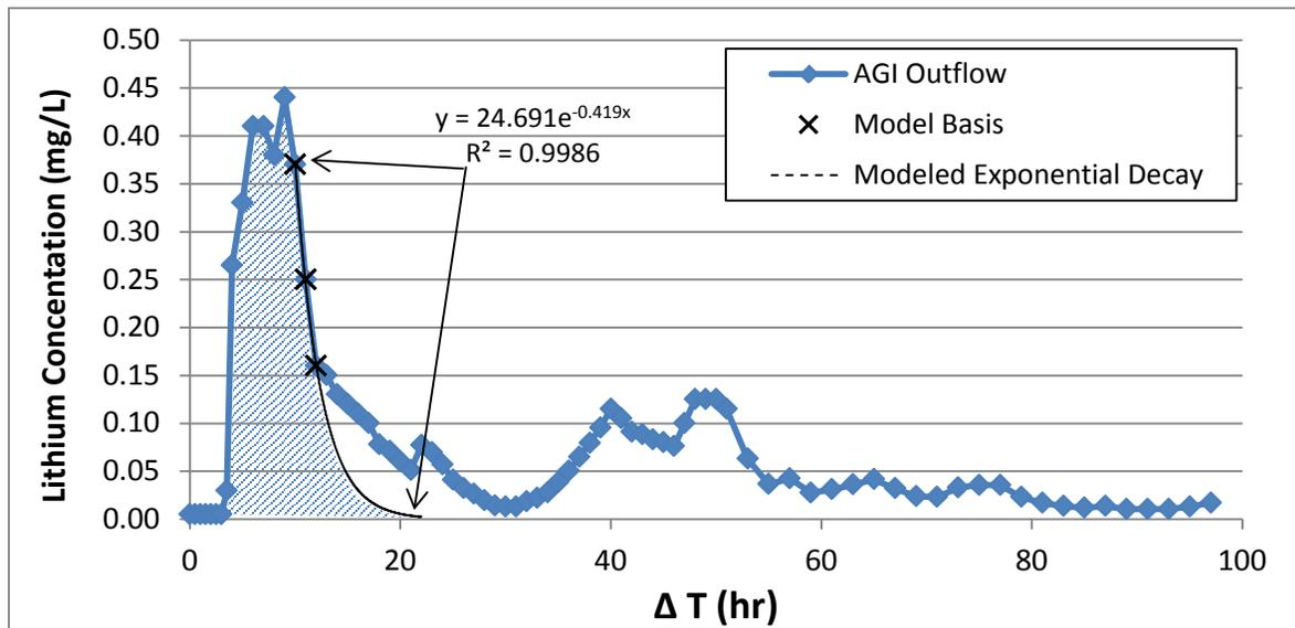
**Figure 14.** Concentration of lithium tracer measured at the outflow weirs for elapsed times after tracer injection ( $T = 0$ ) at 12:05 on September 10, 2012. Values represent means of duplicate autosamplers, except between 17:05 on September 10 and 09:05 on September 11, when samples were collected from only one autosampler. The dashed line is the extrapolated exponential decay of the descending limb of the first peak in the hydrograph, which is assumed to be contributed from only Pump No. 2
