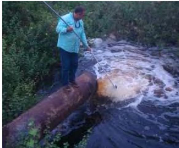
**Figure 10.** Sampling the discharge from the inflow pump for total phosphorus analysis.
