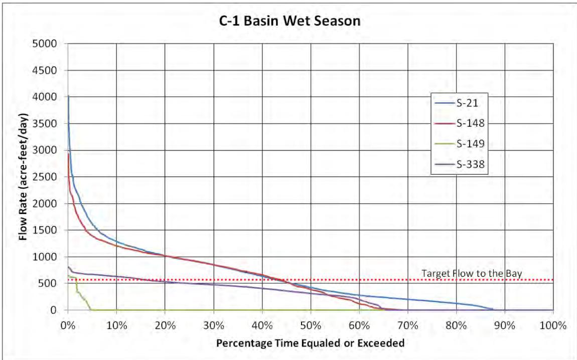
Figure C-8. Flow duration curves for the C-1 basin water control structures during the wet season.
