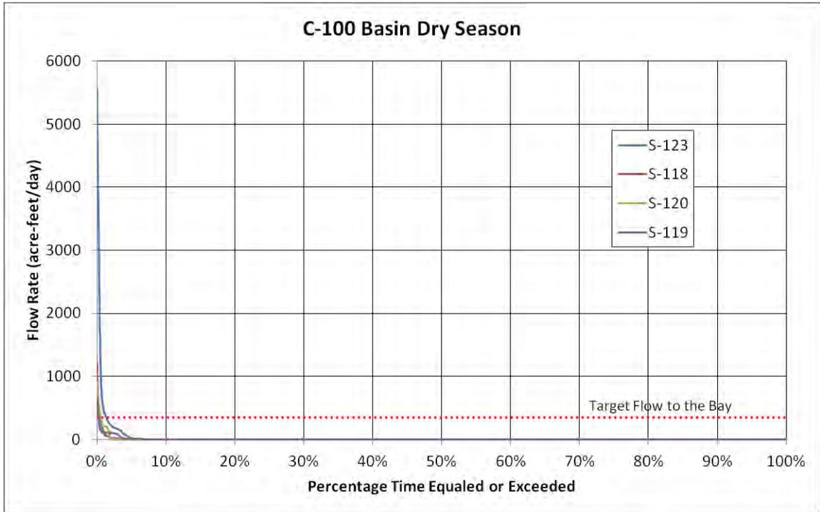
Figure C-3. Flow duration curves for C-100 basin water control structures during the dry season.
