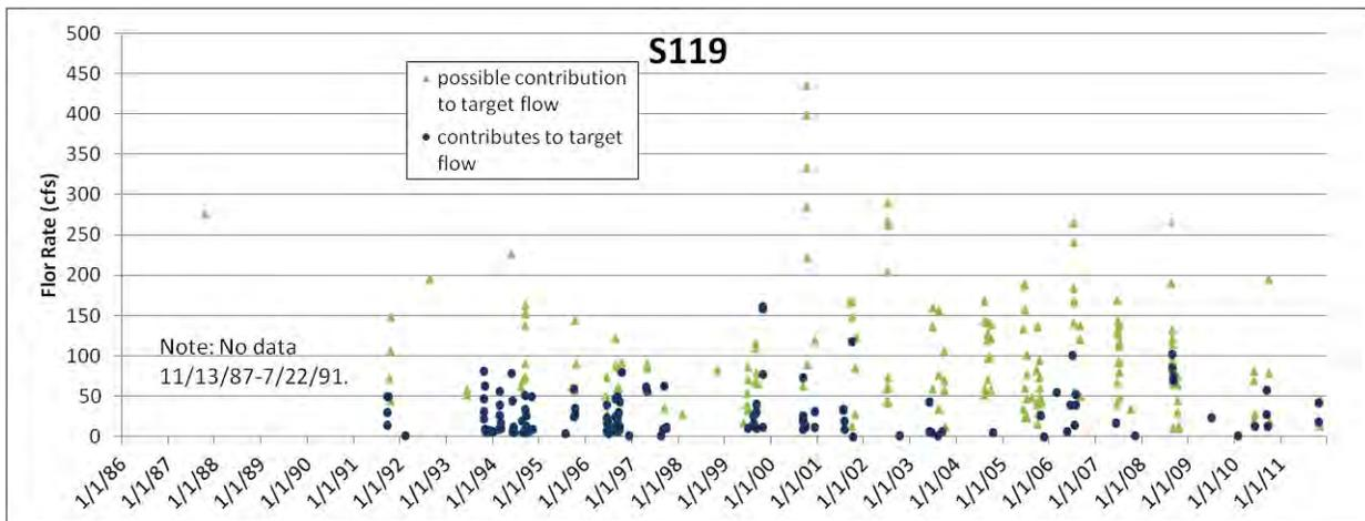
Figure C-6. S-119 water flow contributions toward target flow at S-123.
