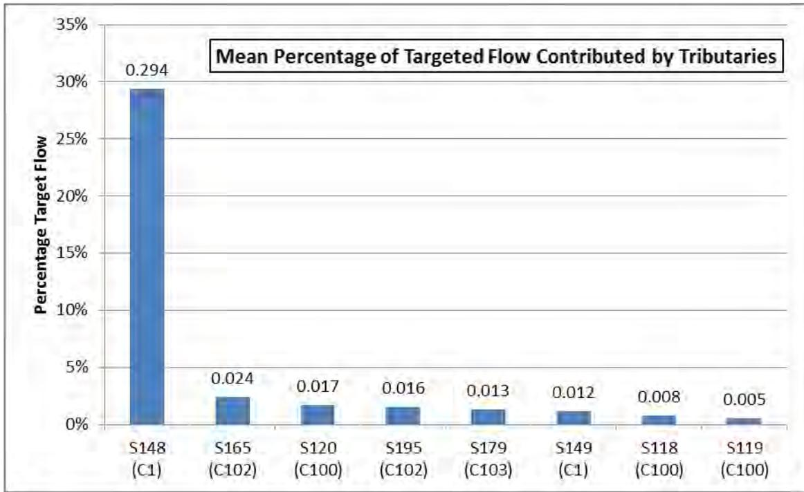
Figure C-28. Ranked estimated percentage of maximum mean daily flow passing through tributary structures that contributed toward individual outfall flow targets. Structures are given on the X axis with the basin in parentheses below.
