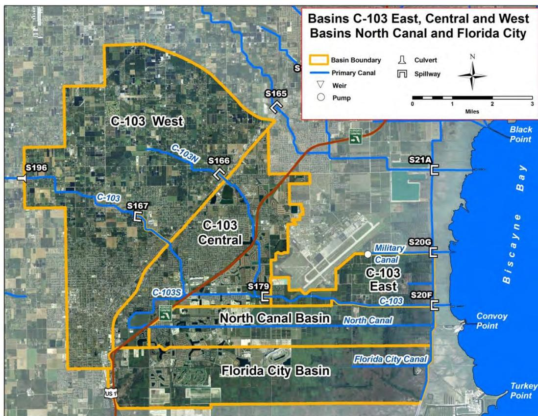
**Figure 12.** Map of the C-103 basin (shaded area) with associated primary canals.
