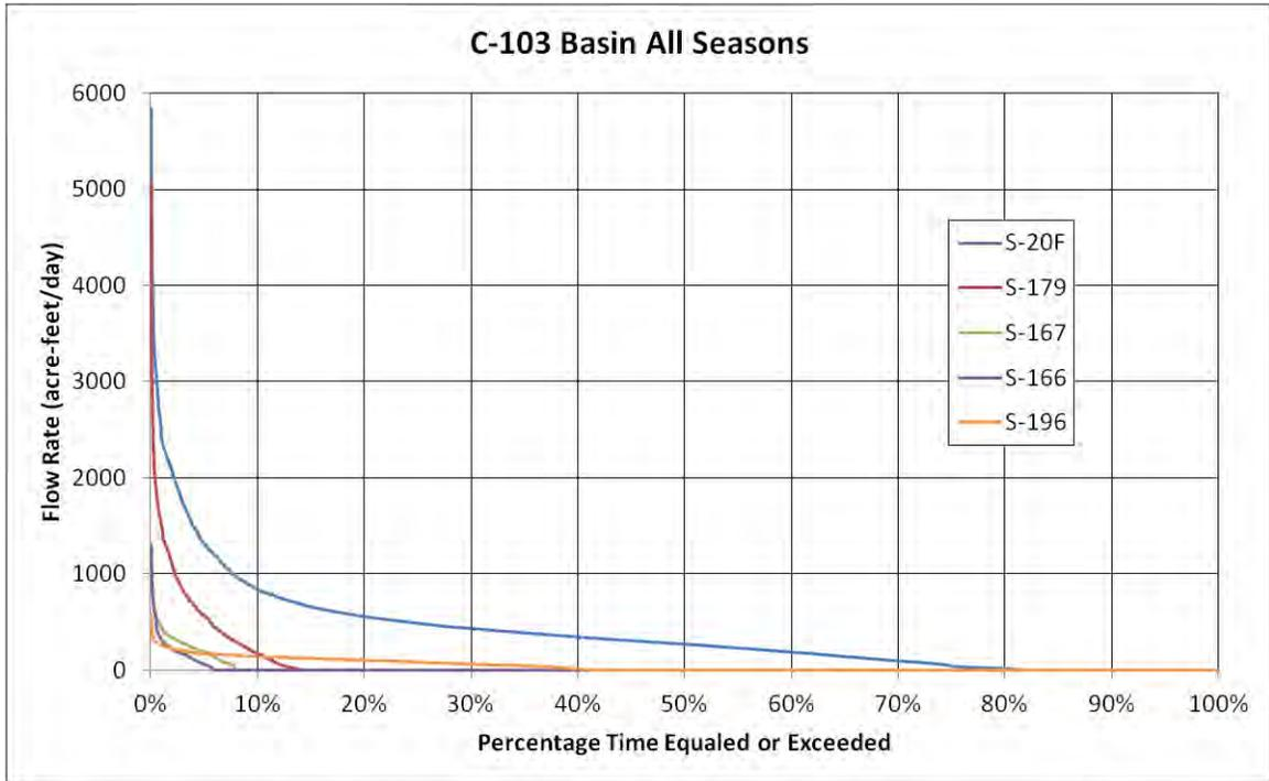
Figure C-21. Flow duration curves for the C-103 basin water control structures during all seasons.
