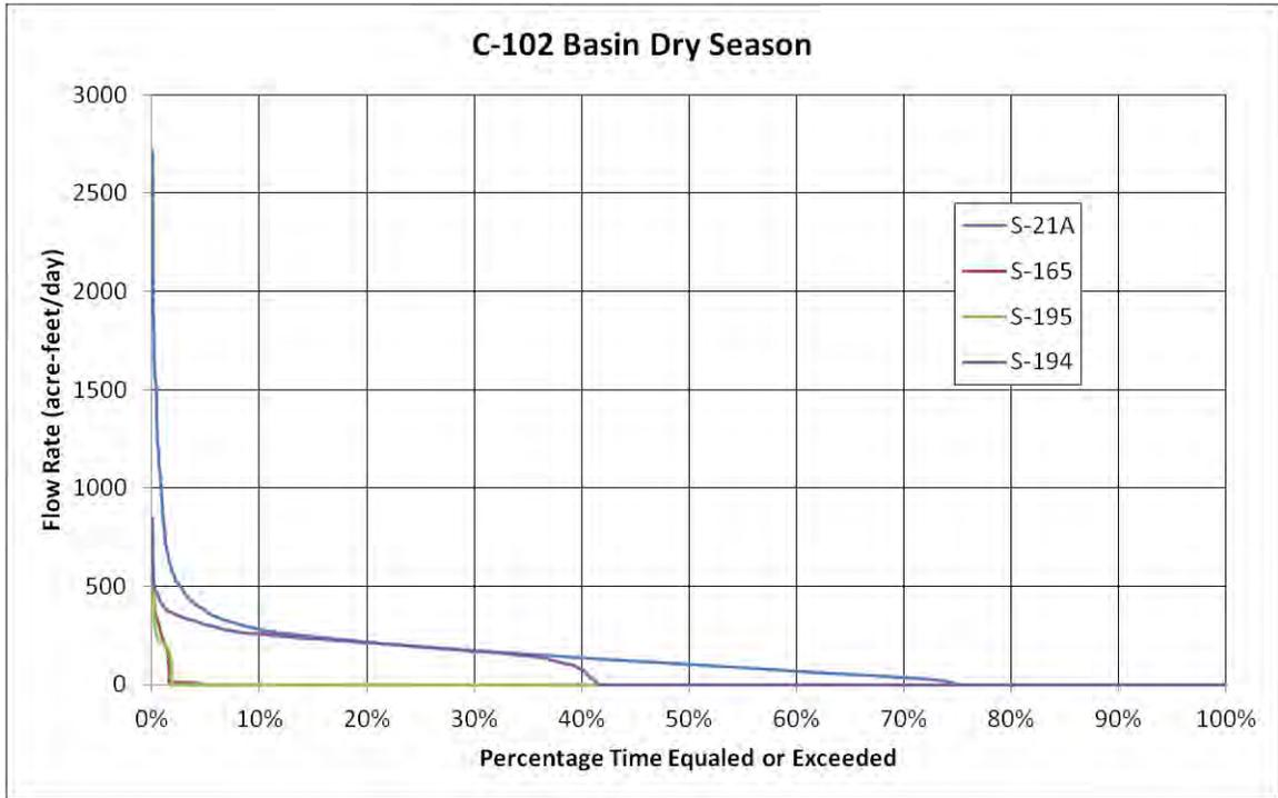
Figure C-15. Flow duration curves for the C-102 basin water control structures during the dry season.
