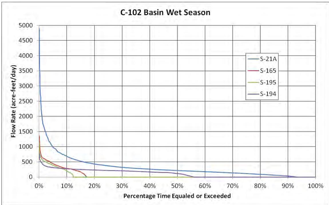
Figure C-14. Flow duration curves for the C-102 basin water control structures during the wet season.
