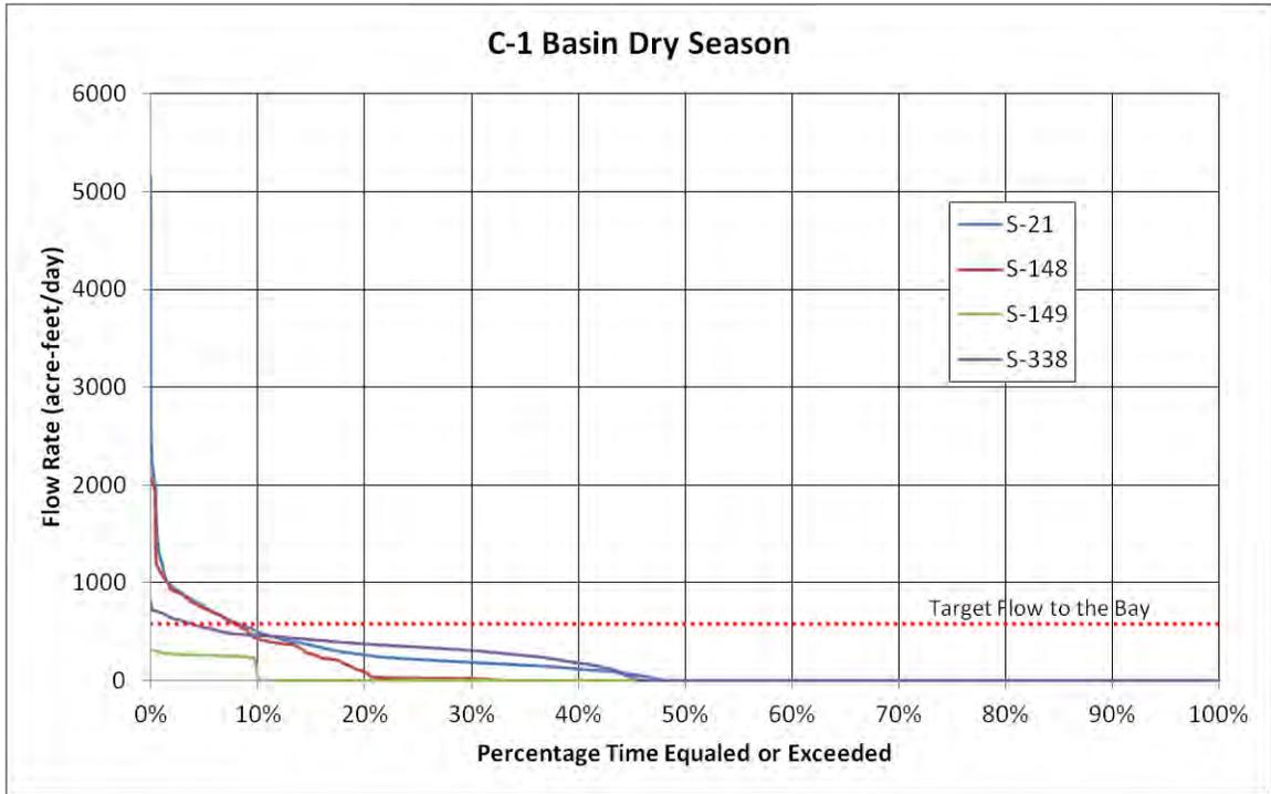
Figure C-9. Flow duration curves for the C-1 basin water control structures during the dry season.
