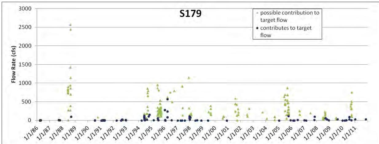
Figure C-24. S-179 water flow contributions toward an approximated target flow at S-20F.
