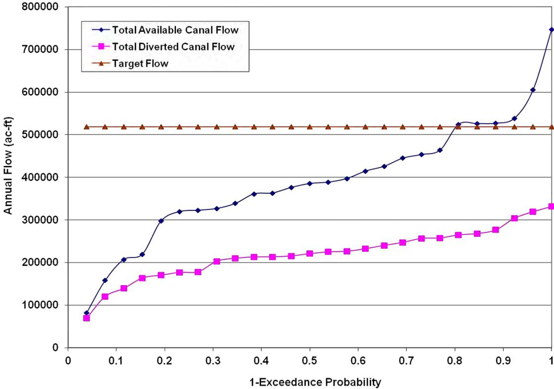
Figure 4. Updated (1986–2011) plot of annual canal discharges and diverted water from the BBCW PIR.
