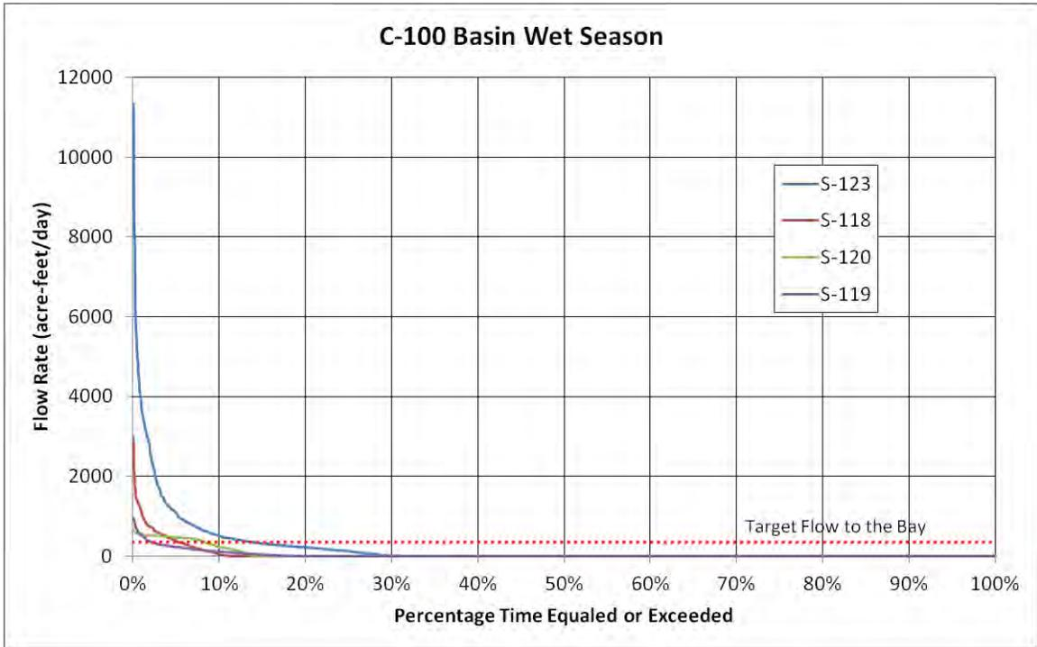
Figure C-2. Flow duration curves for C-100 basin water control structures during the wet season.
