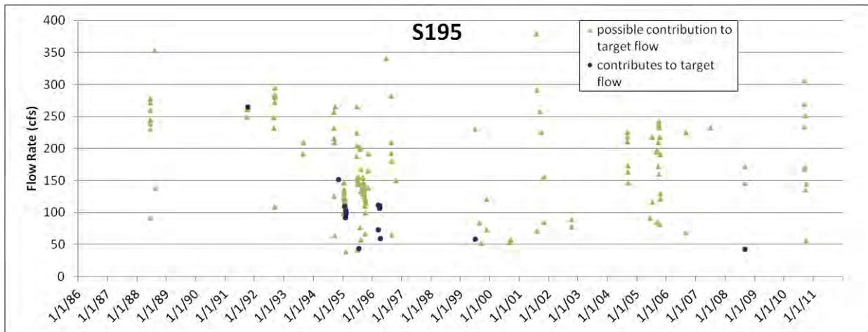
Figure C-16. S-195 water flow contributions toward an approximated target flow at S-21A.
