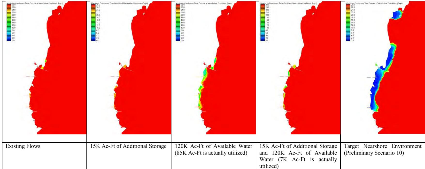
Figure 18: 21 Creek Simulation Comparison: Maximum Continuous Time Outside of Mesohaline Range (Days)
