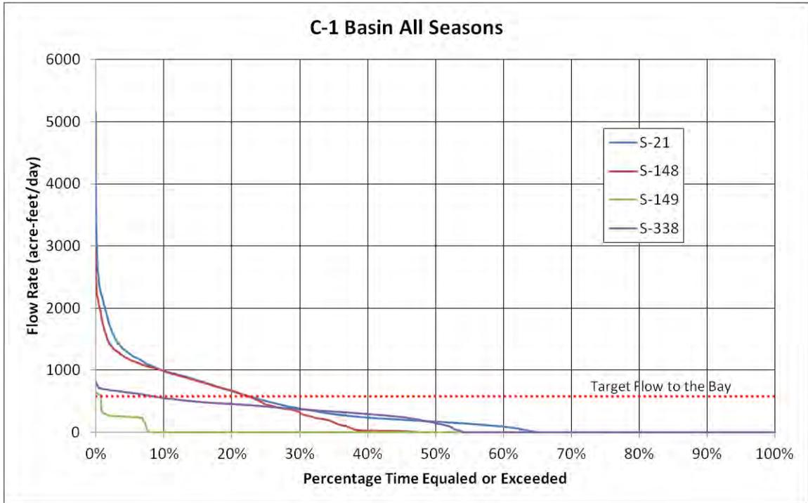
Figure C-7. Flow duration curves for the C-1 basin water control structures during all seasons.
