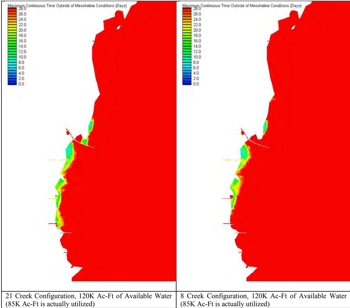
Figure 19: Comparison of 21 Creek Configuration and 8 Creek Configuration: Maximum Continuous Time Outside of Mesohaline Range (Days)
