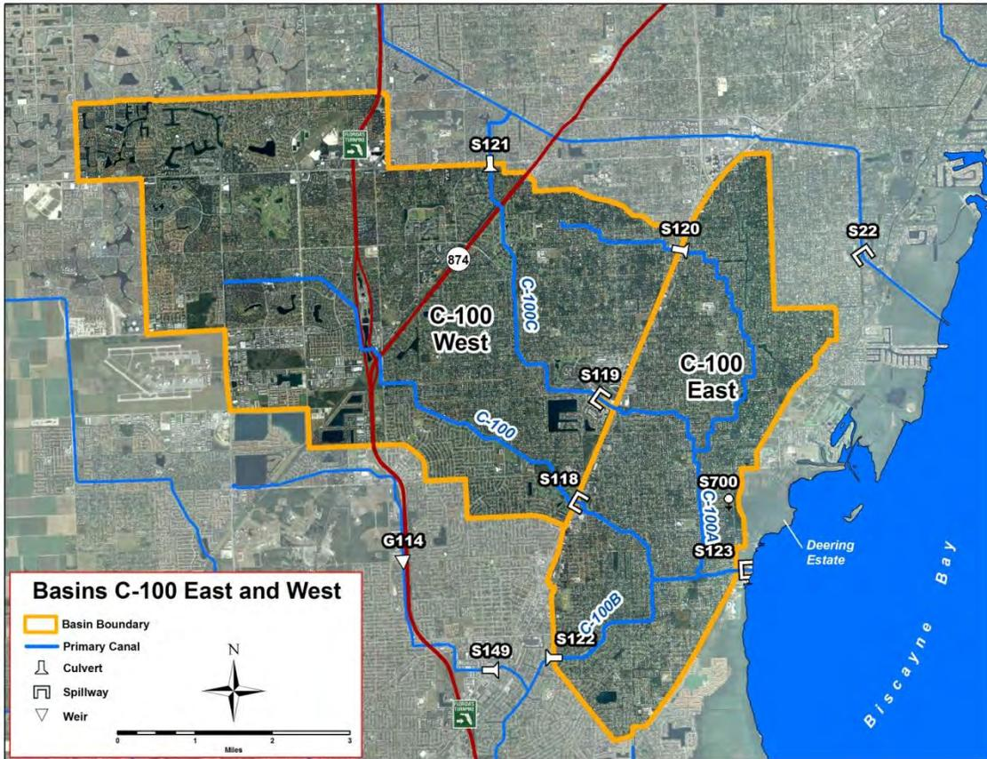
Figure 7. Map of the C-100 basin (shaded area) with associated primary canals.
