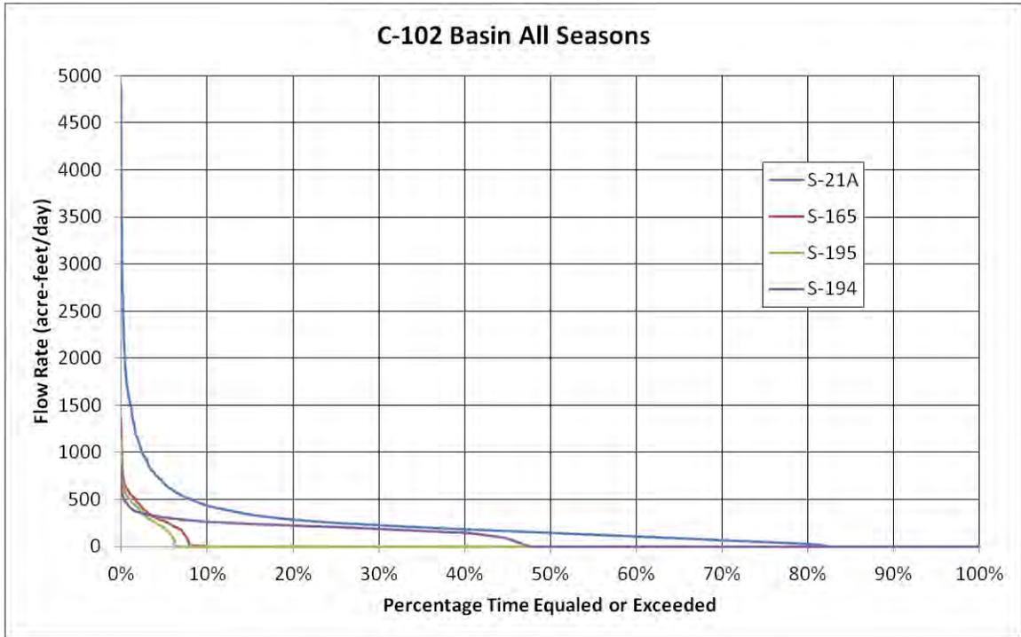
Figure C-13. Flow duration curves for the C-102 basin water control structures during all seasons.
