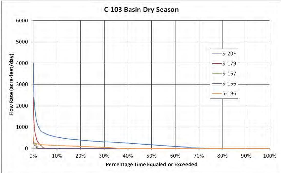
Figure C-23. Flow duration curves for the C-103 basin water control structures during the dry season.
