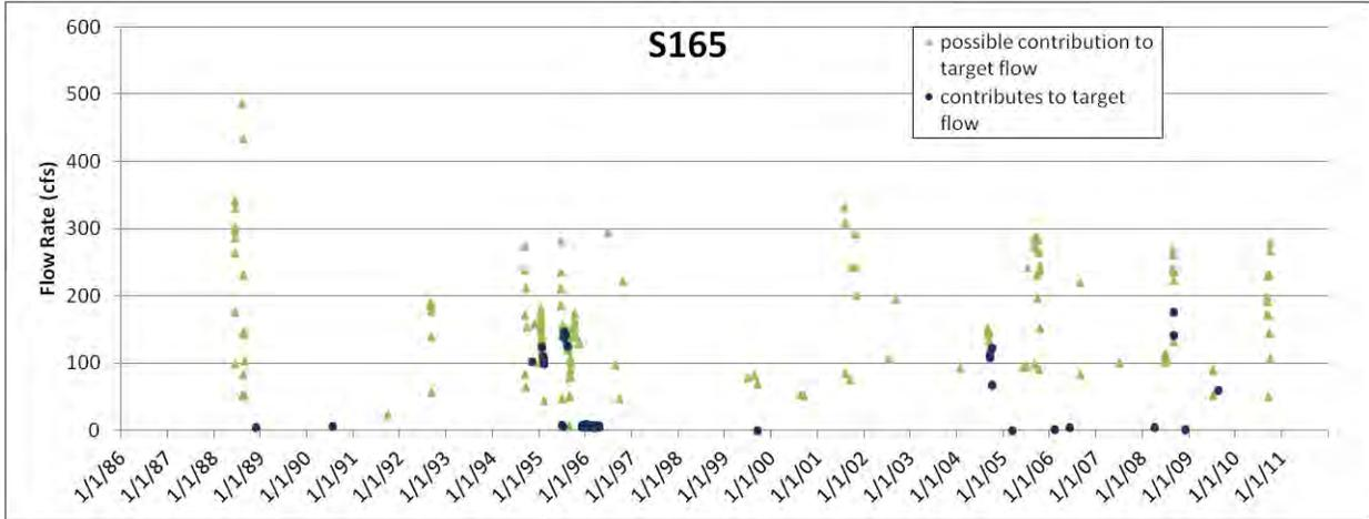
Figure C-17. S-165 water flow contributions toward an approximated target flow at S-21A.
