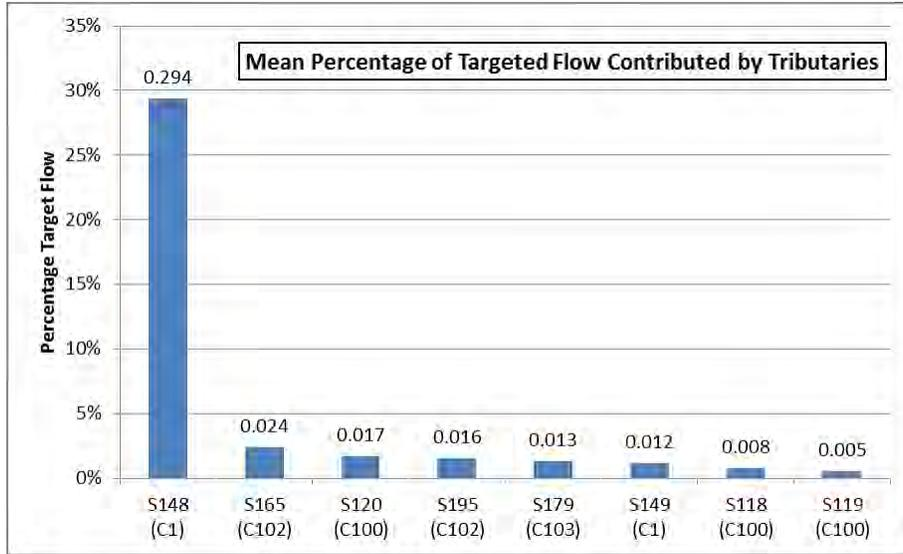
**Figure 8.** Ranked estimated percentage of maximum mean daily flow passing through tributary structures that contributed toward individual outfall flow targets. Structures are given on the X axis with the basin in parentheses below.
