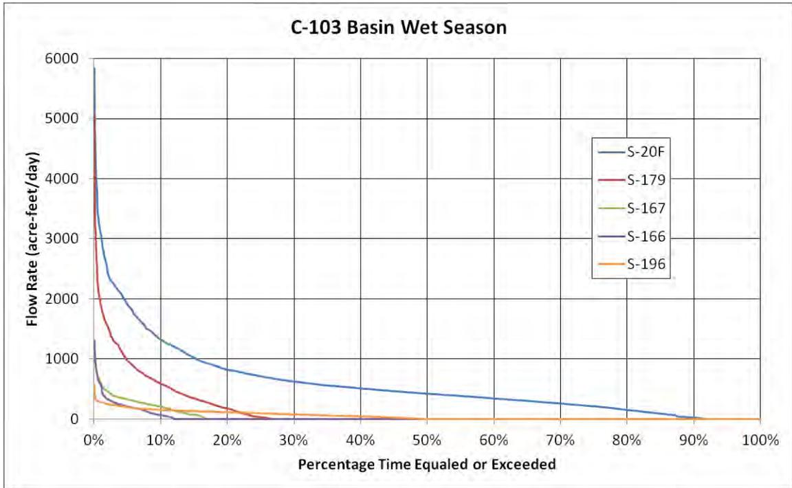
Figure C-22. Flow duration curves for the C-103 basin water control structures during the wet season.
