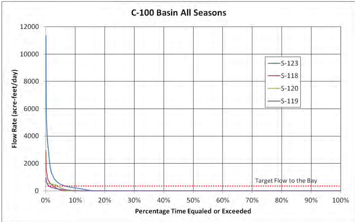
Figure C-1. Flow duration curves for the C-100 basin water control structures during all seasons.
