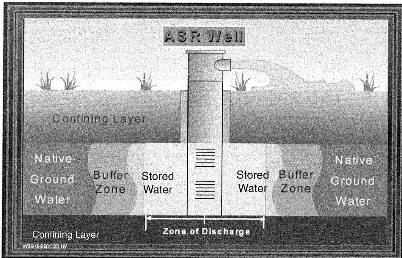
Figure 1 Zone of Discharge in an ASR Well
