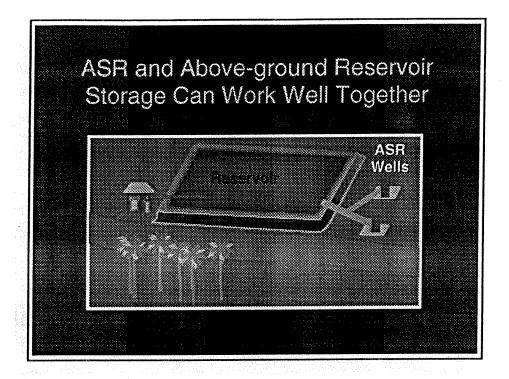
A combination of ASR wells and surface storage can increase the volume stored by allowing capture of high volume, high rate surface flows associated with storm events. This would increase water supply yield, improve recharge water quality, and reduce harm to the estuaries from peak flows.
