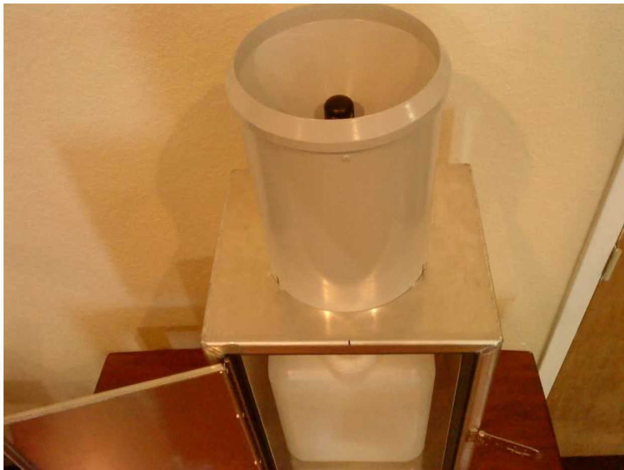
Figure 2.6-2. Top view of the tipping bucket rainfall gauge. The aperture is protected from debris by a screened cap.
