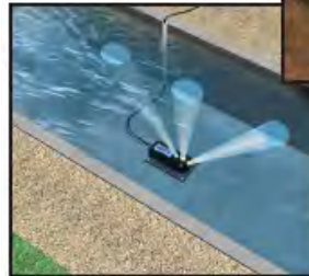
Example of an Argonaut-SW installed in an irrigation canal.
