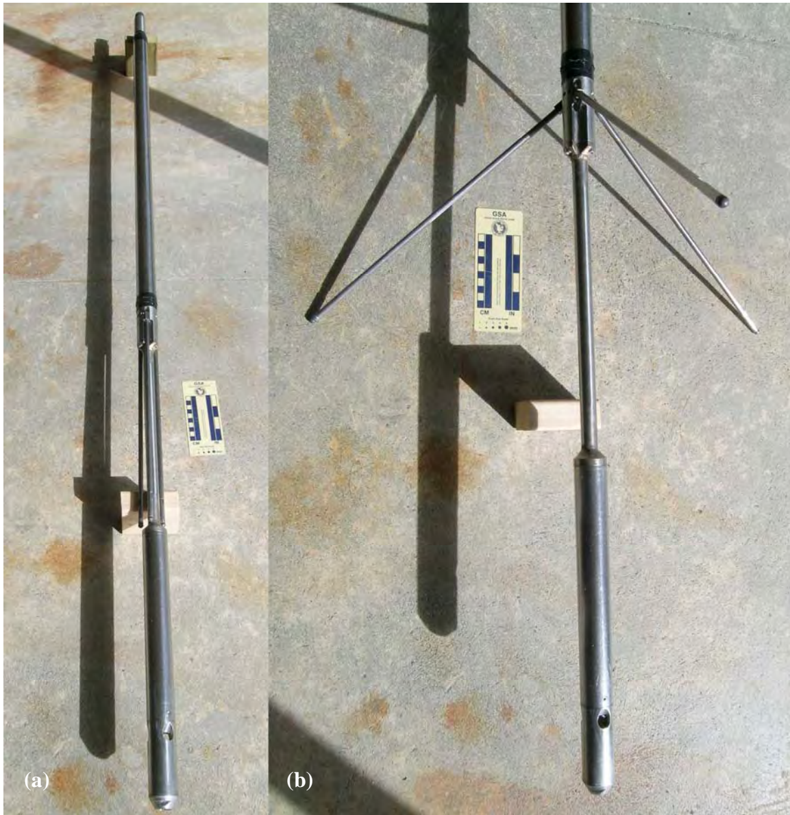
Figure 6. (a) Caliper and fluid temperature/resistivity tool with (b) detail of arms and fluid probe.
