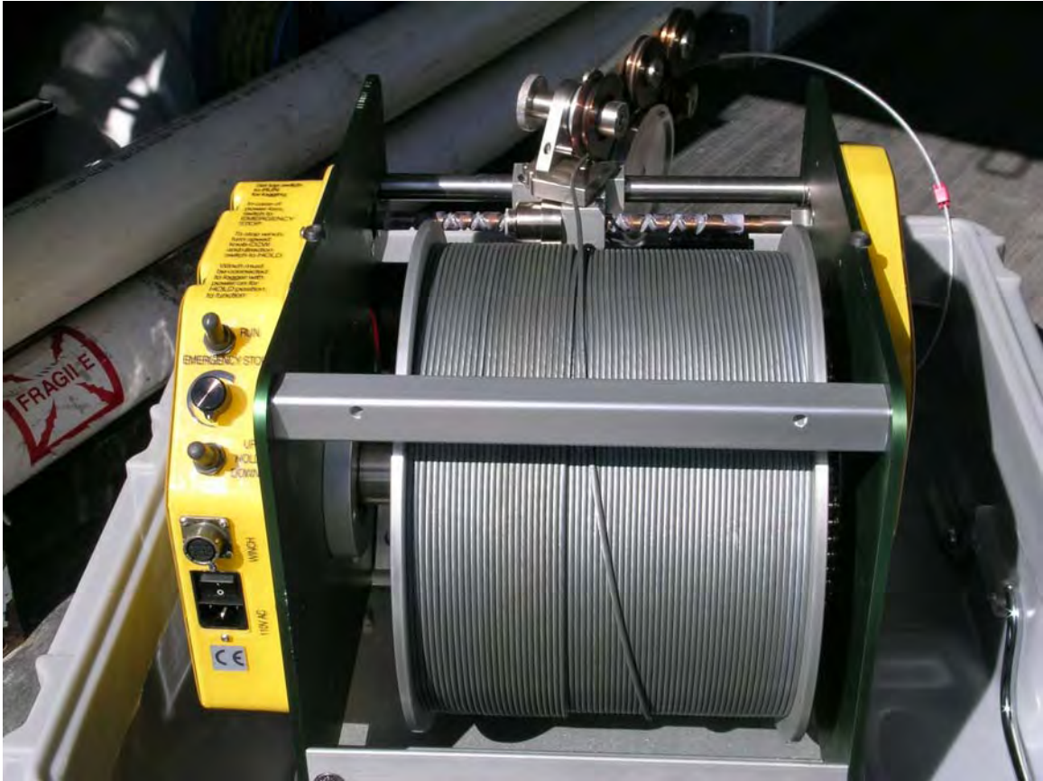
Figure 4. View of the large 4MCX1000 (3,280 feet of cable) winch.
