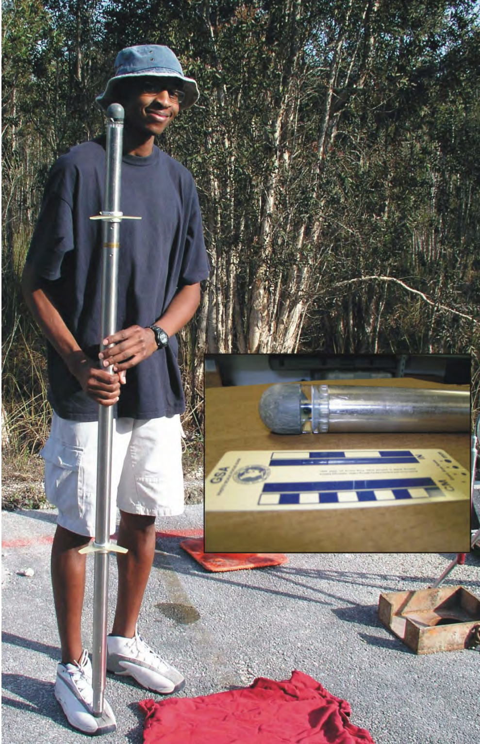
Figure 10. Student holding OBI-49 fitted with plastic rod-spring centralizers. Inset shows detail of optical head.
