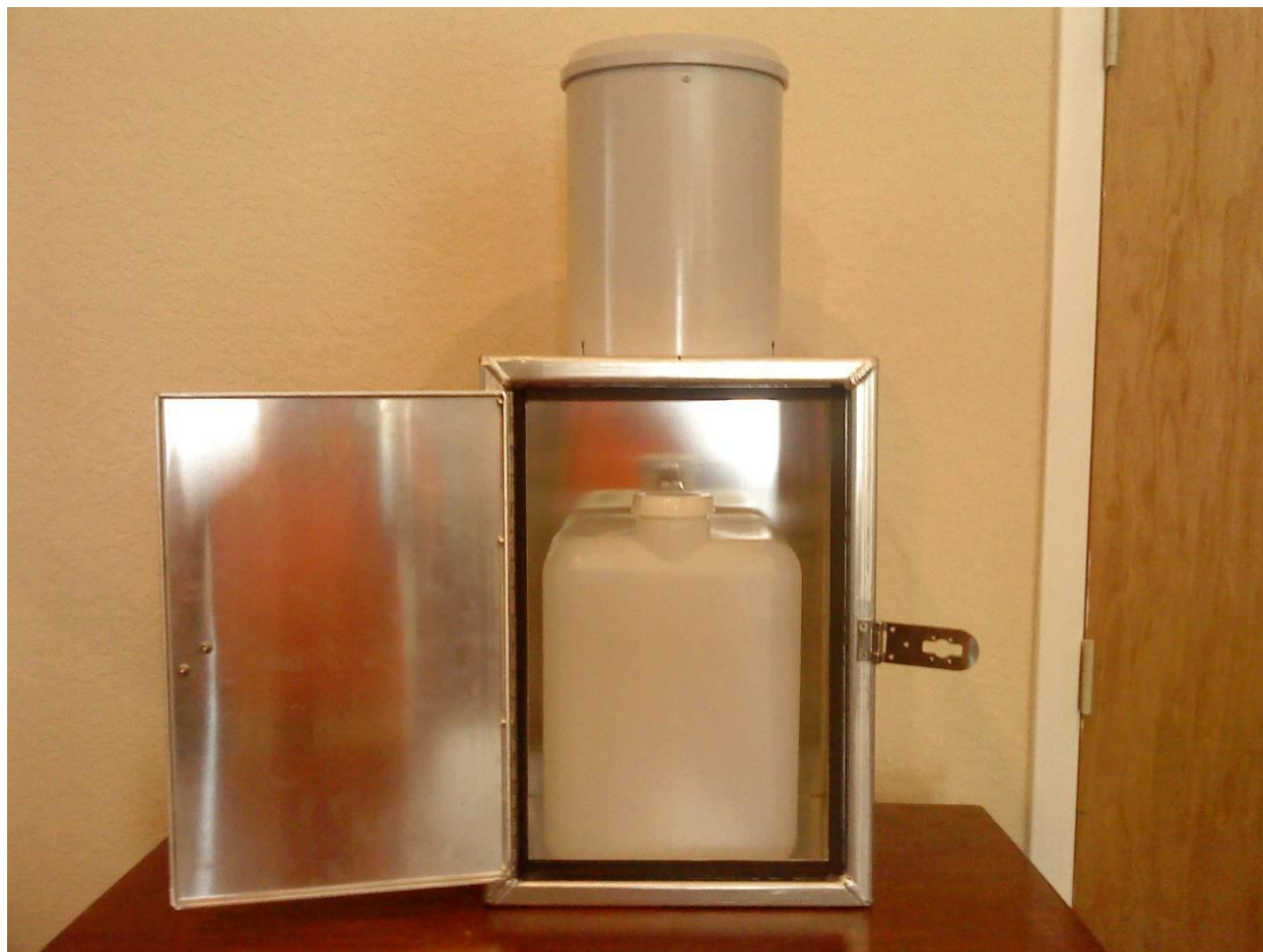
Figure 2.6-1. Integrated tipping bucket rain gauge with the rainfall collector located in a protective metal housing. The setup will also have a piece of polyethylene tubing connecting the rain gauge
