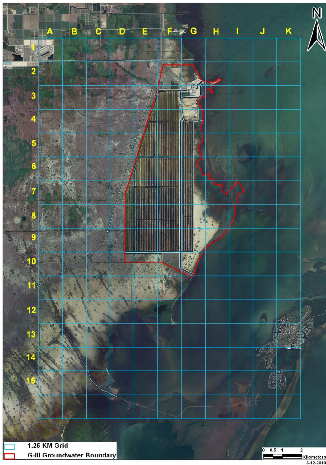
Figure 2.2-3. Grid Design for Porewater Surveys in Biscayne Bay and Card Sound
