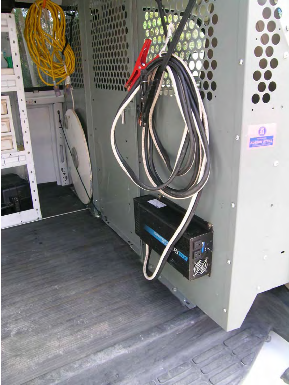
Figure 3. Wall mounted Excel Tech XP-1100 power inverter.
