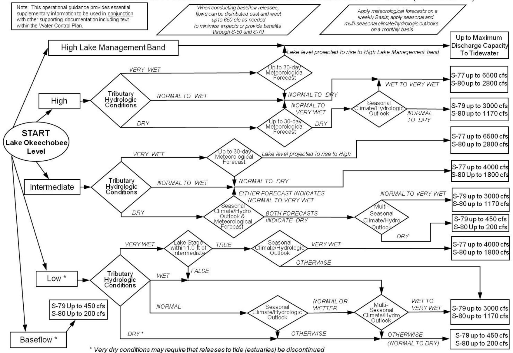
Figure 3. Guidance to establish allowable Lake Okeechobee releases to tide.
