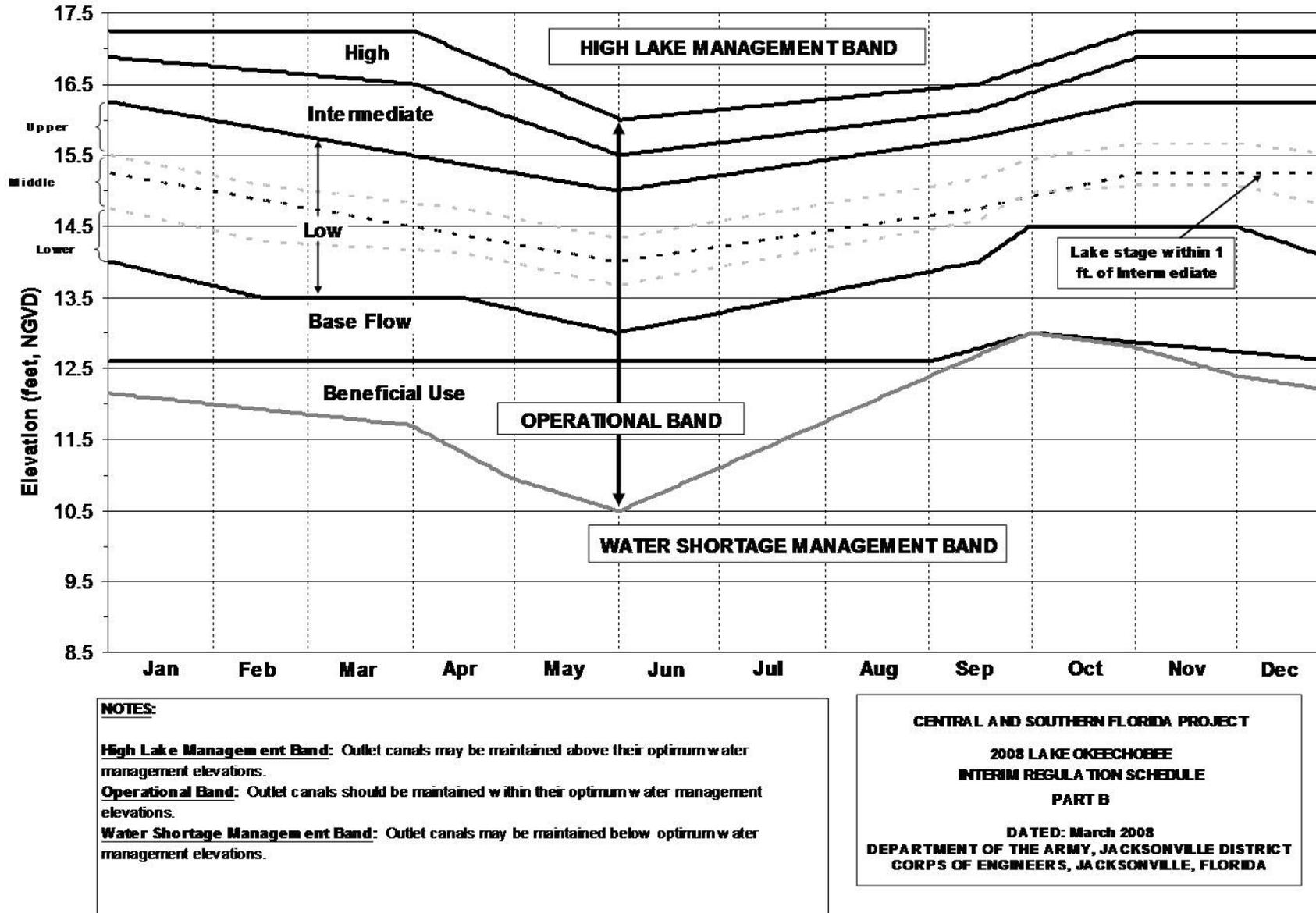
Figure 1. Bands and subbands for Lake Okeechobee developed for the 2008 LORS regulation schedule.
