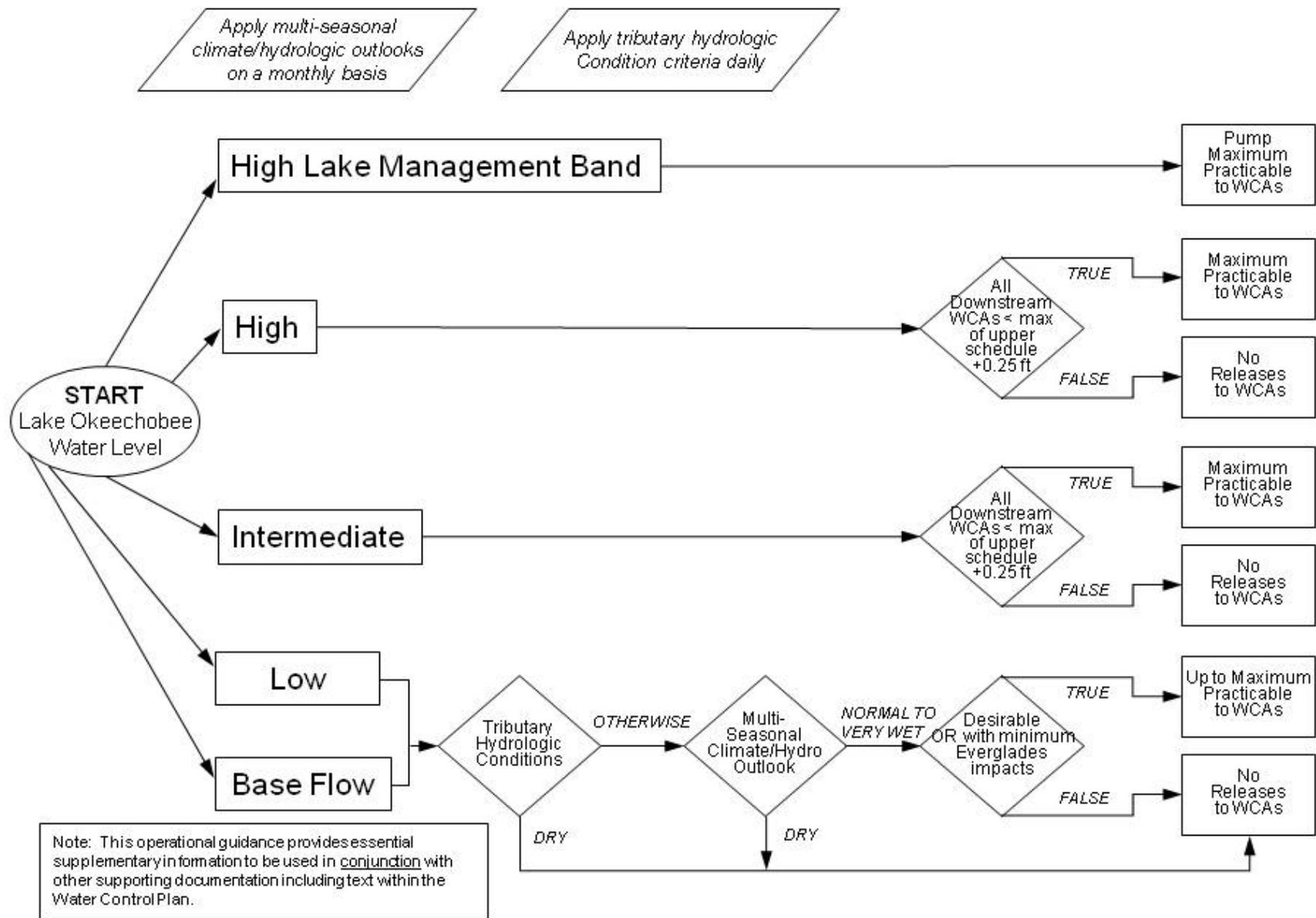
**Figure 2.** Guidance to establish allowable Lake Okeechobee releases to WCAs.
