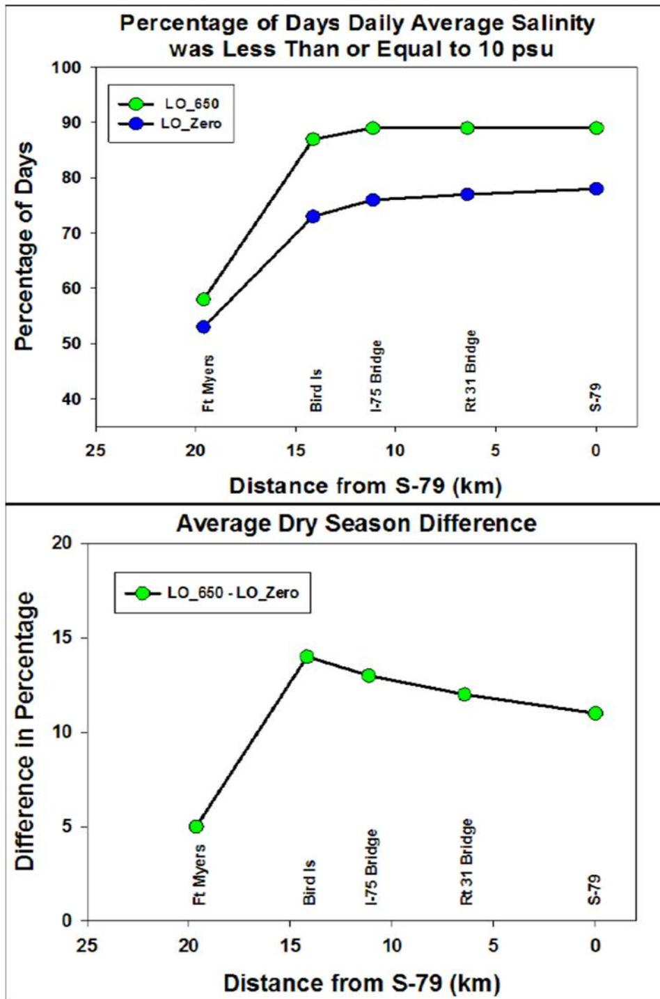
**Figure B-18.** Simulated salinity profile showing percentage of days average salinity was less than 10 psu during the dry season (upper figure) and difference (lower figure) as distance (in km) from S-79 decreases
