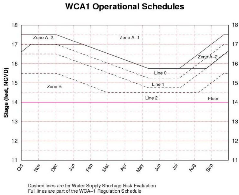
**Figure A-6.** WCA 1 lines for evaluation of water supply risk when using adaptive protocols for Lake Okeechobee operations
