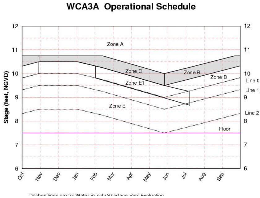
**Figure A-10.** WCA 3A lines for evaluation of water supply risk when using adaptive protocols for Lake Okeechobee operations
