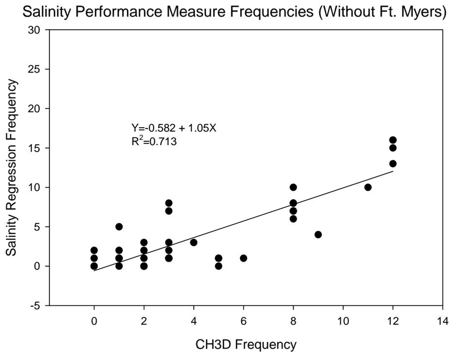
**Figure C-6.** Relationship between frequencies of duration classes calculated using the CH3D hydrodynamic model, and the salinity regressions from the LOOPS model with (top) and without (bottom) Fort Myers stations.
