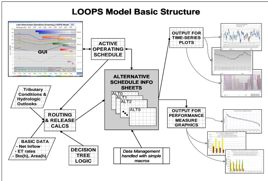
Figure 4. Basic Structure of the LOOPS Model
