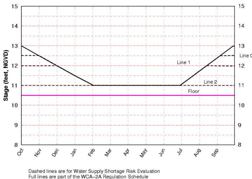
**Figure A-8.** WCA 2A lines for evaluation of water supply risk when using adaptive protocols for Lake Okeechobee operations
