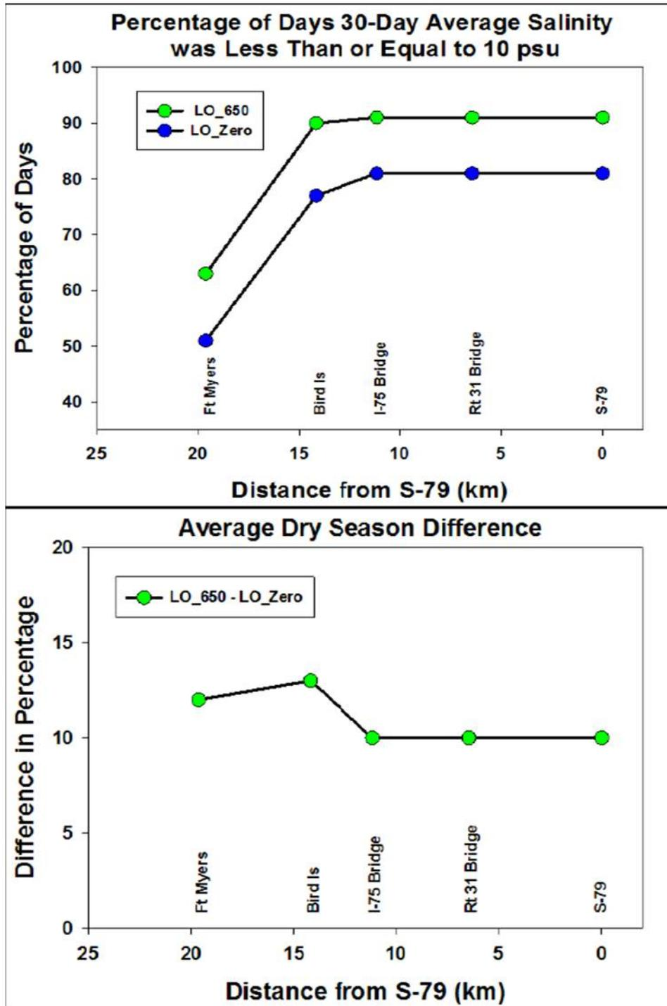
**Figure B-19.** Simulated salinity profile showing percentage of days 30-day moving average was less than 10 psu during the dry season (upper figure) and difference (lower figure) as distance (in km) from S-79 decreases
