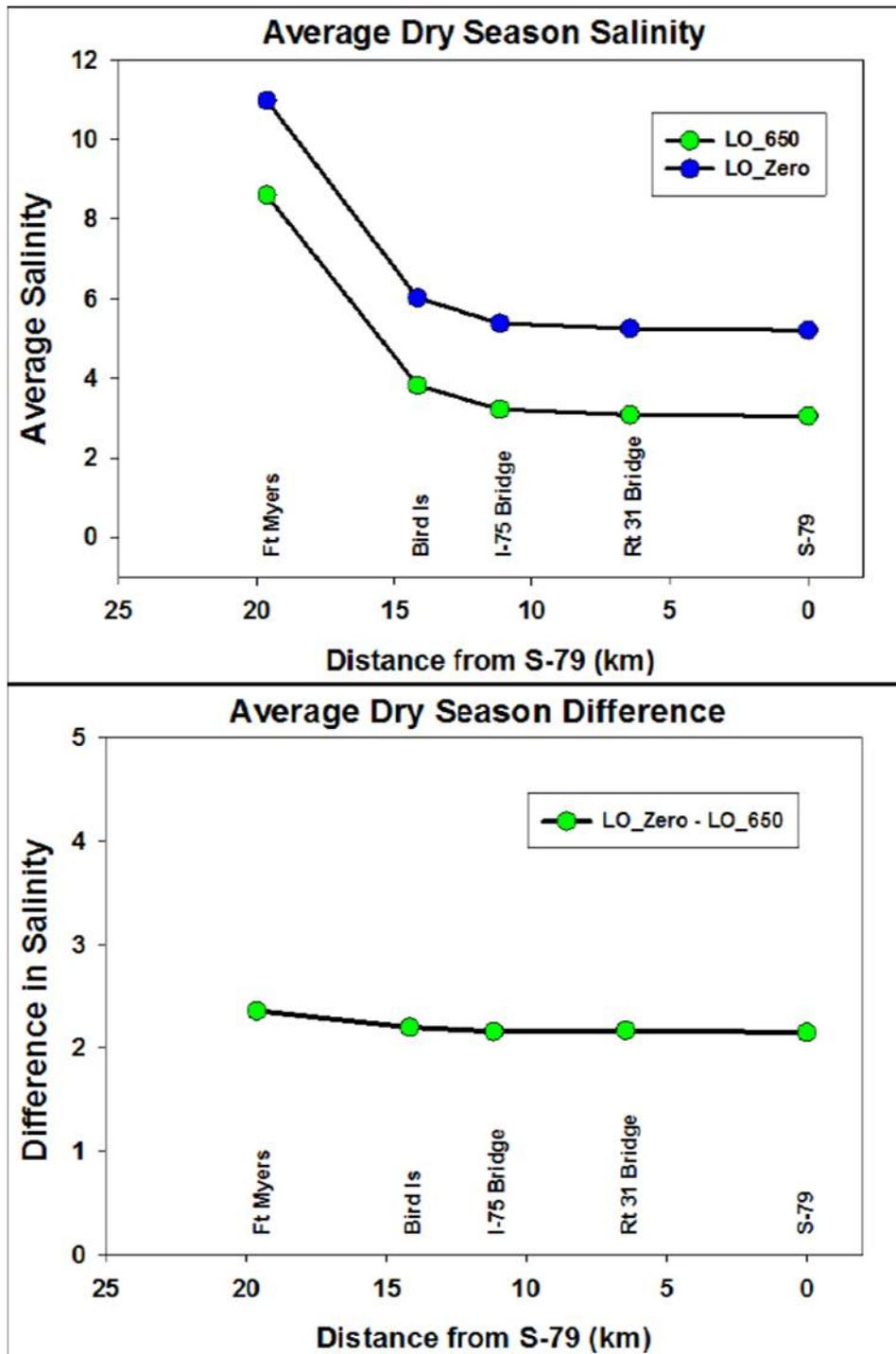
**Figure B-17.** Simulated salinity profile showing average dry season salinity (upper figure) and salinity difference (lower figure) as distance (in kilometers [km]) from S-79 decreases
