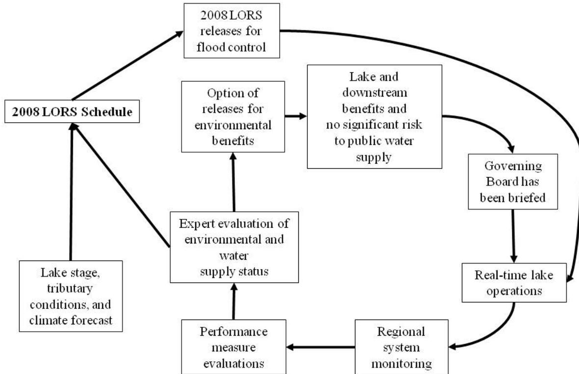
**Figure 6.** Feedback loop for real-time operations of Lake Okeechobee
