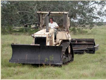
A roller-chopper used to remove small hardwoods from herbaceous understories
