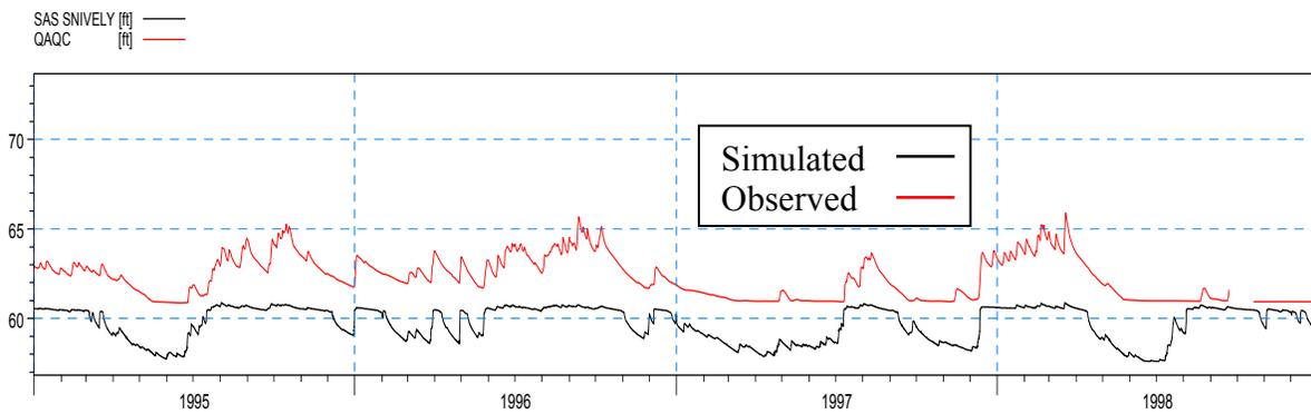
**Figure 4-54: Simulated and observed heads at SAS SNIVELY during the calibration period**
