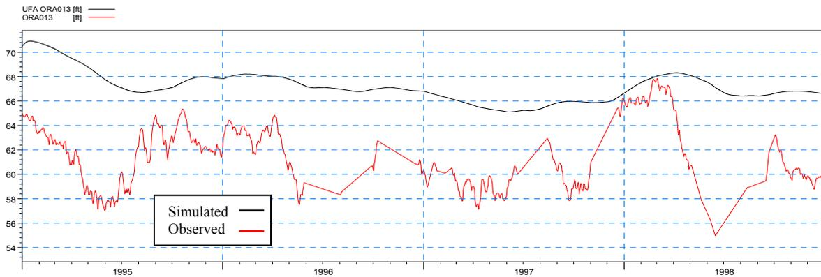
**Figure 4-74: Simulated and observed heads at UFA ORA 013 during the calibration period**
