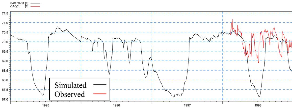
**Figure 4-49: Simulated and observed heads at SAS CAST during the calibration period**
