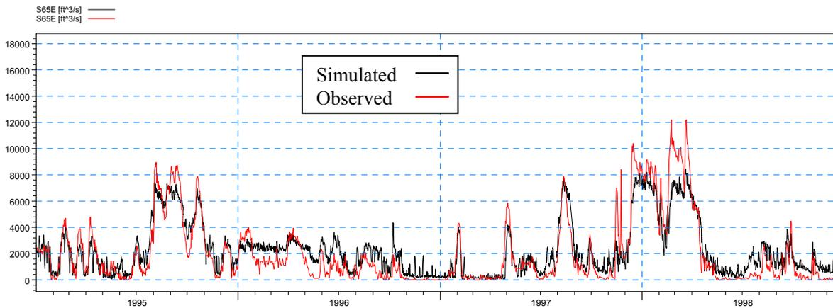
**Figure 4-44: Simulated and observed discharge at S-65E during the calibration period**
