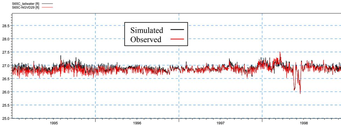
**Figure 4-35: Simulated and observed tailwater stage at S-65C during the calibration period**
