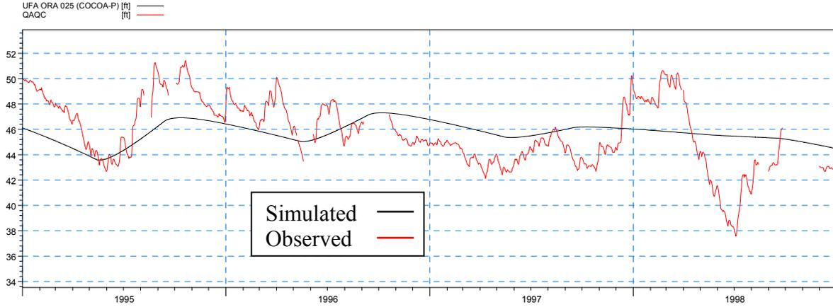
**Figure 4-75: Simulated and observed heads at UFA ORA 025/Cocoa-P during the calibration period**
