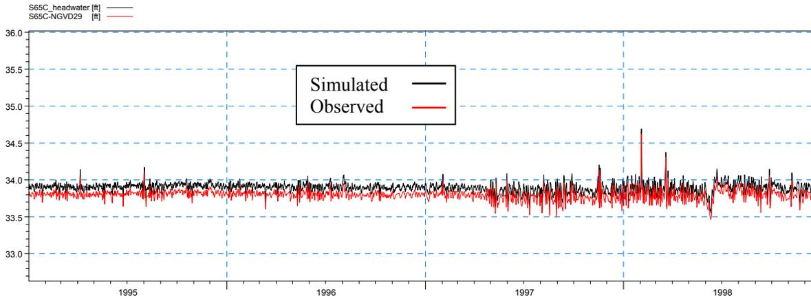
**Figure 4-34: Simulated and observed headwater stage at S-65C during the calibration period**
