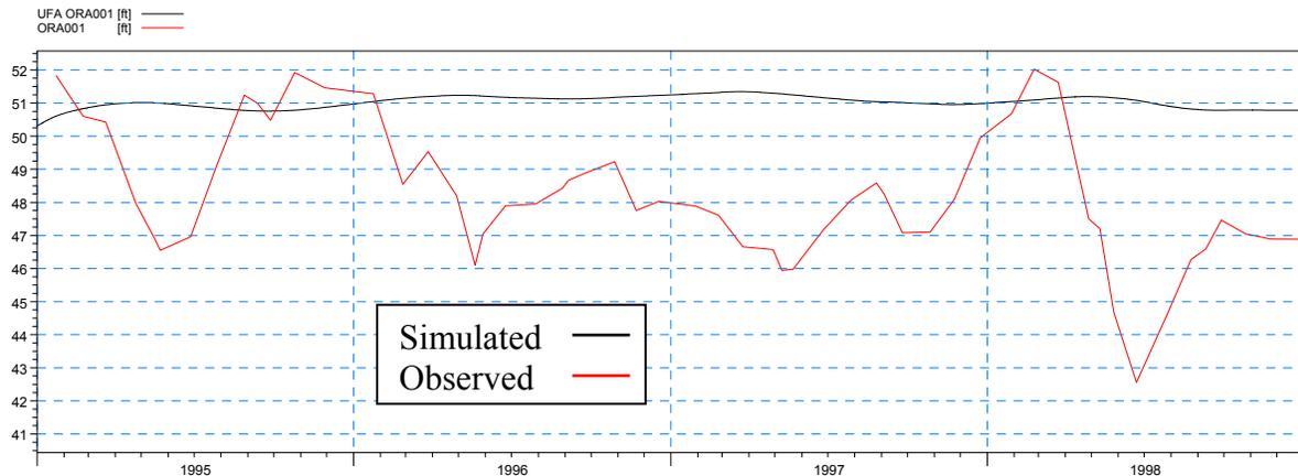
**Figure 4-68: Simulated and observed heads at UFA ORA 001 during the calibration period**
