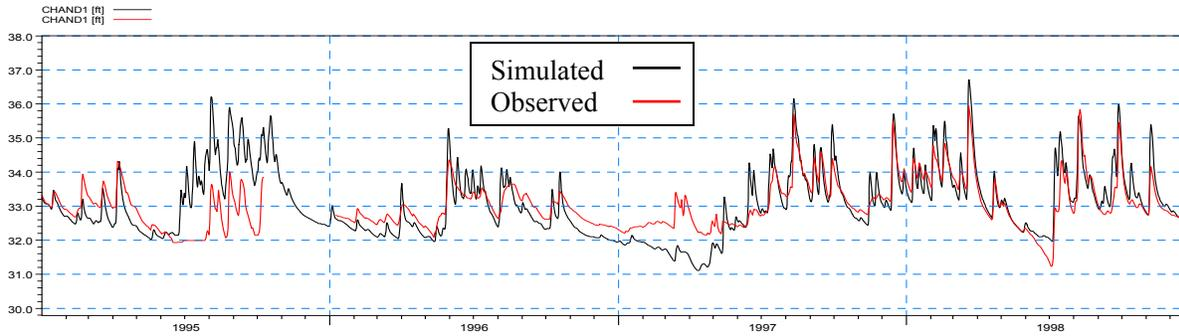
**Figure 4-43: Simulated and observed stage at CHAND1 during the calibration period**
