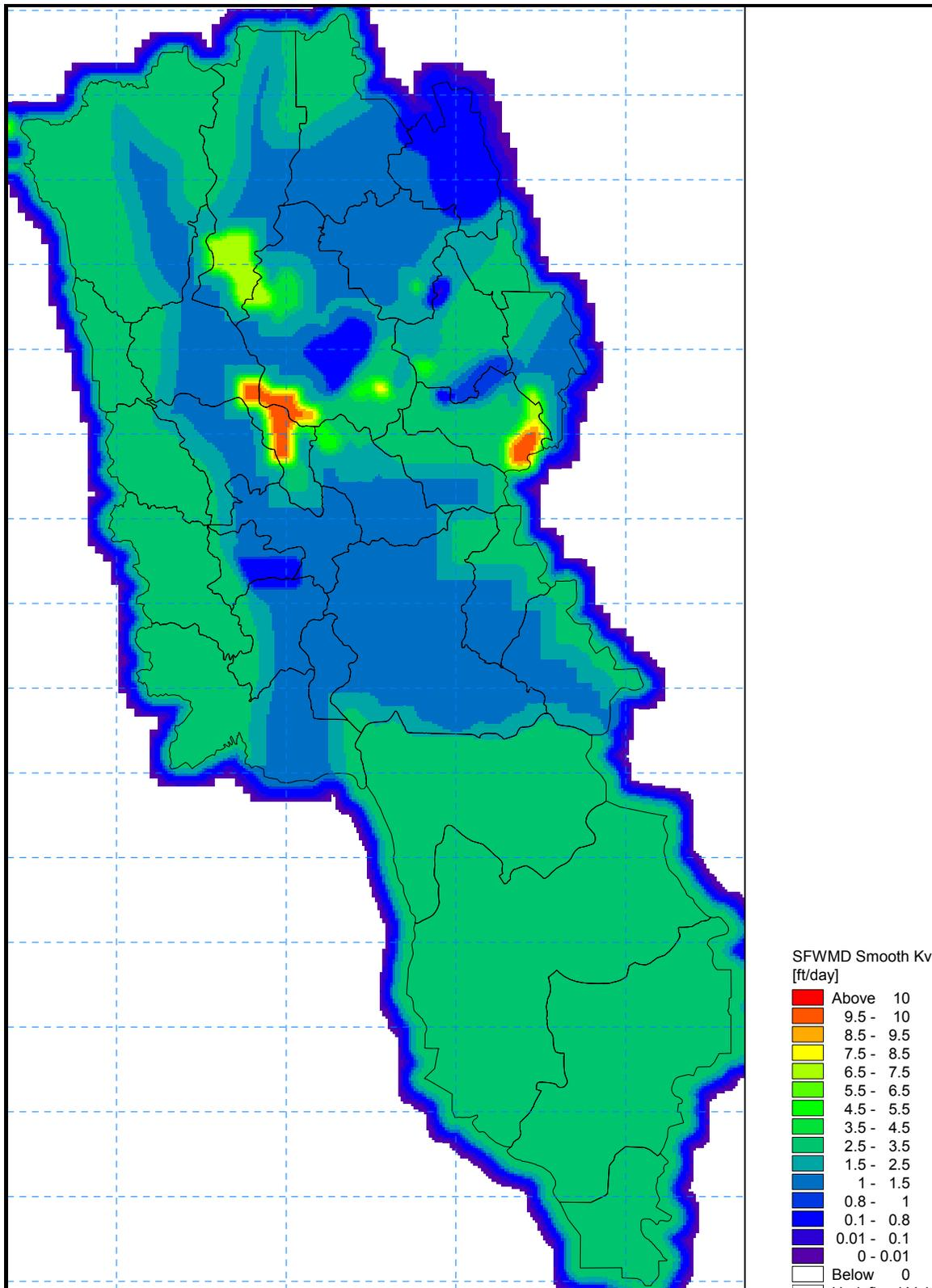
Figure 2-8: AFET-W Vertical Hydraulic Conductivity of the Surficial Aquifer
