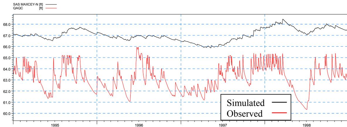
**Figure 4-63: Simulated and observed heads at SAS MAXCEY-N during the calibration period**
