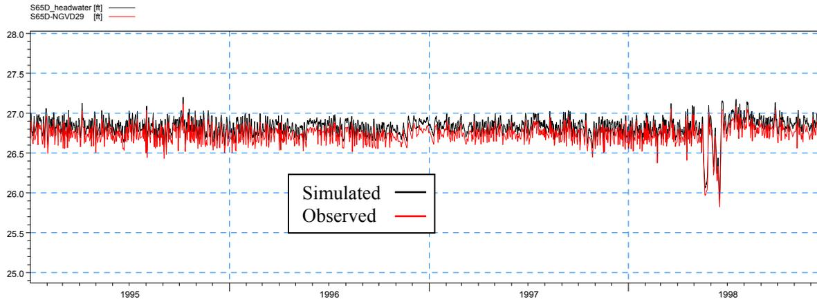
**Figure 4-37: Simulated and observed headwater stage at S-65D during the calibration period**
