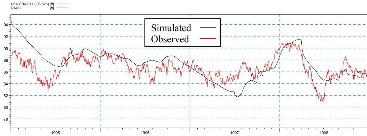
**Figure 4-70: Simulated and observed heads at UFA ORA 017/GS 825 during the calibration period**
