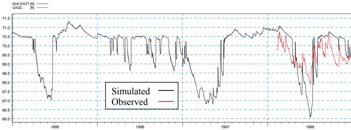
**Figure 4-50: Simulated and observed heads at SAS EXOT during the calibration period**
