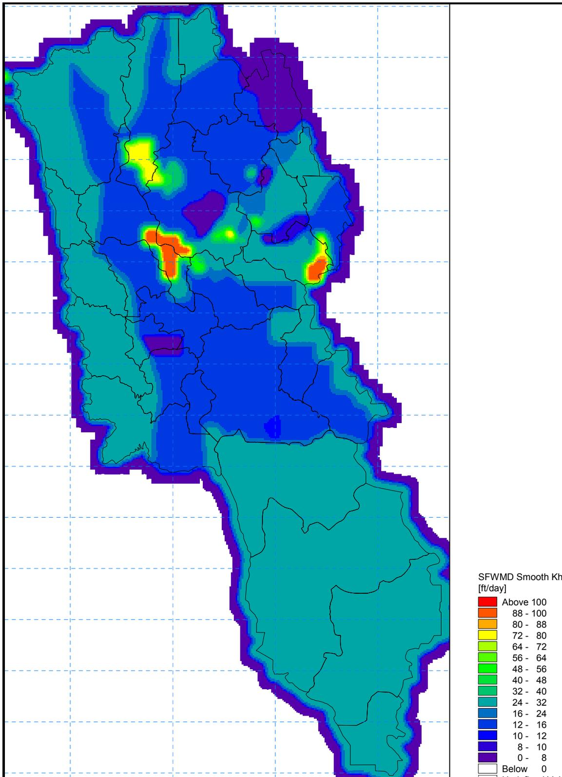
Figure 2-7: AFET-W Horizontal Hydraulic Conductivity of the Surficial Aquifer
