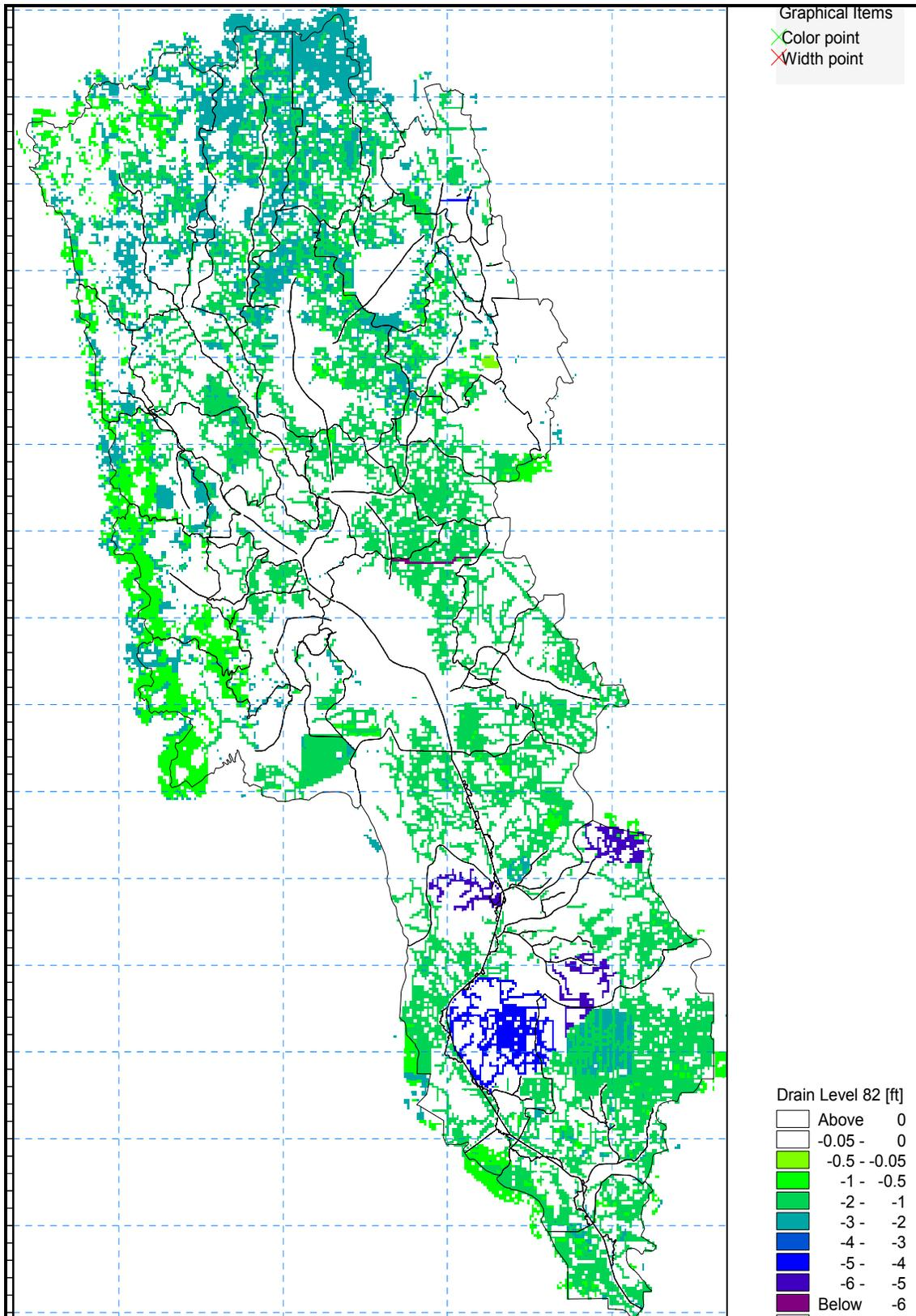
Figure 2-13: AFET-W Drain Levels (negative indicates ft below land surface)
