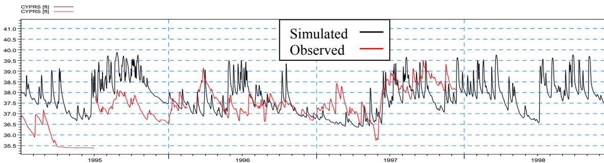
**Figure 4-42: Simulated and observed stage at CYPRS during the calibration period**
