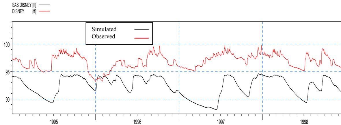
**Figure 4-60: Simulated and observed heads at SAS DISNEY during the calibration period**
