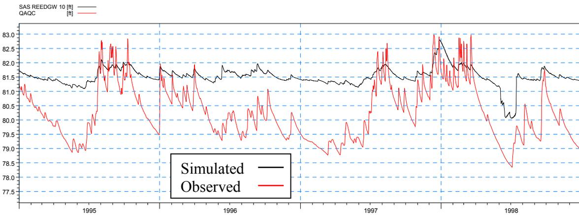
**Figure 4-47: Simulated and observed heads at SAS REEDGW 10 during the calibration period**
