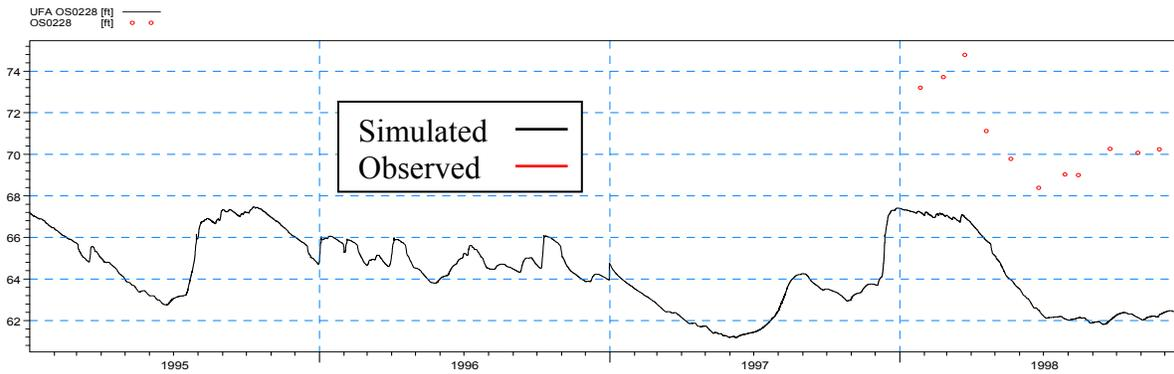
**Figure 4-56: Simulated and observed heads at SAS OSO228 during the calibration period**
