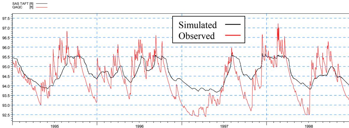
**Figure 4-45: Simulated and observed heads at SAS TAFT during the calibration period**
