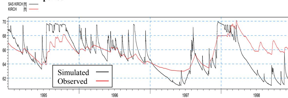
**Figure 4-51: Simulated and observed heads at SAS KIRCH during the calibration period**
