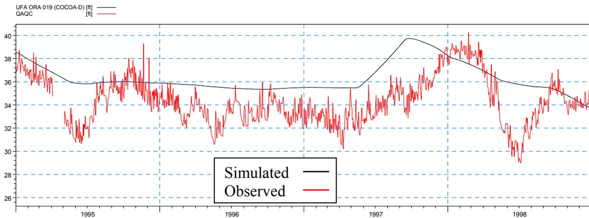
**Figure 4-77: Simulated and observed heads at UFA ORA 019 (COCOA-D) during the calibration period**
