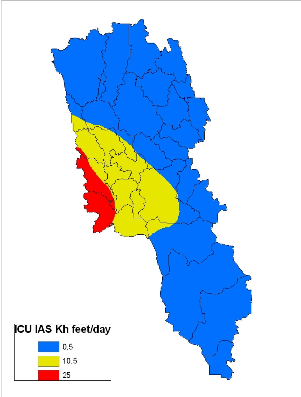
**Figure 2-9: AFET-W Horizontal Hydraulic Conductivity of the Intermediate Aquifer System**
