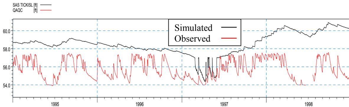
**Figure 4-62: Simulated and observed heads at SAS TICKISL during the calibration period**
