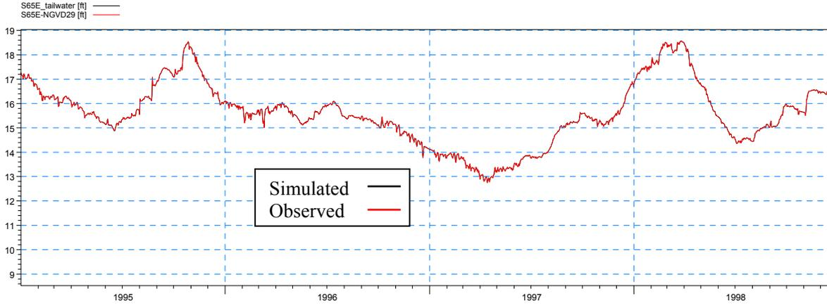
**Figure 4-40: Simulated and observed headwater stage at S-65E during the calibration period**
