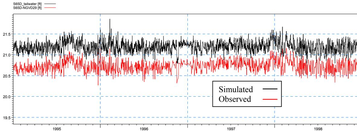
**Figure 4-38: Simulated and observed tailwater stage at S-65D during the calibration period**
