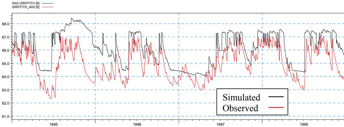
**Figure 4-67: Simulated and observed heads at SAS GRIFFITH during the calibration period**
