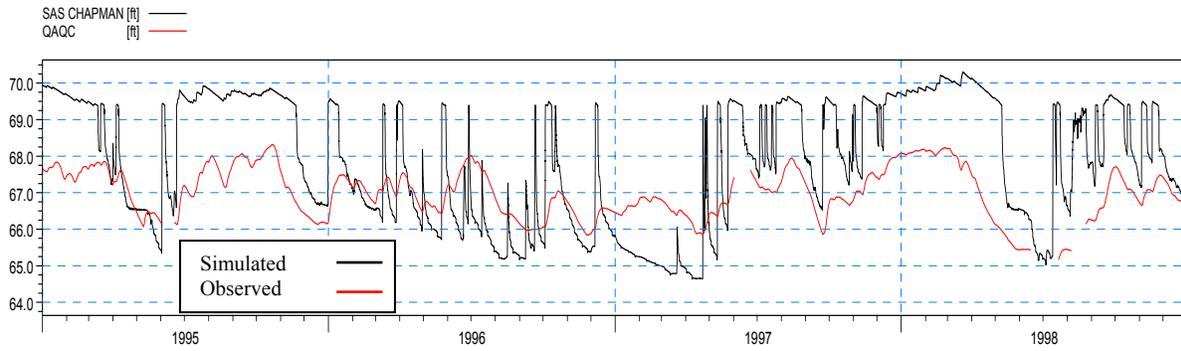
**Figure 4-58: Simulated and observed heads at SAS CHAPMAN during the calibration period**
