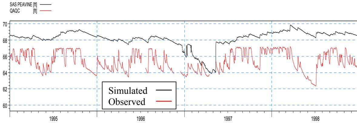
**Figure 4-64: Simulated and observed heads at SAS PEAVINE during the calibration period**
