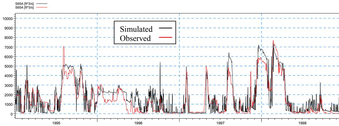
**Figure 4-32: Simulated and observed discharge at S-65A during the calibration period**
