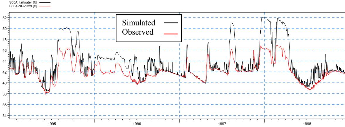
**Figure 4-31: Simulated and observed tailwater stage at S-65A during the calibration period**
