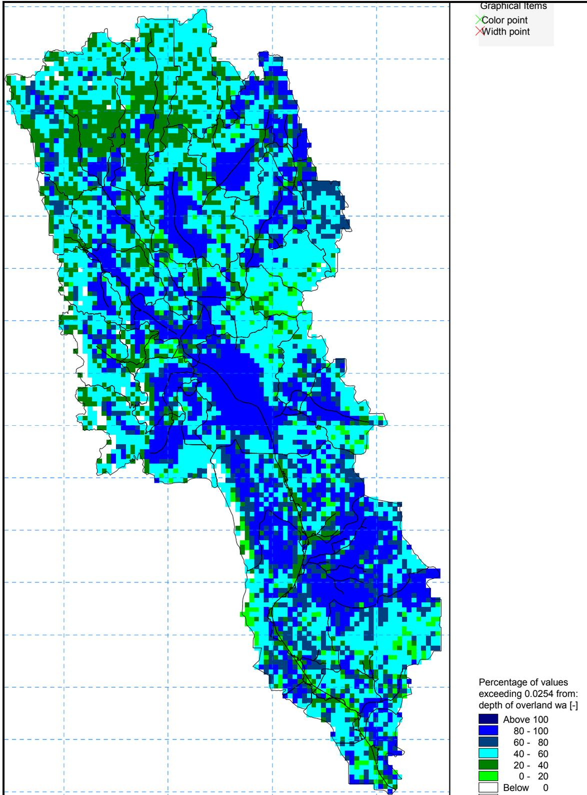
Figure 4-89: Percentage of time overland flow depths exceed 1 inch during the period from 1996 to 1997
