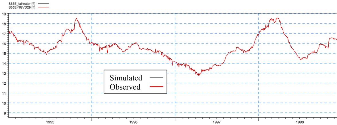
**Figure 4-41: Simulated and observed tailwater stage at S-65E during the calibration period**
