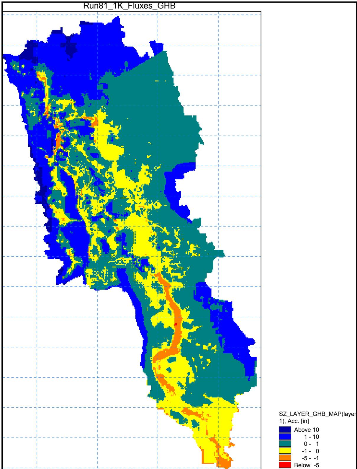
Figure 4-80: Simulated Upper Floridan Aquifer recharge rates from the 1,000 ft surficial aquifer model
