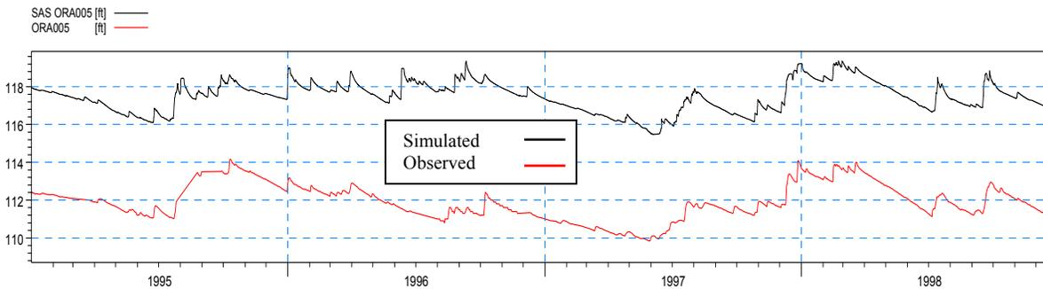
**Figure 4-57: Simulated and observed heads at SAS ORA005 during the calibration period**
