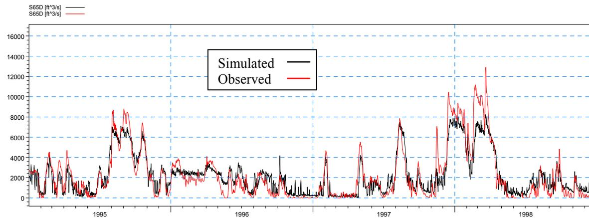
**Figure 4-39: Simulated and observed discharge at S-65D during the calibration period**
