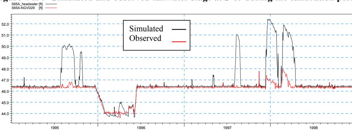
**Figure 4-30: Simulated and observed headwater stage at S-65A during the calibration period**
