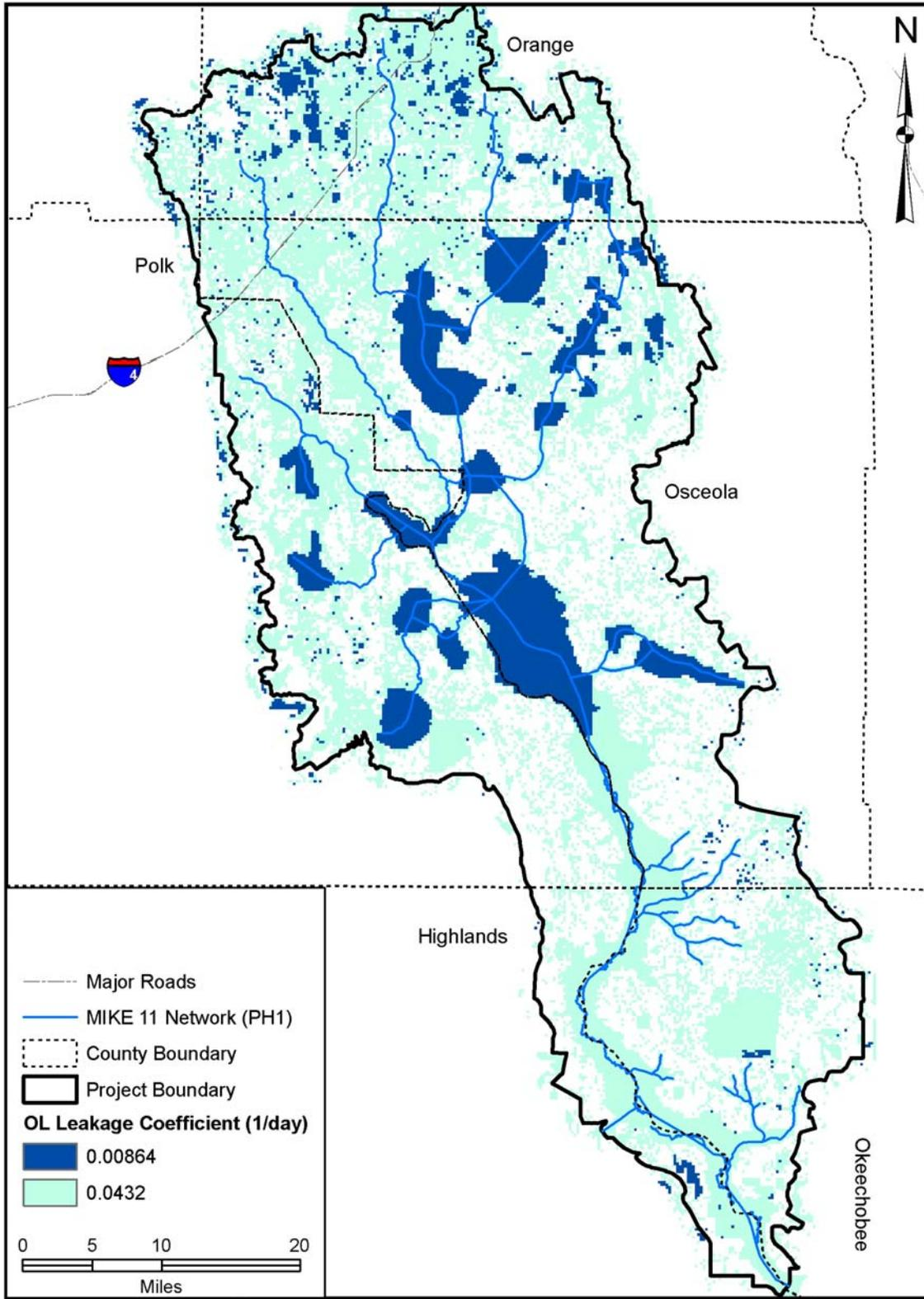
Figure 2-4: AFET and AFET-W Overland – Saturated Zone Leakage Coefficients (day<sup>-1</sup>)
