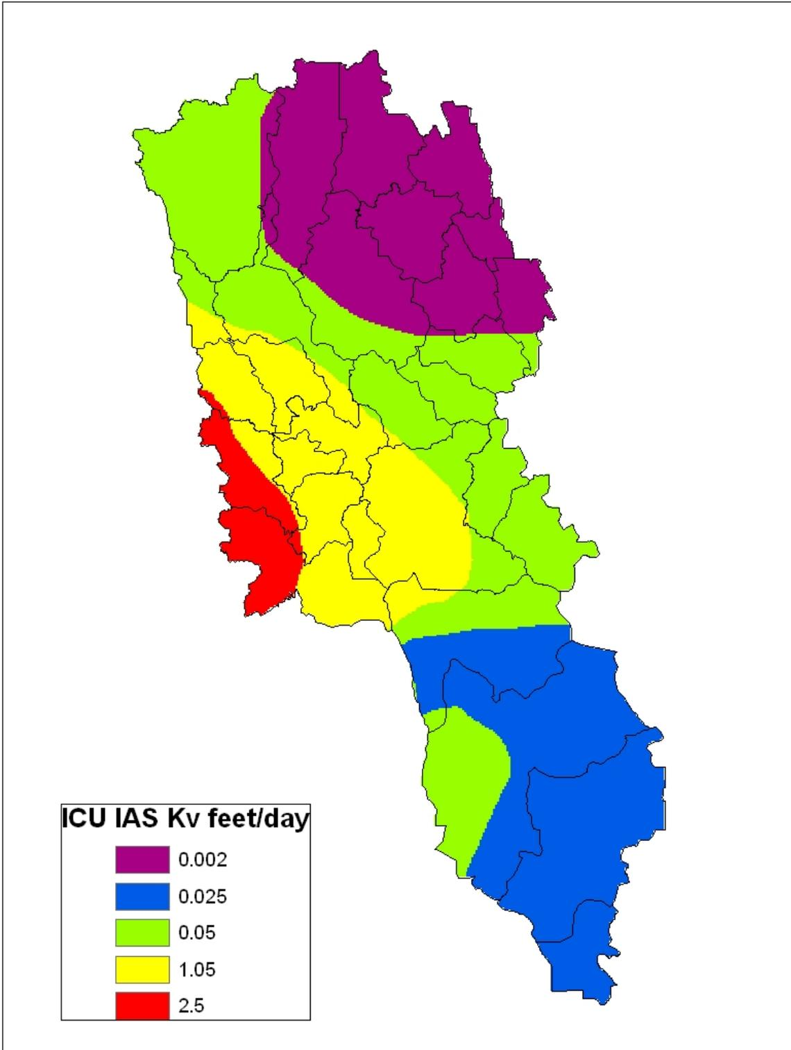
Figure 2-10: AFET-W Vertical Hydraulic Conductivity of the Intermediate Confining Unit
