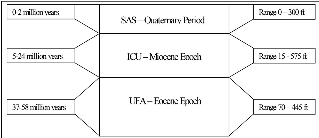
**Figure 2-6: Conceptual Geological Model**
