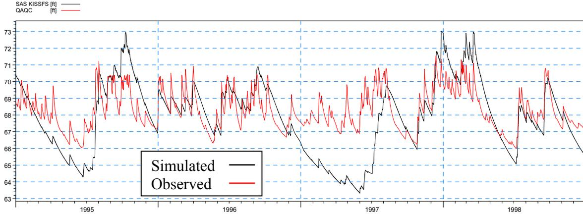
**Figure 4-46: Simulated and observed heads at KISSFS during the calibration period**
