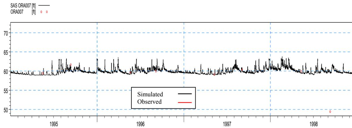
**Figure 4-59: Simulated and observed heads at SAS ORA007 during the calibration period**
