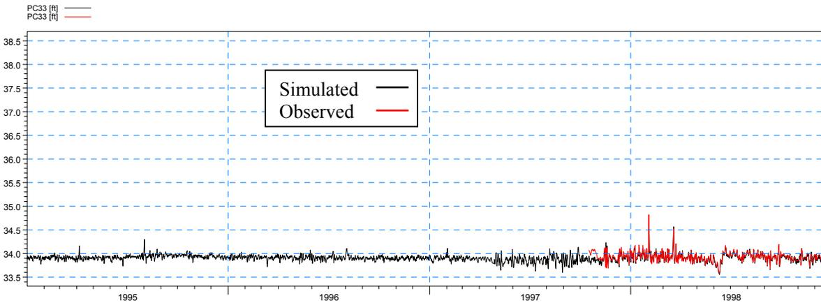
**Figure 4-33: Simulated and observed stage at PC33 during the calibration period**
