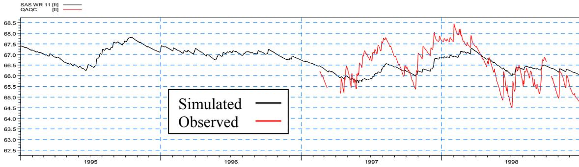
**Figure 4-55: Simulated and observed heads at SAS WR 11 during the calibration period**
