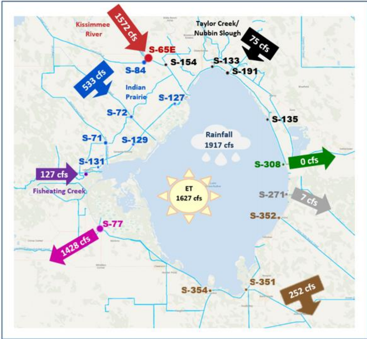
Figure LO-5. Inflows into Lake Okeechobee from Indian Prairie basins, Taylor Creek/Nubbin Slough, Kissimmee River and Fisheating Creek, and outflows to the west via S-77, to the east via S-308, to the south via S-351, S-352, S-354, and to southeast via S-271 (formerly Culvert 10A) for the week of December 12 – December 18, 2022.
