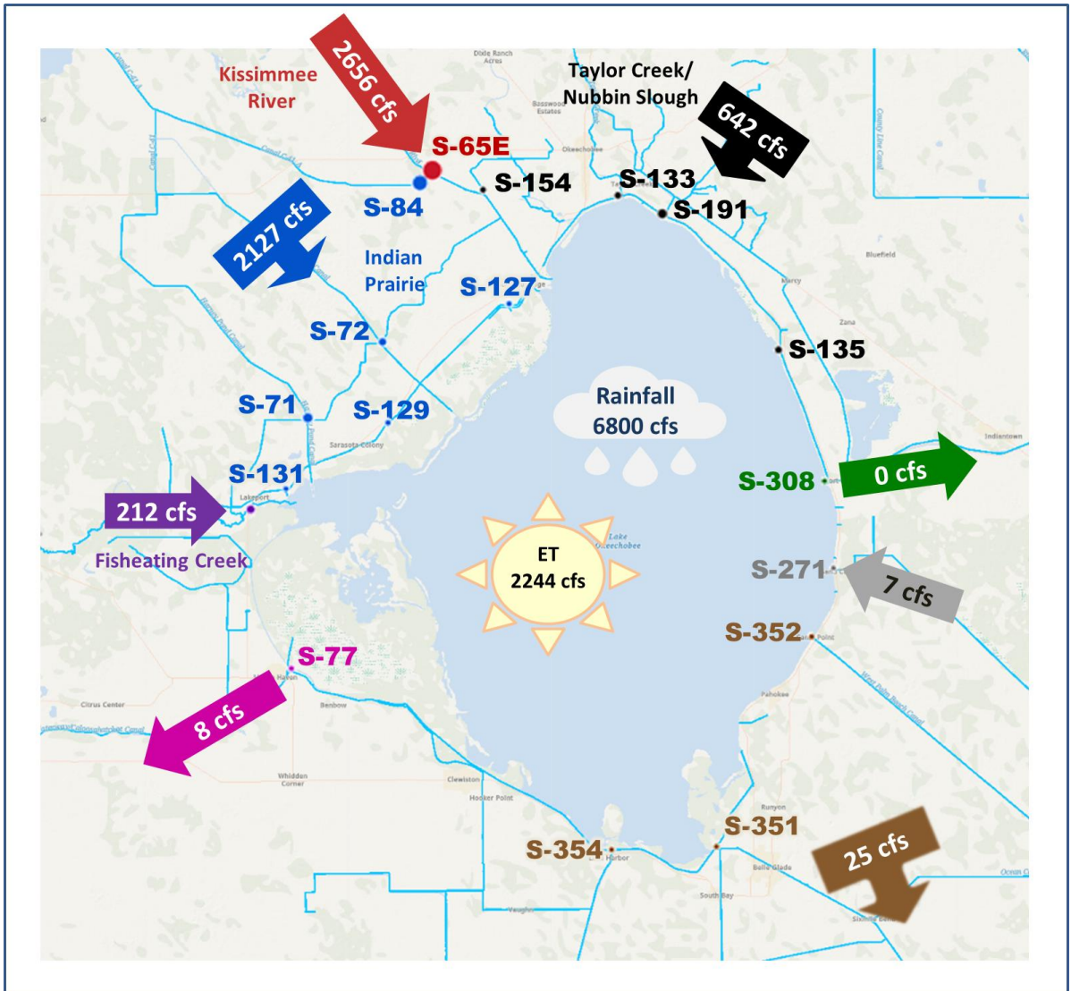
Figure LO-5. Inflows into Lake Okeechobee from Indian Prairie basins, Taylor Creek/Nubbin Slough, Kissimmee River and Fisheating Creek, and outflows to the west via S-77, to the east via S-308, to the south via S-351, S-352, S-354, and to southeast via S-271 (formerly Culvert 10A) for the week of November 7 - 13, 2022.
