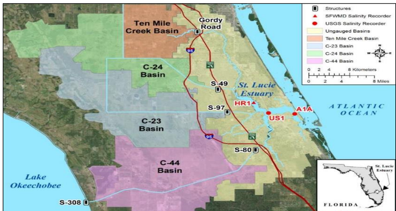
Figure ES-1. Basins, water control structures and salinity monitoring sites in the St. Lucie Estuary.
