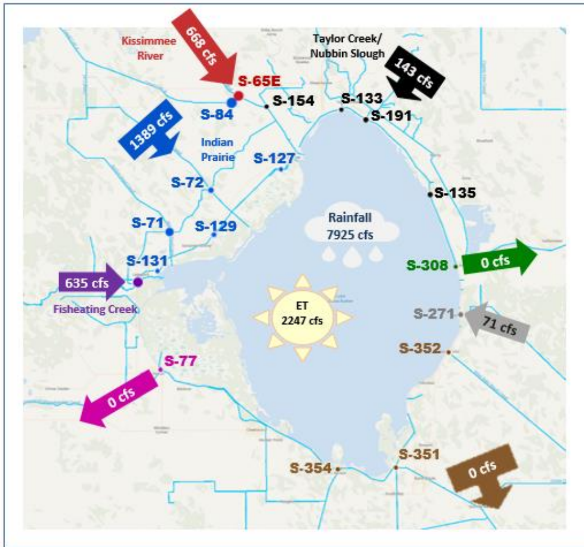
Figure LO-5. Inflows into Lake Okeechobee from Indian Prairie basins, Taylor Creek/Nubbin Slough, Kissimmee River and Fisheating Creek, and outflows to the west via S-77, to the east via S-308, to the south via S-351, S-352, S-354, and to southeast via S-271 (formerly Culvert 10A) for the week of September 12-18, 2022.
