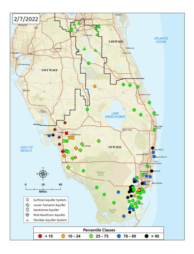
Figure 1. Real-Time Groundwater Level Map
