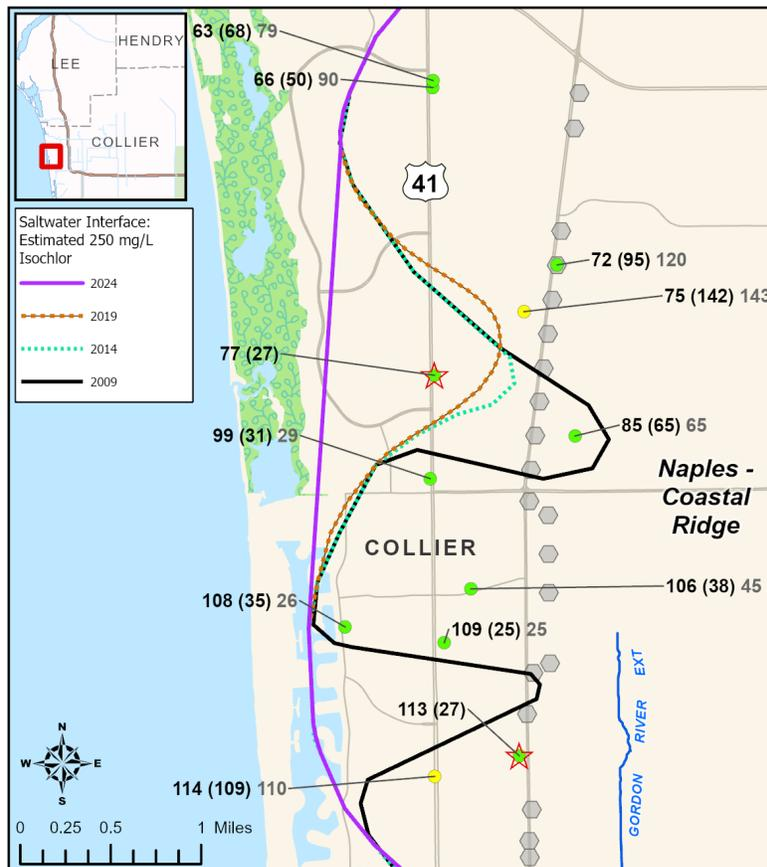
Figure 50. Position of the 2024 saltwater interface in the LTA in the City of Naples area in Collier County, primarily due to newly obtained data.
