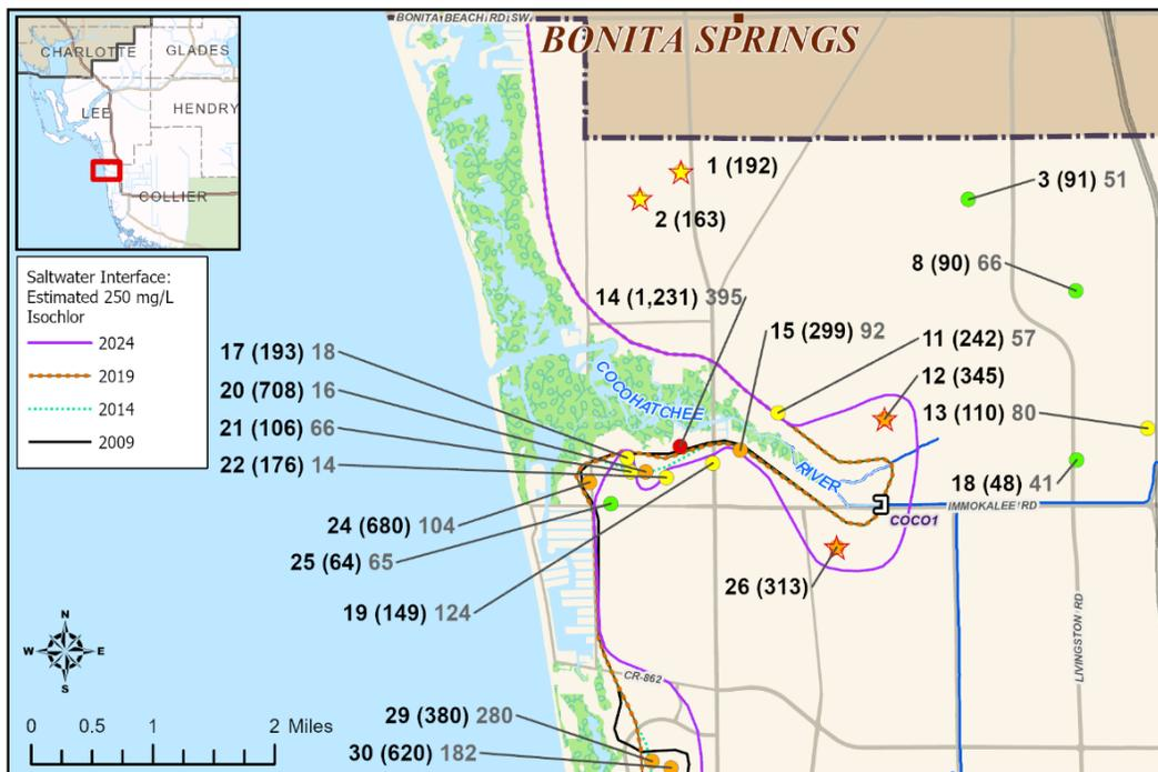
Figure 45. Position of the 2024 saltwater interface in the WTA near the Cocohatchee River in Collier County.
