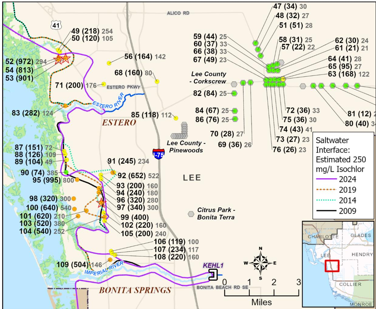
Figure 43. Position of the 2024 saltwater interface in the WTA in coastal Lee County.
