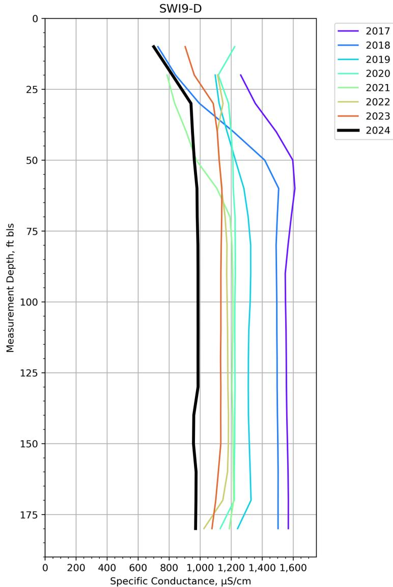
Figure 33. Fluid specific conductance versus depth plot for SWI9-D ID 136332 (Map ID 45), located at the southeastern edge of the 2024 interface in **Figure 31** in the City of Pompano Beach in Broward County.
