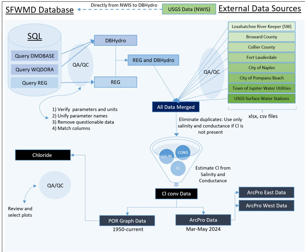
Figure 3. The data gathering and evaluation process for the saltwater intrusion evaluation conducted by the SFWMD.
