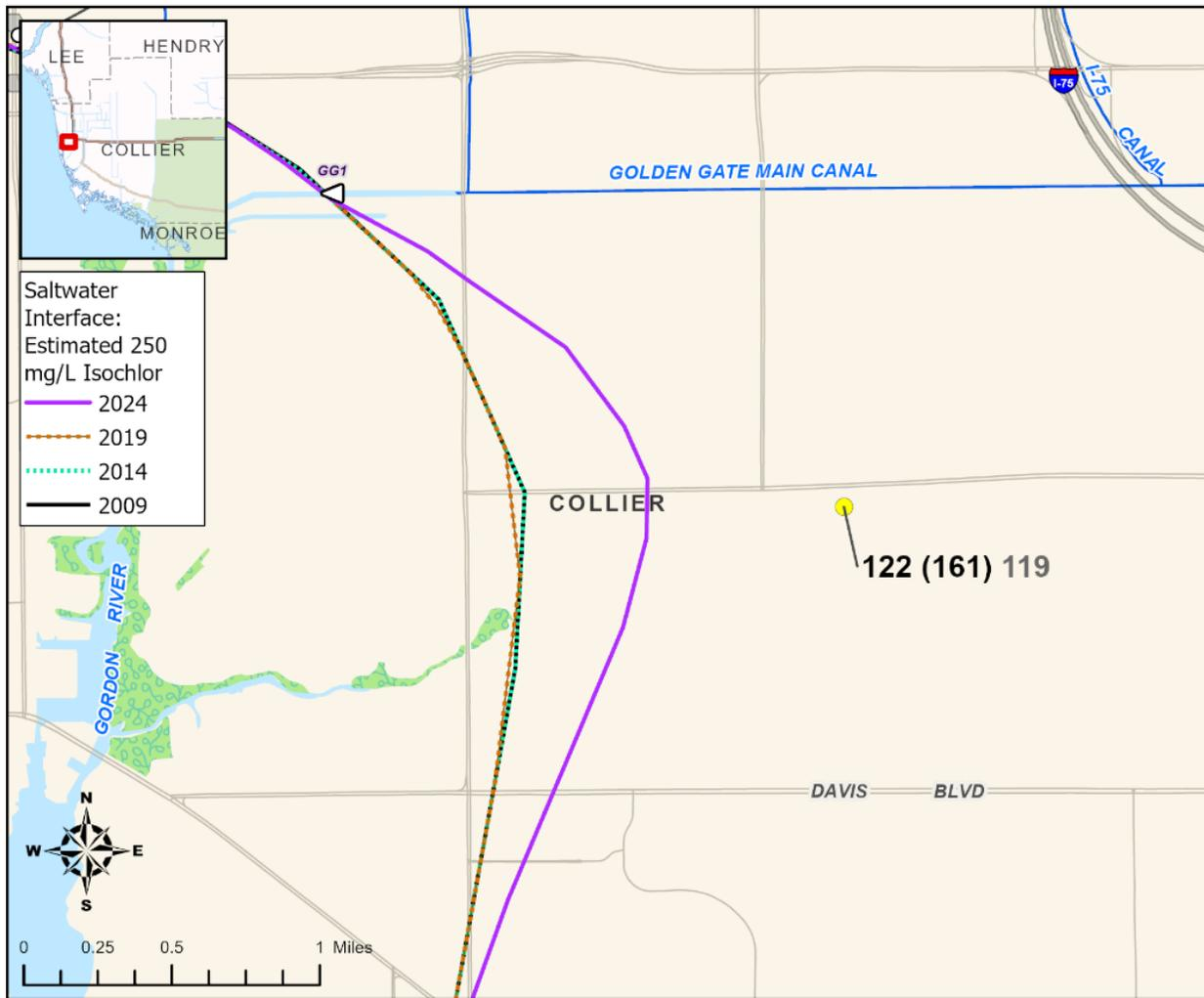
Figure 51. Position of the 2024 saltwater interface in the LTA east of the City of Naples and the Gordon River in Collier County, due to increasing chloride concentrations at C3 ID 2997 Map ID 122.
