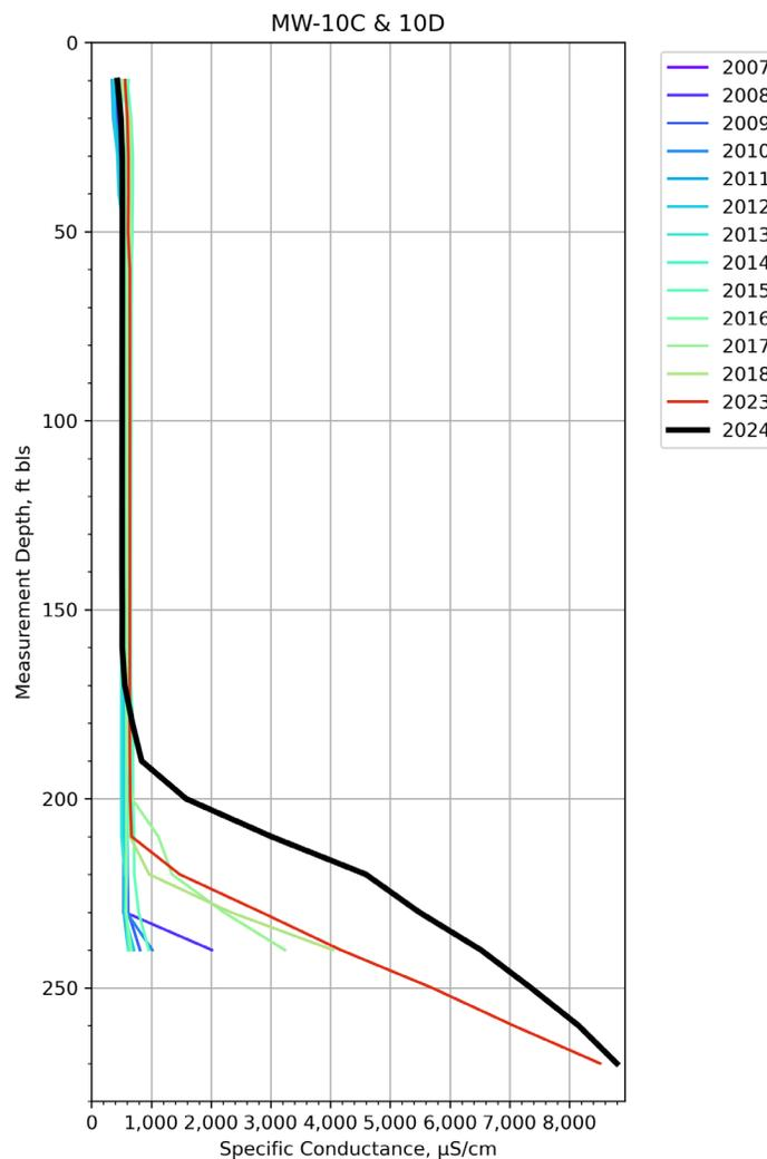
Figure 37. Fluid specific conductance plot for City of Fort Lauderdale monitor wells MW10C and MW10D ID 286505 near the Dixie PS wellfield in Broward County.
