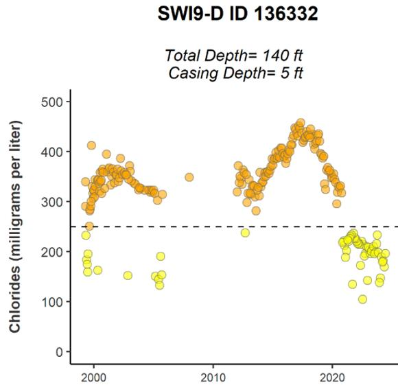
Figure 32. Chloride time-series plot for SWI9-D ID 136332, located at the southeastern edge of the 2024 interface in Figure 31 (Map ID 45) in the City of Pompano Beach in Broward County.
