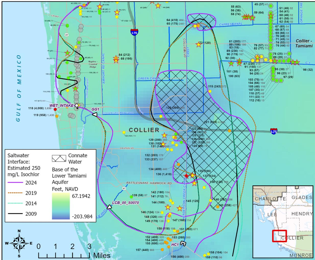
Figure 53. Connate water areas in the LTA, wells with 2024 chloride concentrations, and approximate elevation of the base of the LTA in Collier County (Zumbro et al. 2023).
