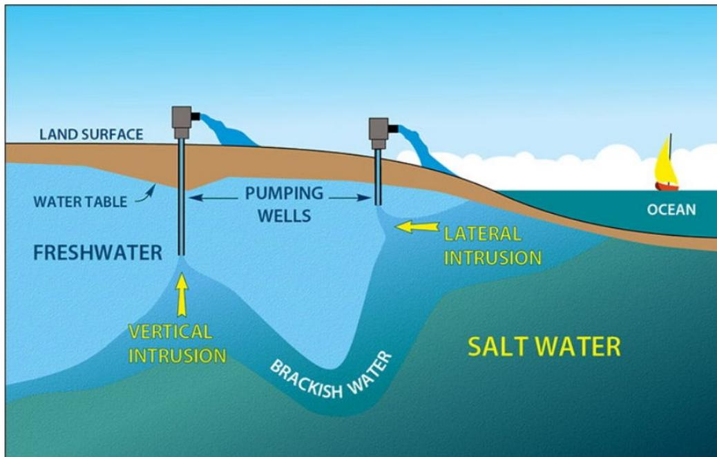
Figure 2. Conceptual drawing of lateral and vertical saltwater intrusion within coastal aquifers (Feltgen 2015).
