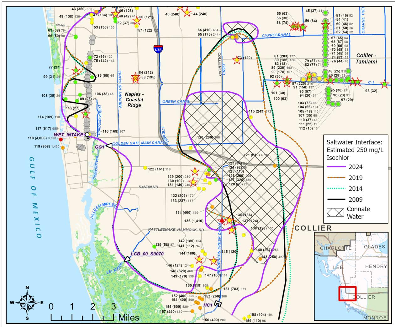
Figure 52. Position of the 2024 saltwater interface in the LTA indicating two areas of connate water in Collier County. Groundwater chloride concentrations in these connate water areas exceed 250 mg/L.
