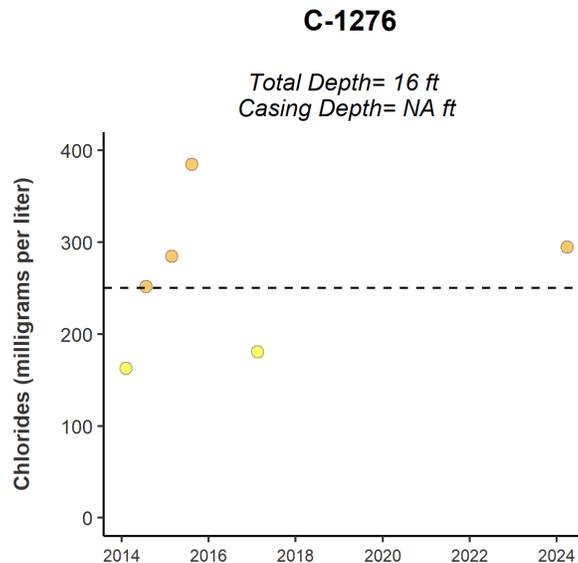
Figure 47. Chloride time-series plot for C-1276 in Collier County.
