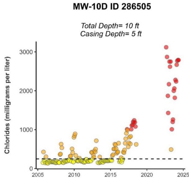
Figure 36. Chloride time-series plot for MW-10D ID 286505 and MW-10C near the Dixie PS wellfield in the City of Fort Lauderdale in Broward County.
