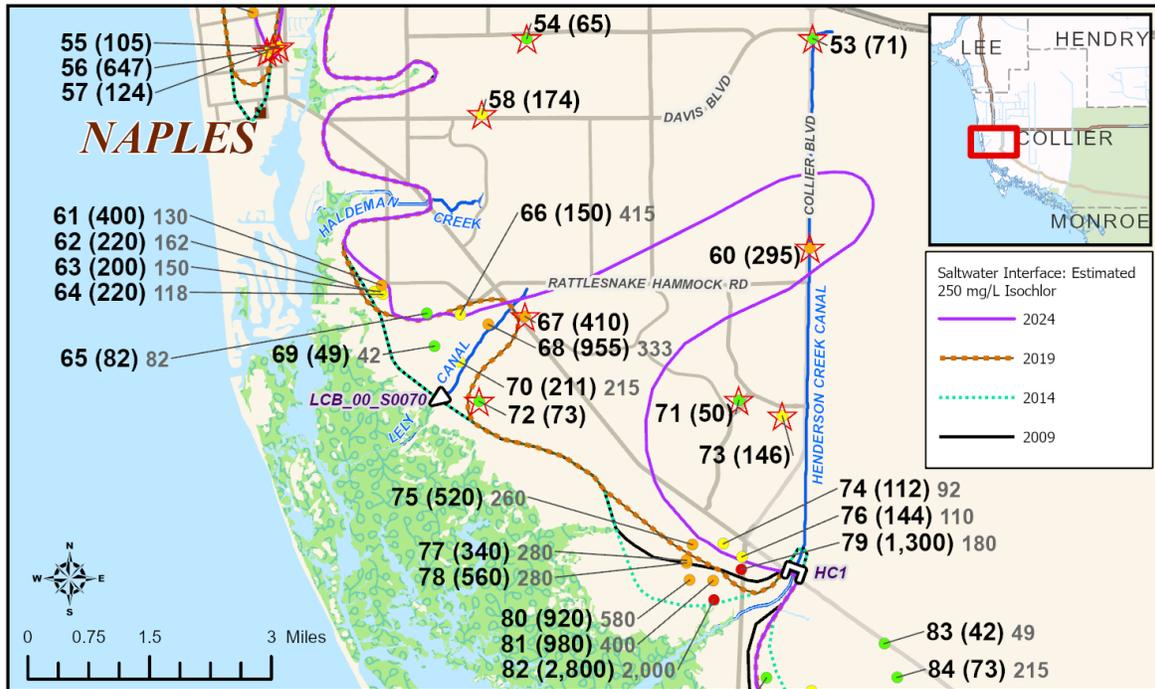
Figure 46. Position of the 2024 saltwater interface in the WTA near Henderson Creek Canal in central Collier County.
