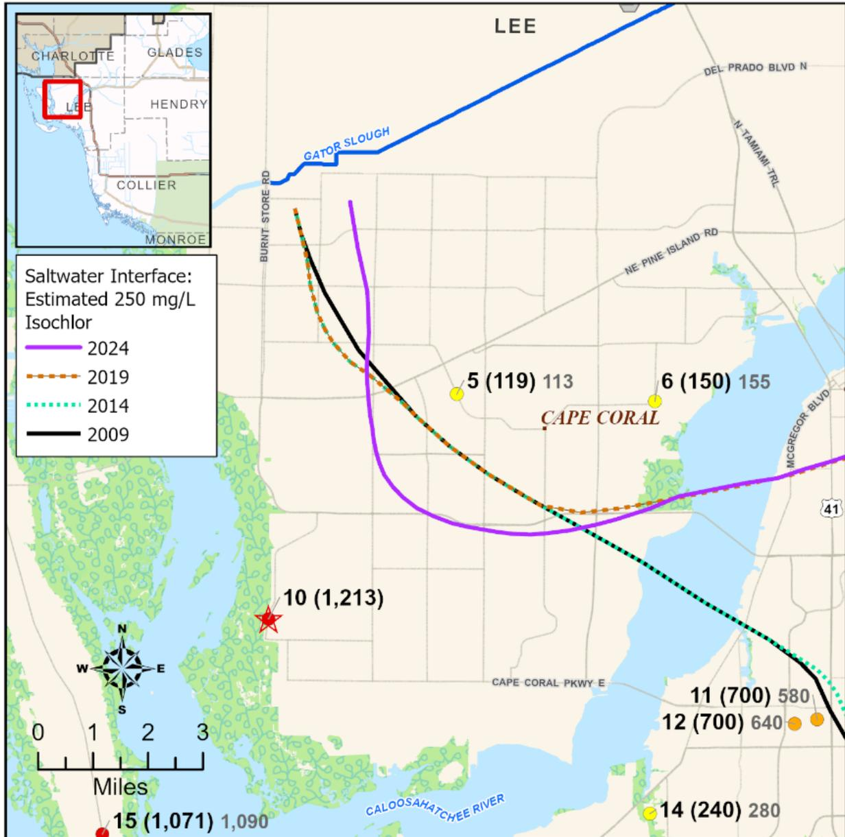
Figure 59. Position of the 2024 saltwater interface in the MHA in the City of Cape Coral in Lee County, reflecting the new groundwater chloride data point in the southwestern corner of the map, which had a 2024 groundwater chloride concentration of 1,213 mg/L.
