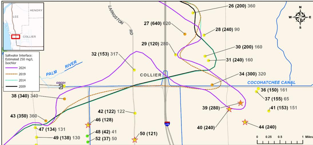
Figure 49. Position of the 2024 saltwater interface in the LTA near the Cocohatchee Canal in Collier County, primarily due to newly obtained data.
