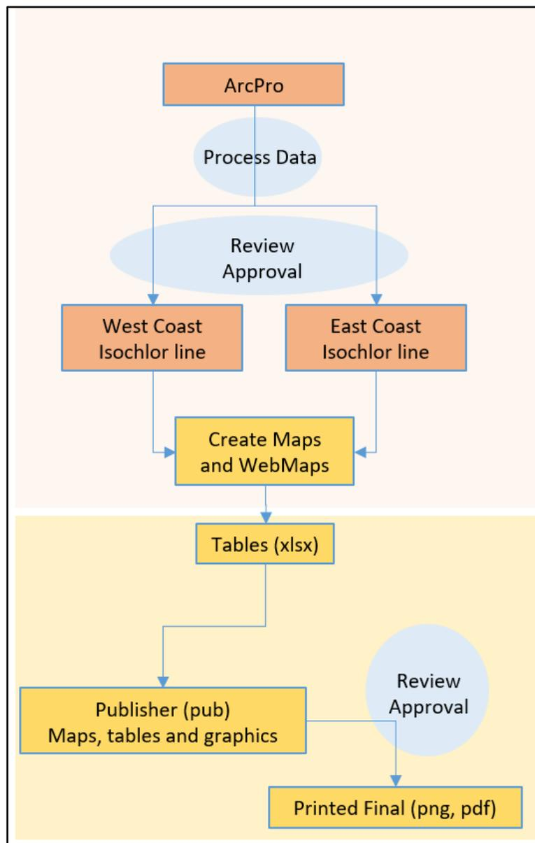
Figure 6. Saltwater interface mapping flow chart.
