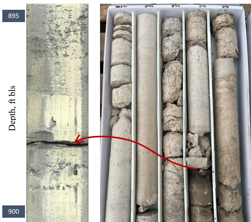
Figure 11. Typical appearance of MCU_I at OSF-108R. Image on the left is from the OBI log. Photo on the right is the core recovered from 890 to 900 ft bls. A partially open bedding plane, granular texture, and vugs are visible on both photos.
