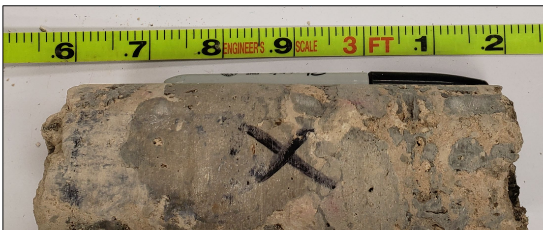
Figure 32. Photo of glauconitic marker unit sample from a depth of 1,647.4 ft bls that was analyzed using XRD.
