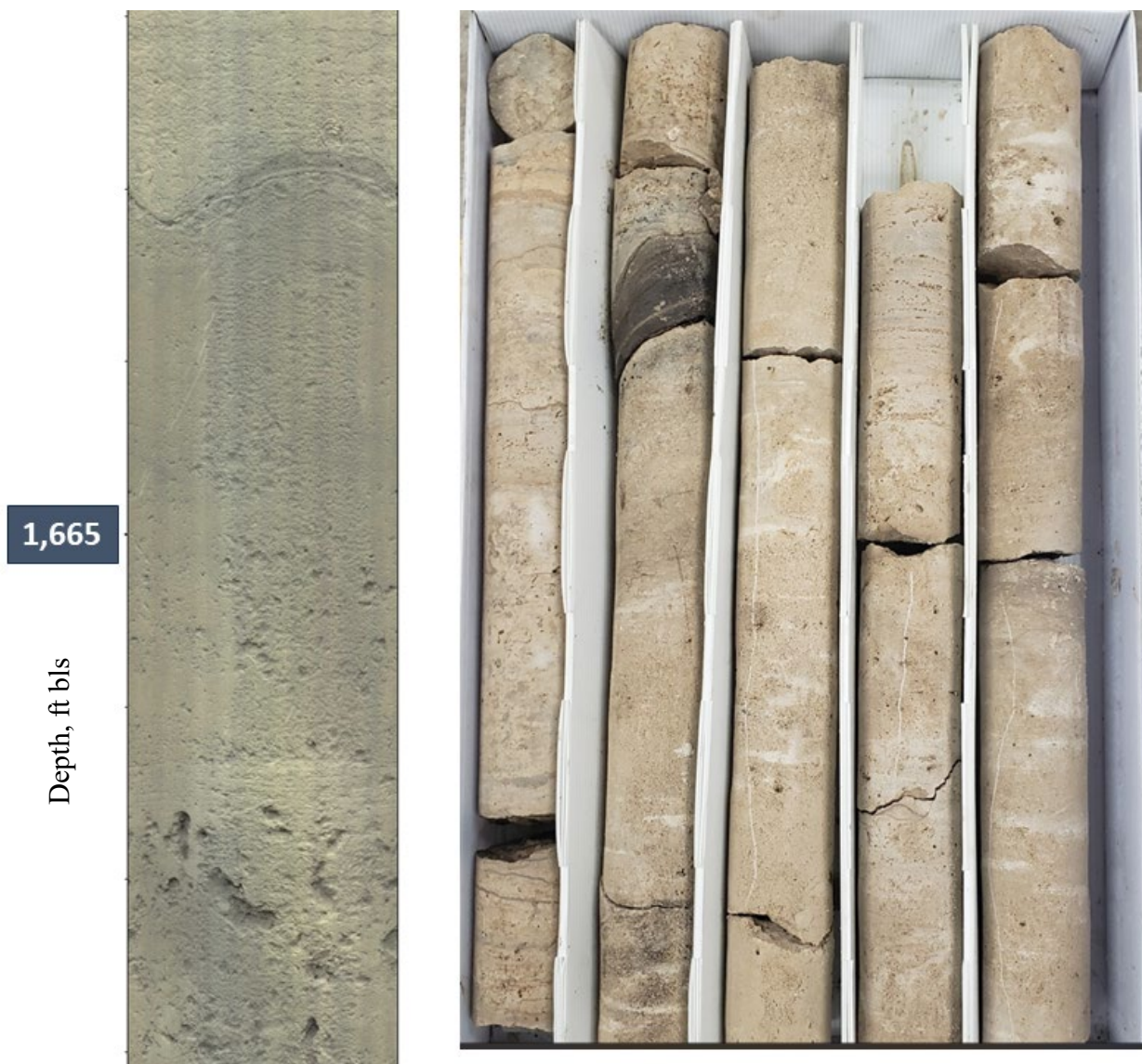
Figure 14. OBI image and photo of core from OSF-108R. OBI image depths are approximately 1,662 to 1,668 ft bls (left) and the cores shown here are from 1,660 (top left of the core box) to 1,670 ft bls (bottom right of the core box). These images show the lack of porosity within the GLAUC lpu .
