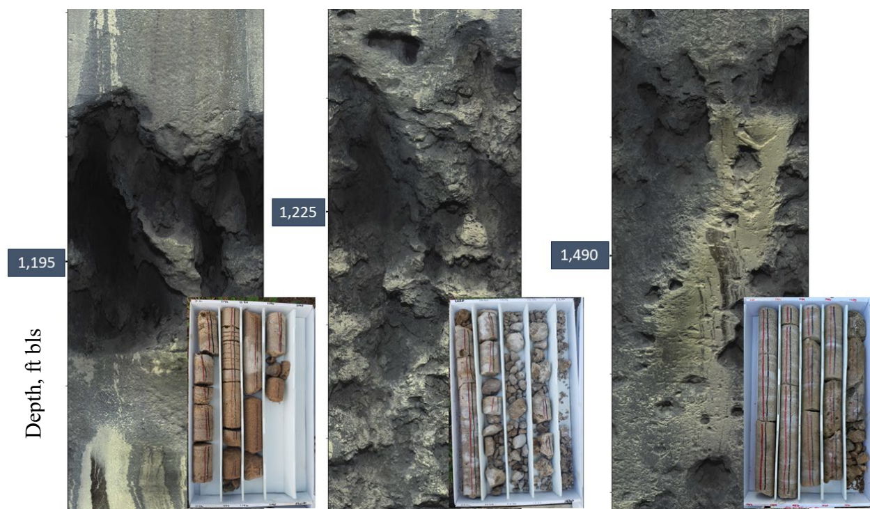
Figure 13. OBI images of a portion of LF1 (left and center) and LF3 (right) in OSF-108R showing abundant large vugs and granular texture.
