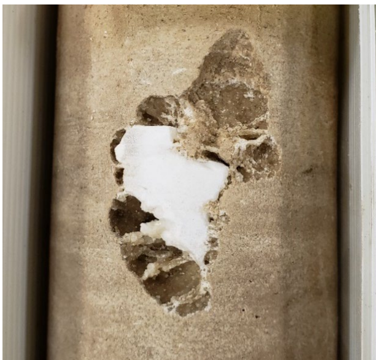
Figure 6. White quartz partially filling a vug in core sample from a depth of 1,536.5 ft bls.
