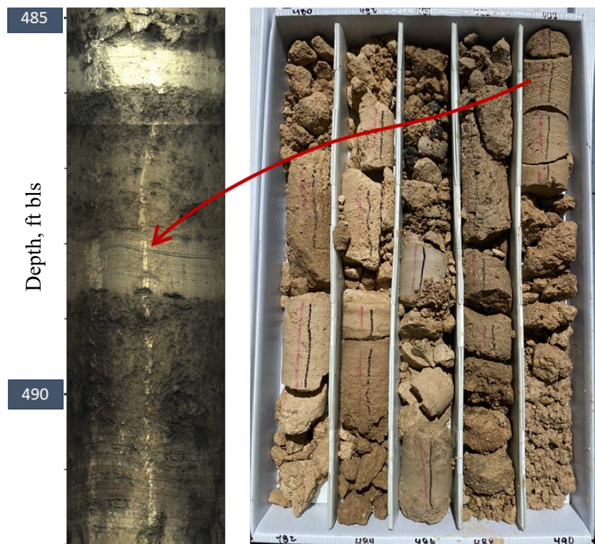
Figure 10. Typical appearance of relatively lower-hydraulic conductivity zones within the APPZ at OSF-108R. Note the vuggy texture above and below the finer-grained, laminated interval in the middle of the image. Depth interval for this image is 485 to 492 ft bls.
