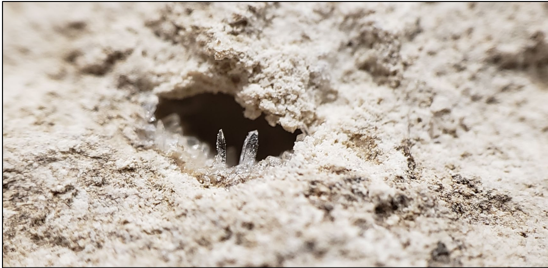
Figure 30. Photo of celestine crystals from a depth of 839.3 ft bls that were analyzed using XRD.
