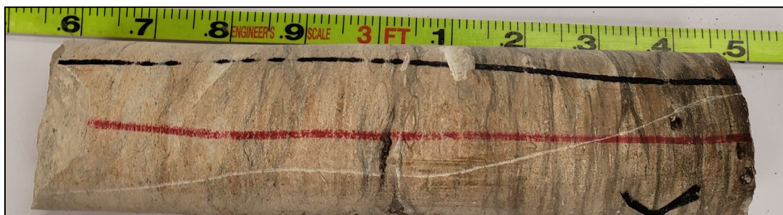
Figure 31. Photo of dark-colored clay-bearing laminations in the core sample analyzed by XRD. Potassium feldspar was also detected in this sample at a depth of 1,592.7 ft bls using XRD.
