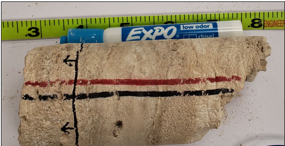
Figure 29. Photo of core from a depth interval of 839.3 to 839.8 ft bls. XRD test was completed on crystals (see Figure 30 ) at a depth of 839.3 ft bls.
