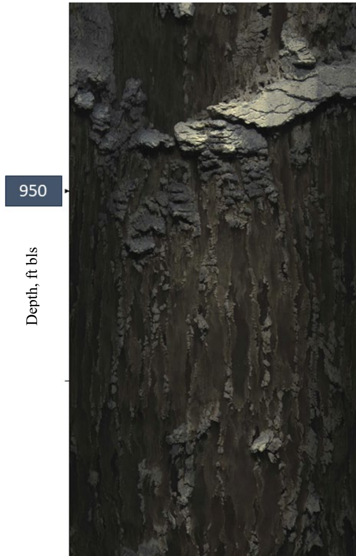
Figure 4. Curtain texture from 949 to 952 ft bls caused by rapid dissolution of evaporites following completion of coring.
