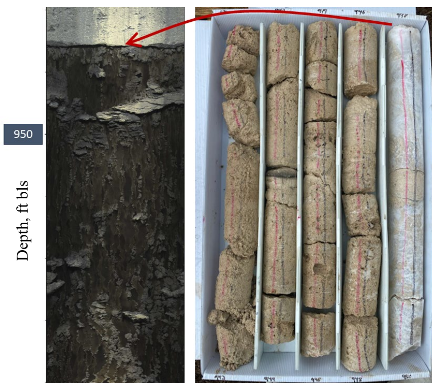
Figure 12. MCU_I to MCU_II transition at a depth of 948.5 ft bls as indicated by the red arrow. The OBI image on the left shows the interval from approximately 948 to 954 ft bls, and the photo on the right is of the core from 940 to 950 ft bls. The dolostone of MCU_I displays a typical vuggy texture (the four yellowish-brown core sample intervals on the left side of the core box). The evaporites of MCU_II display a lack of permeability (right most chamber of the core box with lighter colored, white and tan rock). The evaporites of MCU_II display substantial dissolution in the OBI imagery, which occurred rapidly between the end of reaming (July 30, 2021) and the OBI logging (August 31, 2021) when the rock was exposed to low TDS groundwater.
