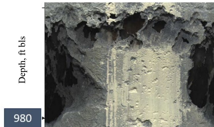
Figure 5. OBI log from 979 to 980 ft bls showing large vugs and voids within fine-grained carbonate.
