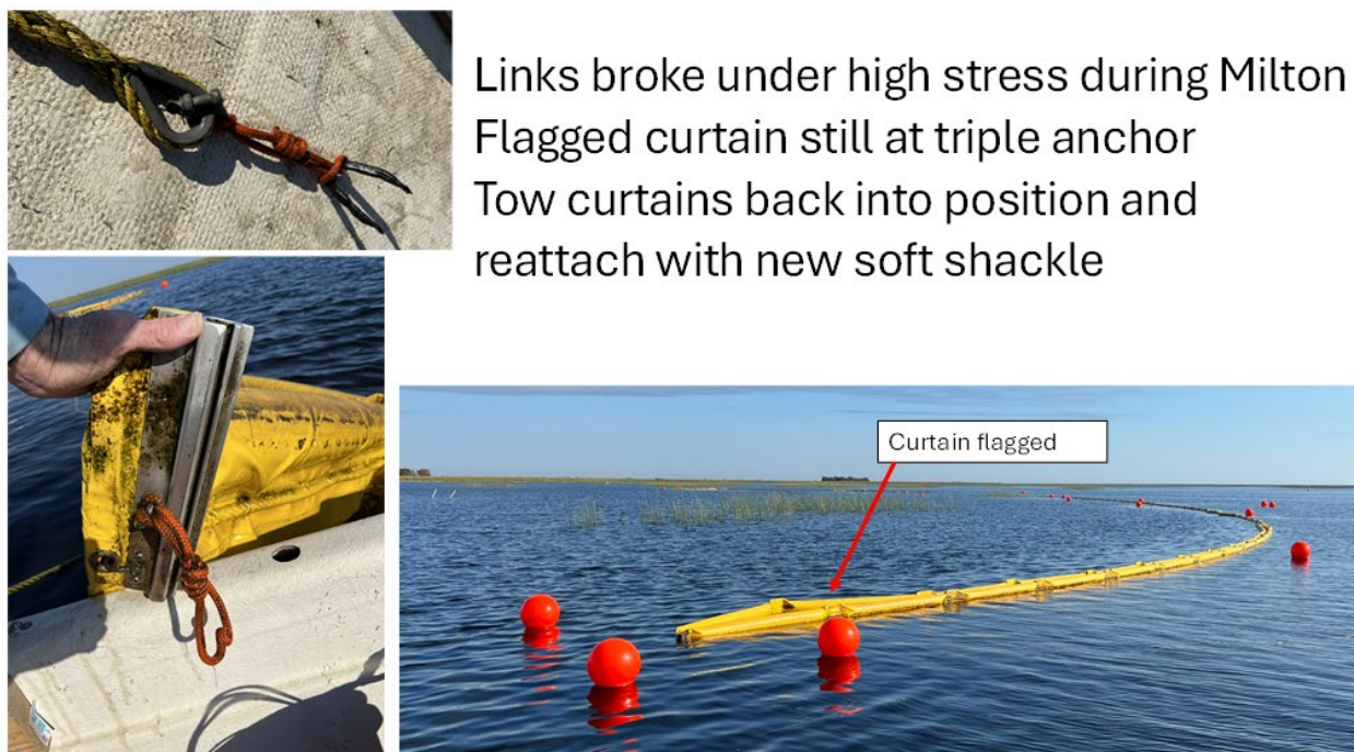
Figure 17. Broken links allowed the turbidity curtain to flag during the passage of Hurricane Milton, and remain anchored at one end for rapid reattachment.
