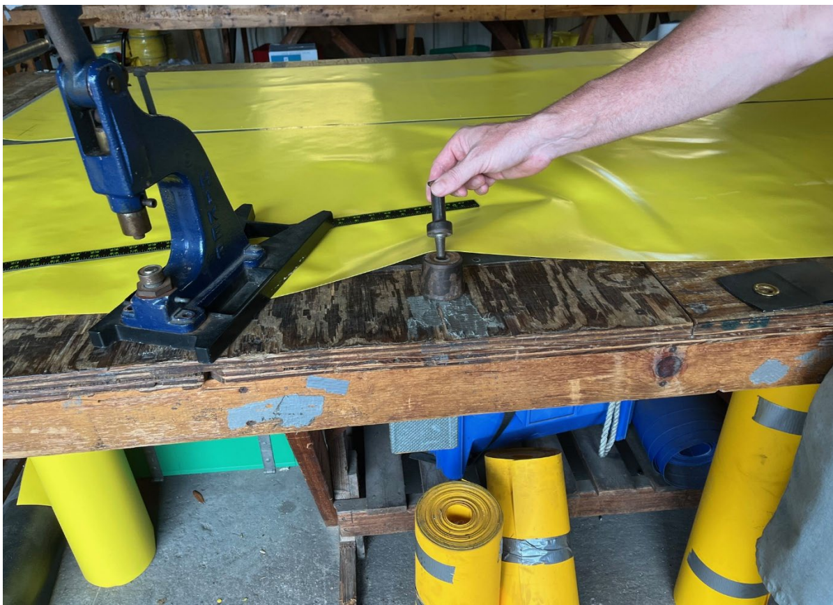
Figure 71. Grommet installation tools at manufacturing facility.
