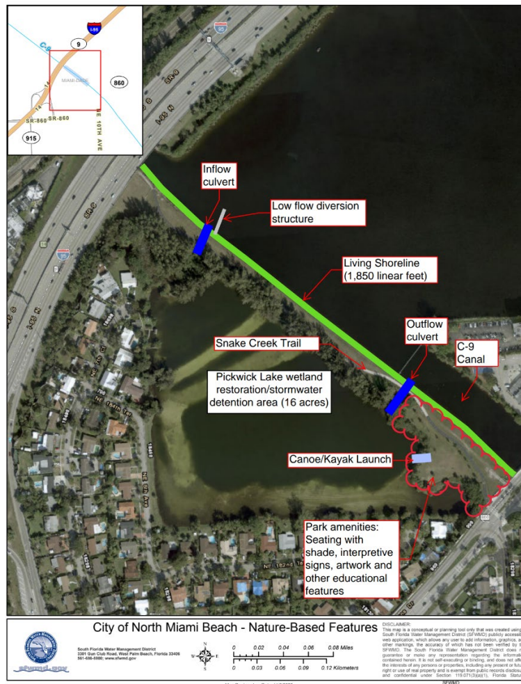
Figure 9-7: Pickwick Lake wetland restoration/stormwater detention area features.
