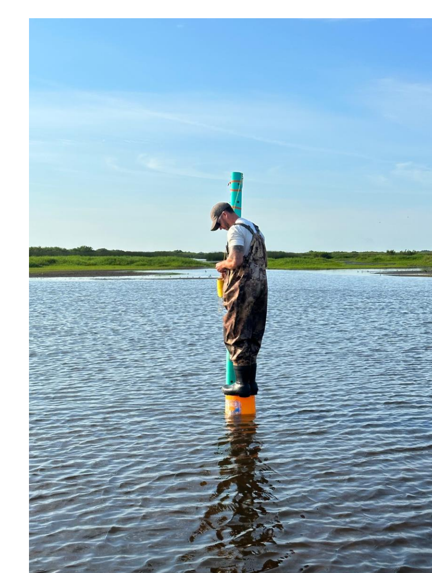
Researcher maintaining DO sensor.
