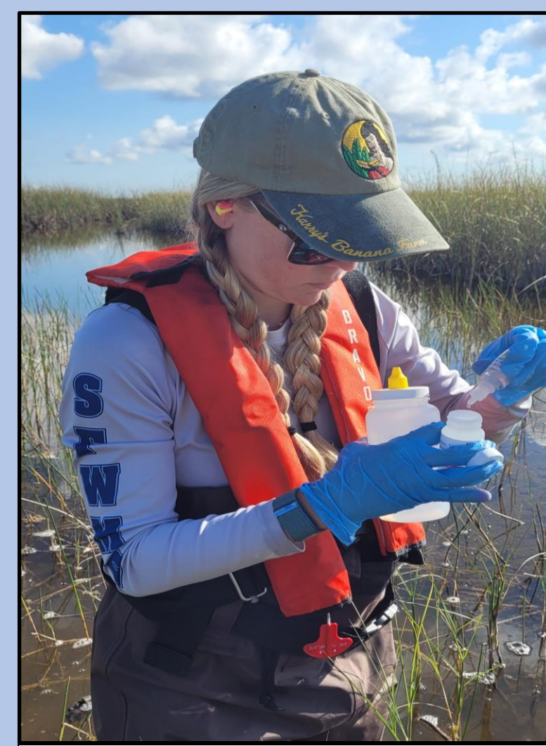
Station CA39 in WCA-3A. Adding acid needed for proper sample preservation.
