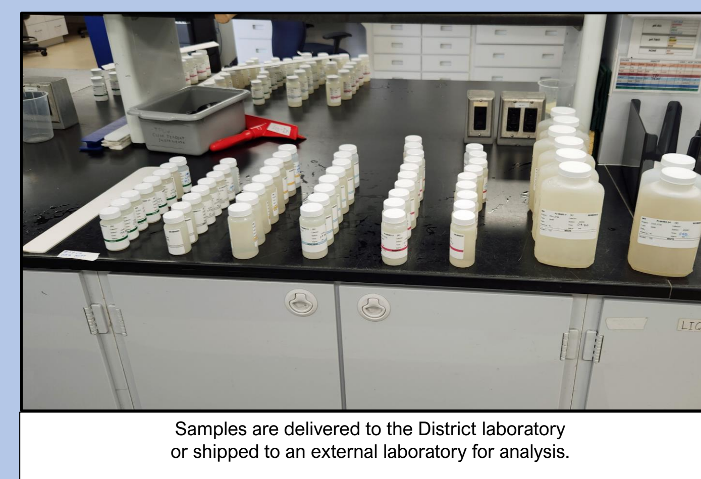
Samples are preserved (filtered, acidified, or chilled) in the field and submitted to the laboratory.
