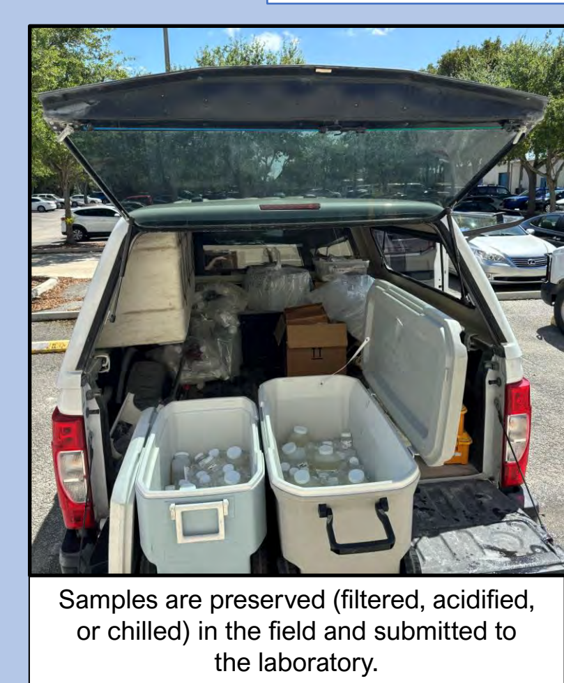
Samples are preserved (filtered, acidified, or chilled) in the field and submitted to the laboratory.
