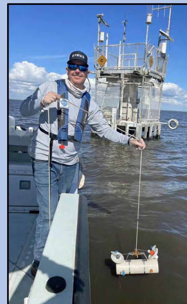
GRAB L001 water quality station on Lake Okeechobee. Collecting a water quality sample using a Van Dorn.
