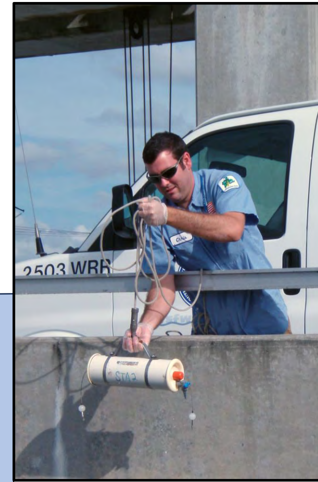
TRUCK S5A-E on the C-51 Canal. Collection of samples upstream of the gates using a Van Dorn.
