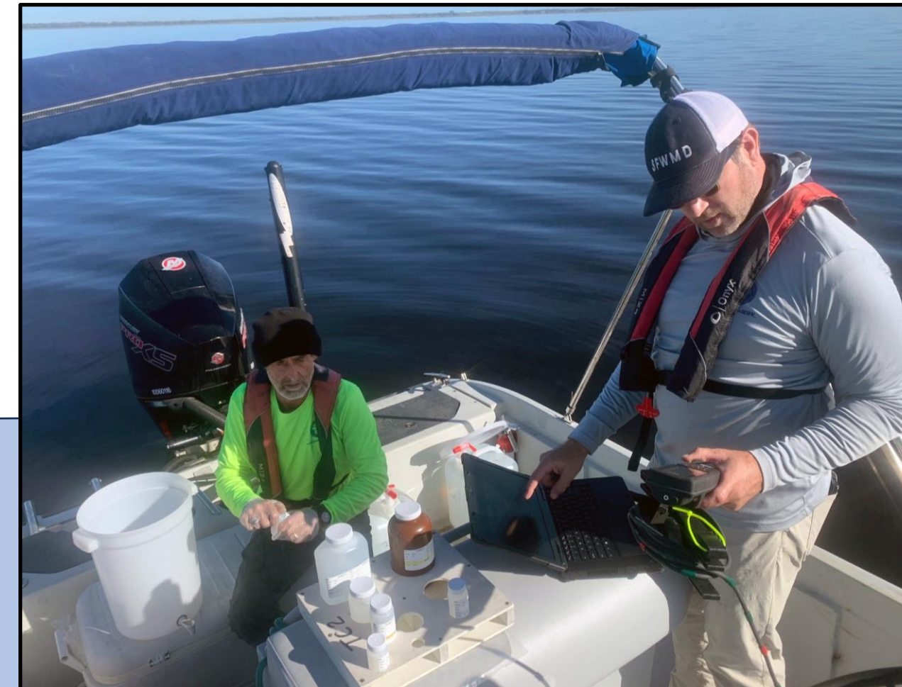
BOAT Station A03 in East Lake Tohopekaliga. Collection of surface water samples and multi-parameter sonde data.
