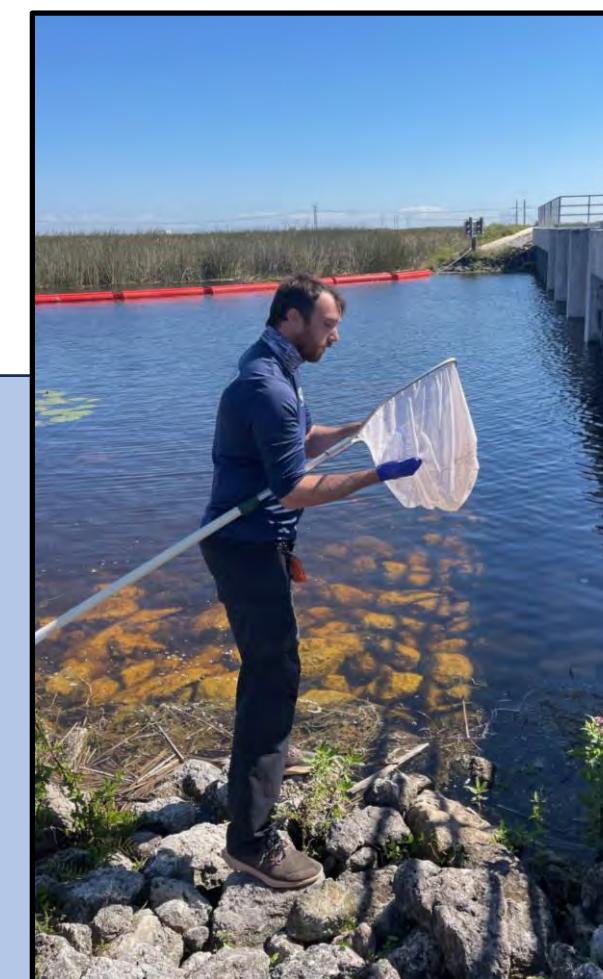
FISH COLLECTION G-734 in Stormwater Treatment Area (STA) 1W Expansion 1. Mosquitofish collection for mercury analysis.
