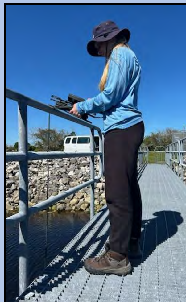
IN-SITU Field instruments measure pH, dissolved oxygen, temperature, specific conductance, and more.
