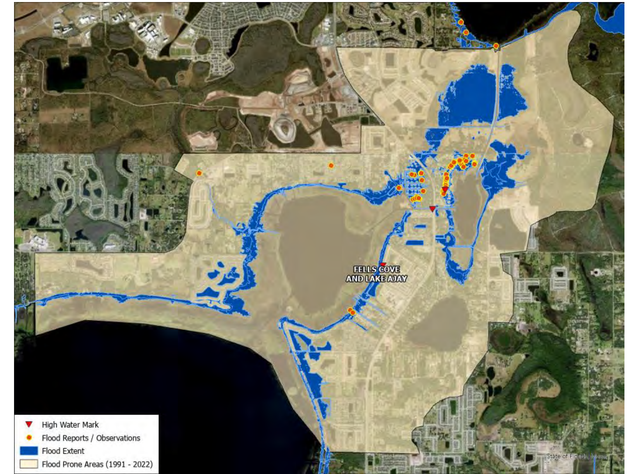
Figure 3. Example of measured flood extent within a flood prone area using a combination of radar and measured stage data.
