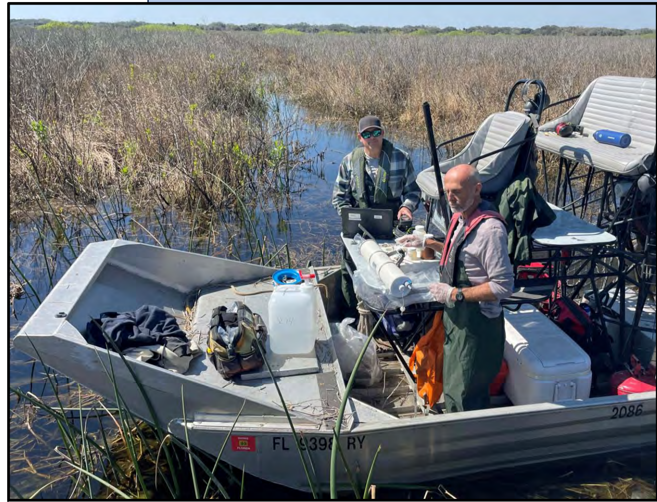
AIRBOAT Station PC34 on the Kissimmee River floodplain. Collection of surface water samples and multi-parameter sonde data.
