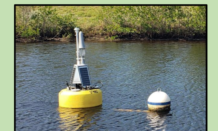
Manatee Mitigation Feature - North Pool Instrumentation buoy. Continuous Monitoring of temperature and specific conductance data.
