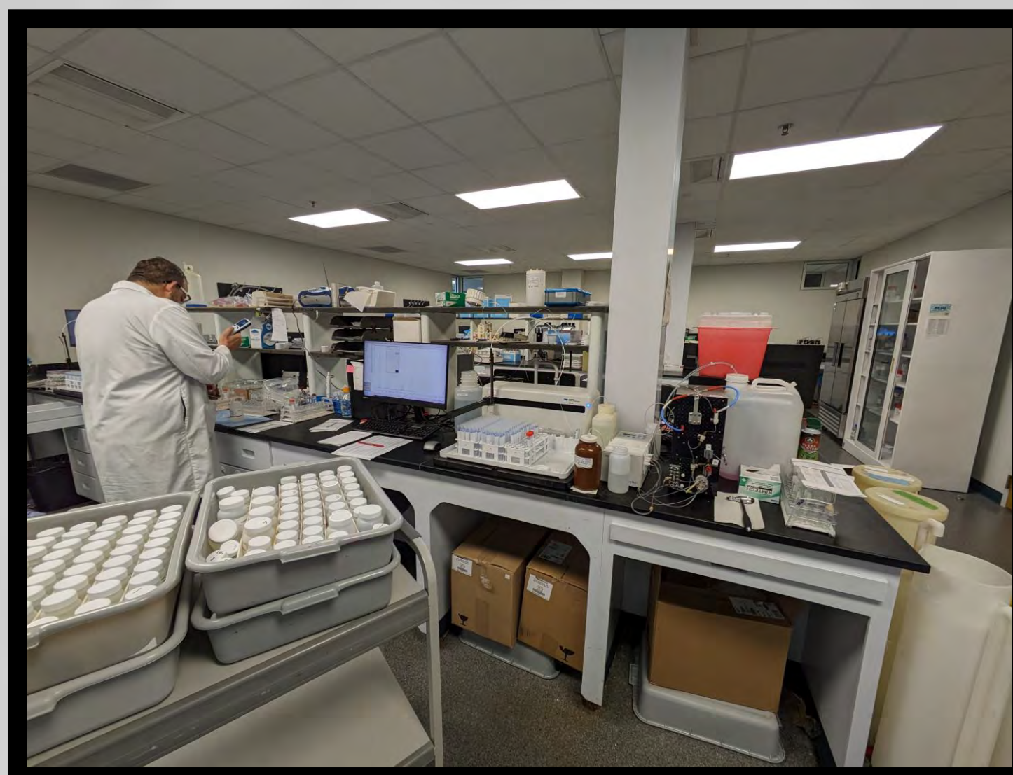
Total Nitrogen: Chemist performs analysis using the FIALab FIAlyzer FLEX instrument. This instrument is versatile and is used by SFWMD laboratory analysts to perform a wide variety of inorganic nutrient analysis (TP, TN, OPO 4 /NO 2 , NH 4 , SiO 2 , etc.).
