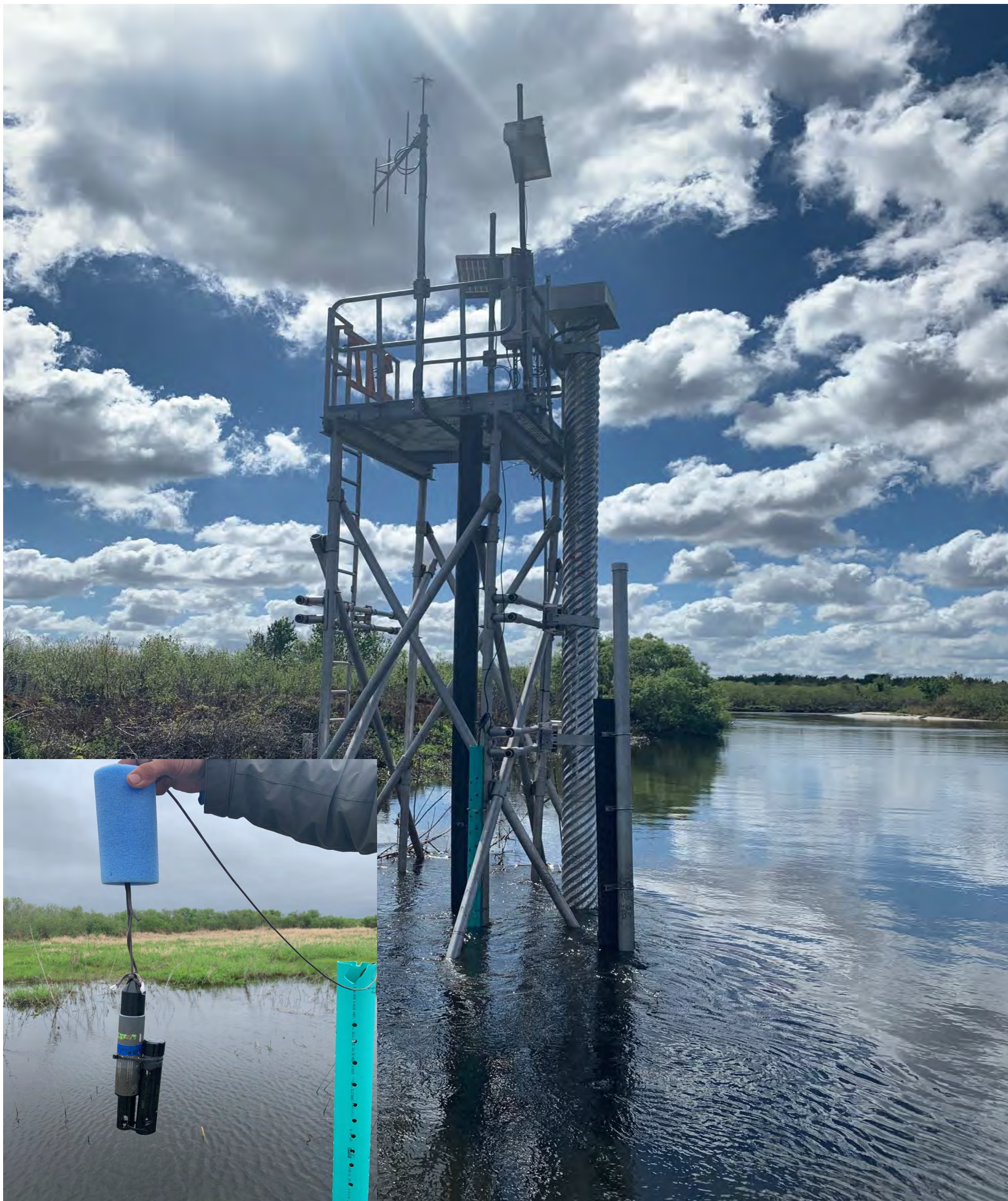
DO sensors are deployed at a network of monitoring sites along the Kissimmee River.
