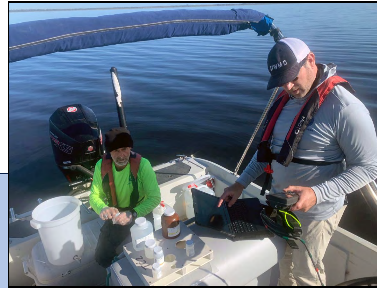
BOAT Station A03 in East Lake Tohopekaliga. Collection of surface water samples and multi-parameter sonde data.
