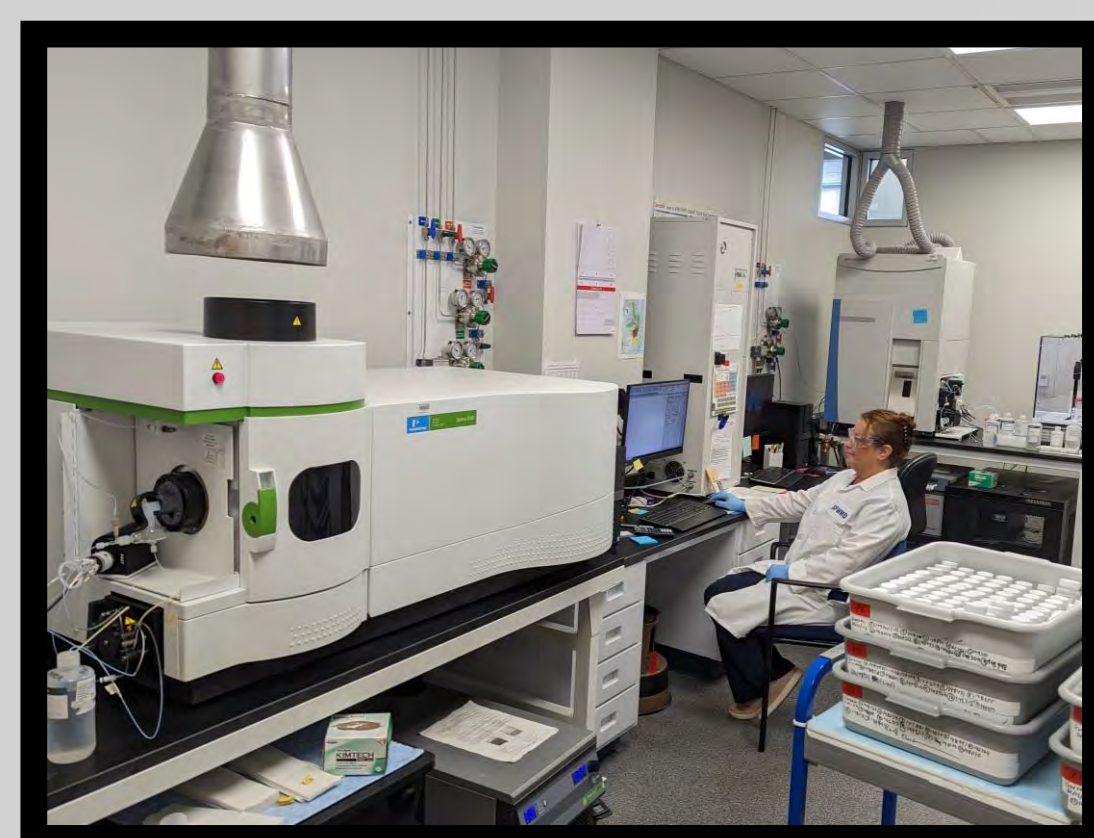
Chemist using ICP-OES to analyze various metals in the sample. See below for a list of the analytical instrumentation and associated procedures.
