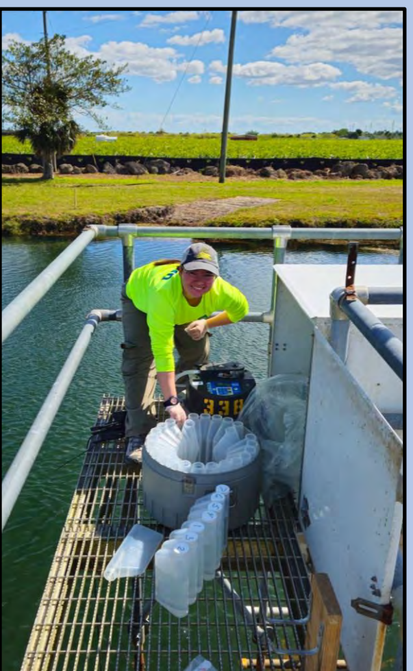
AUTOSAMPLER Station S332DX of the Everglades National Park Inflow North project. Autosampler retrieval and system setup for the next week's sampling.
