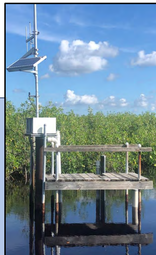
CONTINUOUS MONITORING Station SGT5W1 in Collier County. One of the 43 continuous monitoring locations transmitting data back to District servers.
