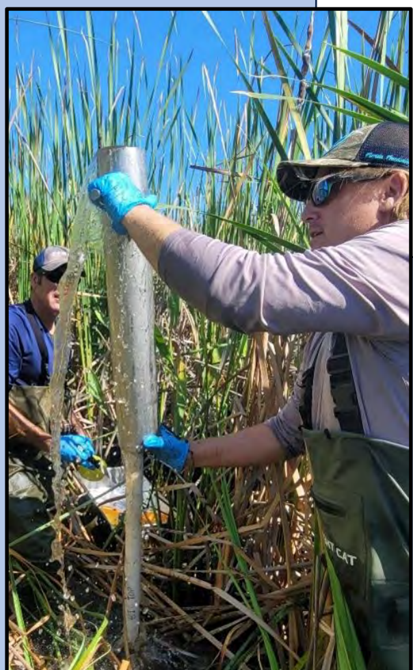
SEDIMENT FS transect in WCA-2A. Processing a sediment sample from a coring tube for laboratory submission.
