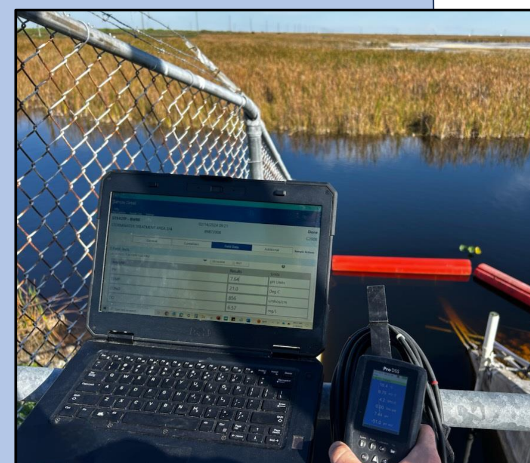
Station G390B in STA-3/4. Field observations and instrument data are entered directly into the computer in the field. This maximizes efficiency and minimizes errors through an abundance of built-in cross-checks. The data and information are uploaded directly into the Laboratory Information Management System (LIMS).
