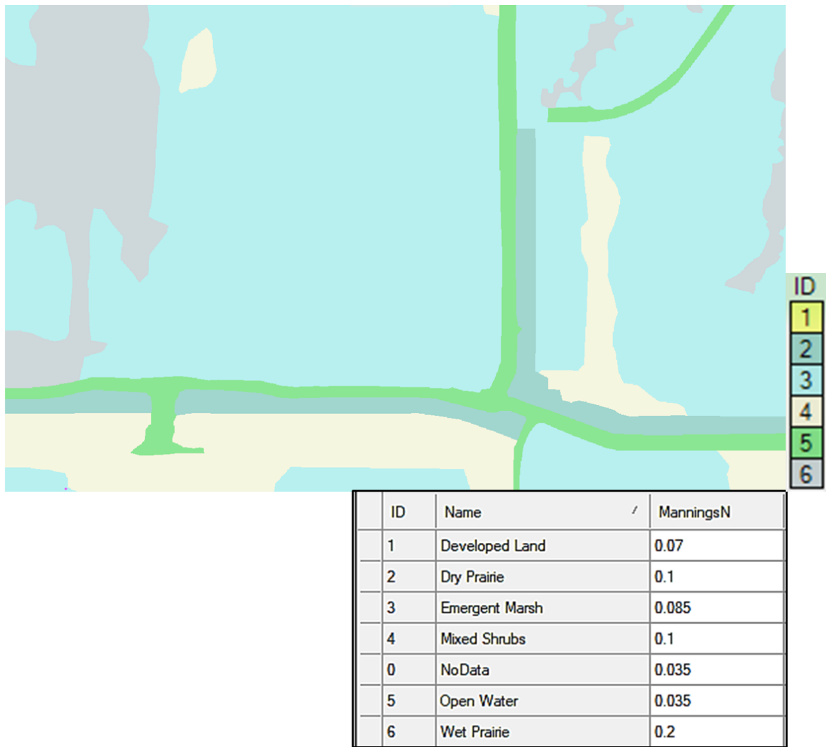
Figure 22. Manning's roughness coefficients based on vegetation distribution.
