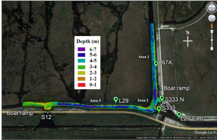
Figure 19. Bathymetry of the survey Area. Data collected on 05/16/2022.
