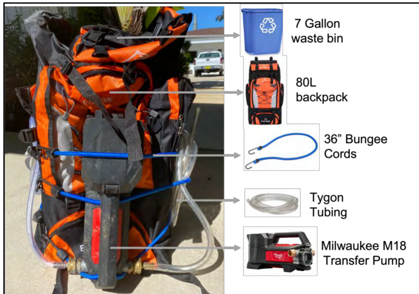
Figure 2.6. The materials needed to create a flocculation collection backpack for flocculation collection in a wetland system.
