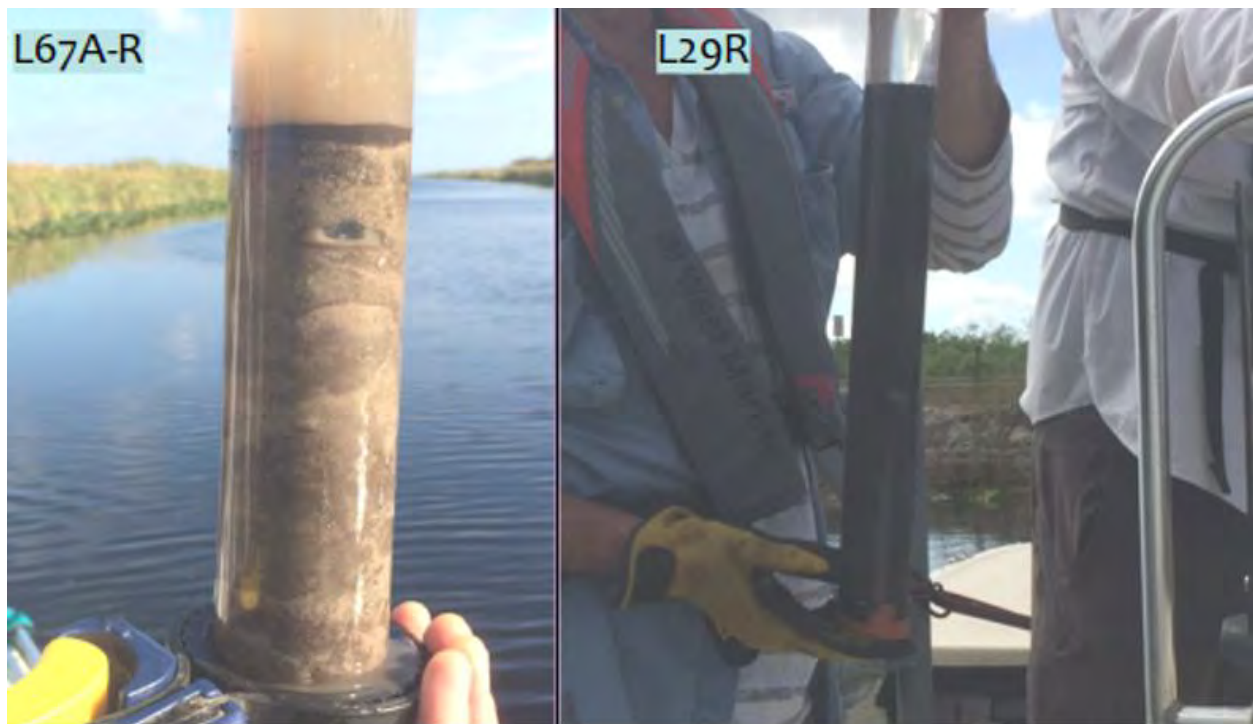
Figure 5: Sediment cores (pictures) taken in L67A-R and L29R. The abundance of organic mud (black) in L29R contrasts with the thin layer on top of the core at L67A-R, which is mostly carbonate sand (Briceño and Gardinali, 2018 ).
