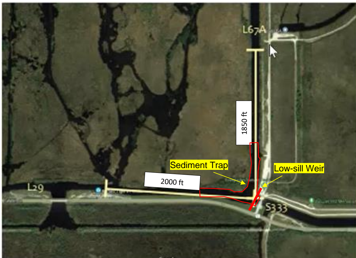
Figure 3. Assumed sediment trap and low-sill weir upstream of S-333 and S-333N complex. Red line indicates the boundary of the sediment trap.
