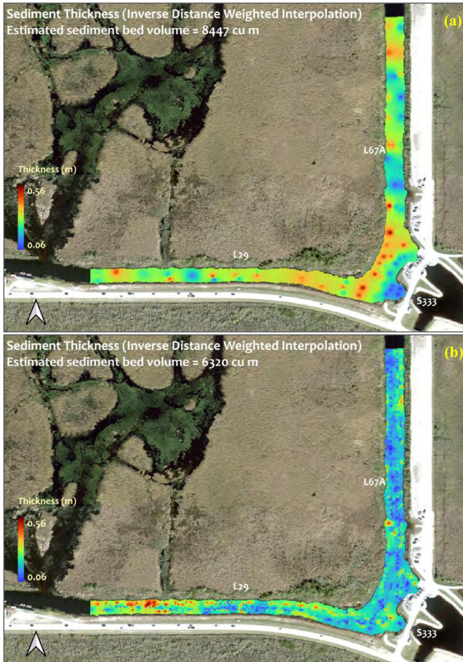
Figure 20. Inverse distance weighted (IDW) interpolation estimate of sediment profile thickness and bed sediment volume estimate; (a) from sediment core data (provided by University of Florida) and (b) from the ASV surveyed area on dates 04/06/2022, 04/07/2022, and 05/16/2022.
