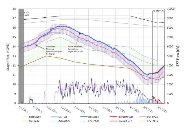
LAT forecasted Lake Okeechobee stages and flows assuming most recent S79 and S80 release targets established by the USACE (S79/S80: 500/0). PA25-simulated ROs are initiated on September 1<sup>st</sup>, 2024 (early start), resulting in observed and forecasted stages tracking above the PA25 simulation line.
