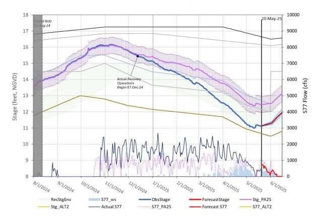
LAT forecasted Lake Okeechobee stages and flows assuming most recent S79 and S80 release targets established by the USACE (S79/S80: 500/0). ROs were not applied to the PA25 simulation, resulting in observed and forecasted stages tracking below the PA25 simulation line.
