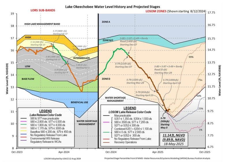
Stage is plotted in NGVD. Please use the left axis for water level history and projected stages. Lake Okeechobee stage NAVD88 offset of -1.25 is based on Final Regulation Schedule Conversion (5/19/2020).
