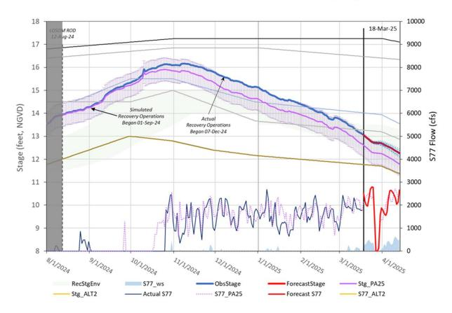
LAT forecasted Lake Okeechobee stages and S-77 flows with 2100 cfs flow target at S-79 and 1200 cfs flow target at S-80 consistent with recovery operations. PA25-simulated recovery operations are initiated on September 1<sup>st</sup>, 2024 (early start), resulting in observed and forecasted stages tracking above the PA25 simulation line.
