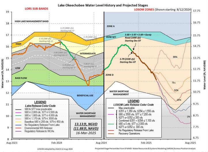
Stage is plotted in NGVD. Please use the left axis for water level history and projected stages. Lake Okeechobee stage NAVD88 offset of -1.25 is based on Final Regulation Schedule Conversion (5/19/2020).
