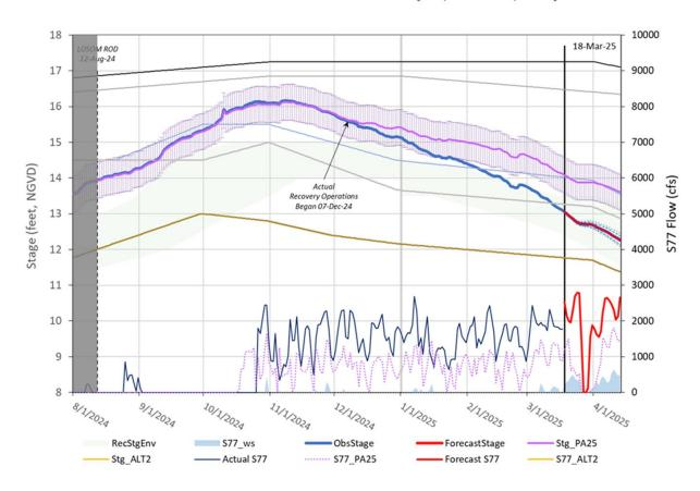
LAT forecasted Lake Okeechobee stages and S-77 flows with 2100 cfs flow target at S-79 and 1200 cfs flow target at S-80 consistent with recovery operations. Recovery operations were not applied to the PA25 simulation, resulting in observed and forecasted stages tracking below the PA25 simulation line.
