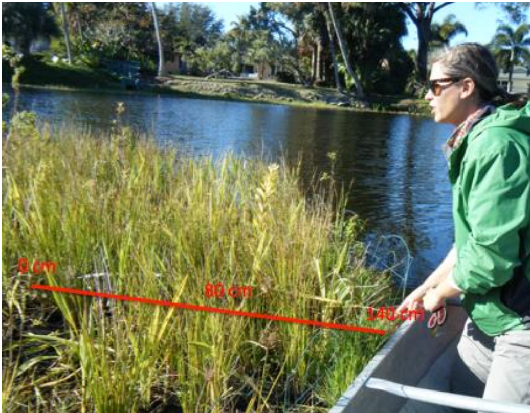
Figure 3. The transect run from the center to the edge of the FTW for microbial community characterization sampling. All samples were collected from the edge to the center at 0 cm, 80 cm, and 140 cm.
