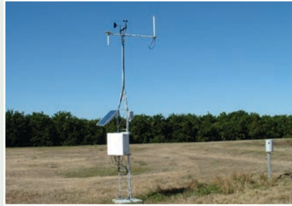
Weather Station with Telemetry
