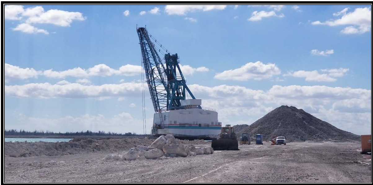
WRQ mining operation - A dragline excavating limerock
