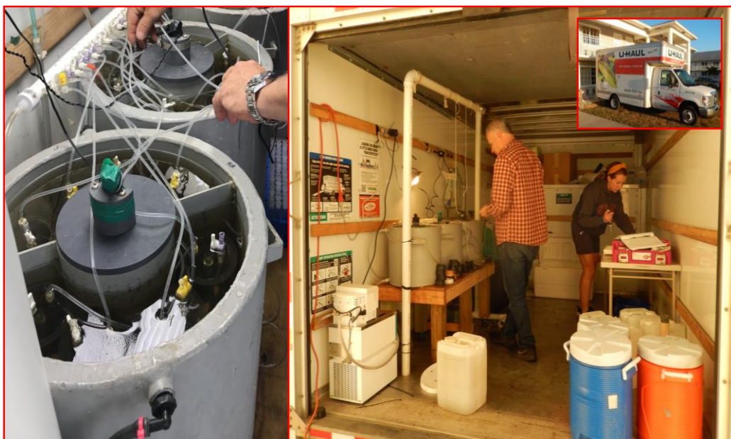
Figure 4. A rental box truck used for an incubation laboratory (December 2018). Double wall incubators were kept at field temperatures using a heating/cooling circulator. The white PVC frame was used to hang compact fluorescent lights for illuminated incubations.
