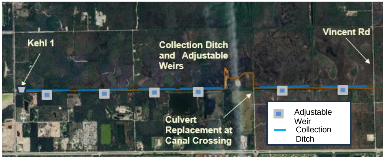
Figure 5-31. Kehl Canal Repair Project Features
