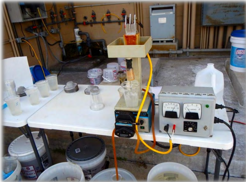
EC Treated / Separation with NO Chemicals or Polymers / 1 L/Min ECpw Lab Unit
