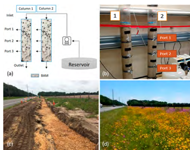
Figure 1. (a) Schematic diagram for column setup. (b) Column study—laboratory view, (c) field construction with BAM deployment, and (d) after construction for cotreatment of groundwater and stormwater.
