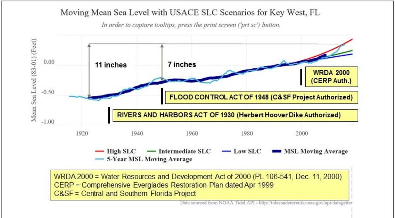
Figure 10. USACE SLC curves for Key West over 30 years from June 1988 to June 2018.
