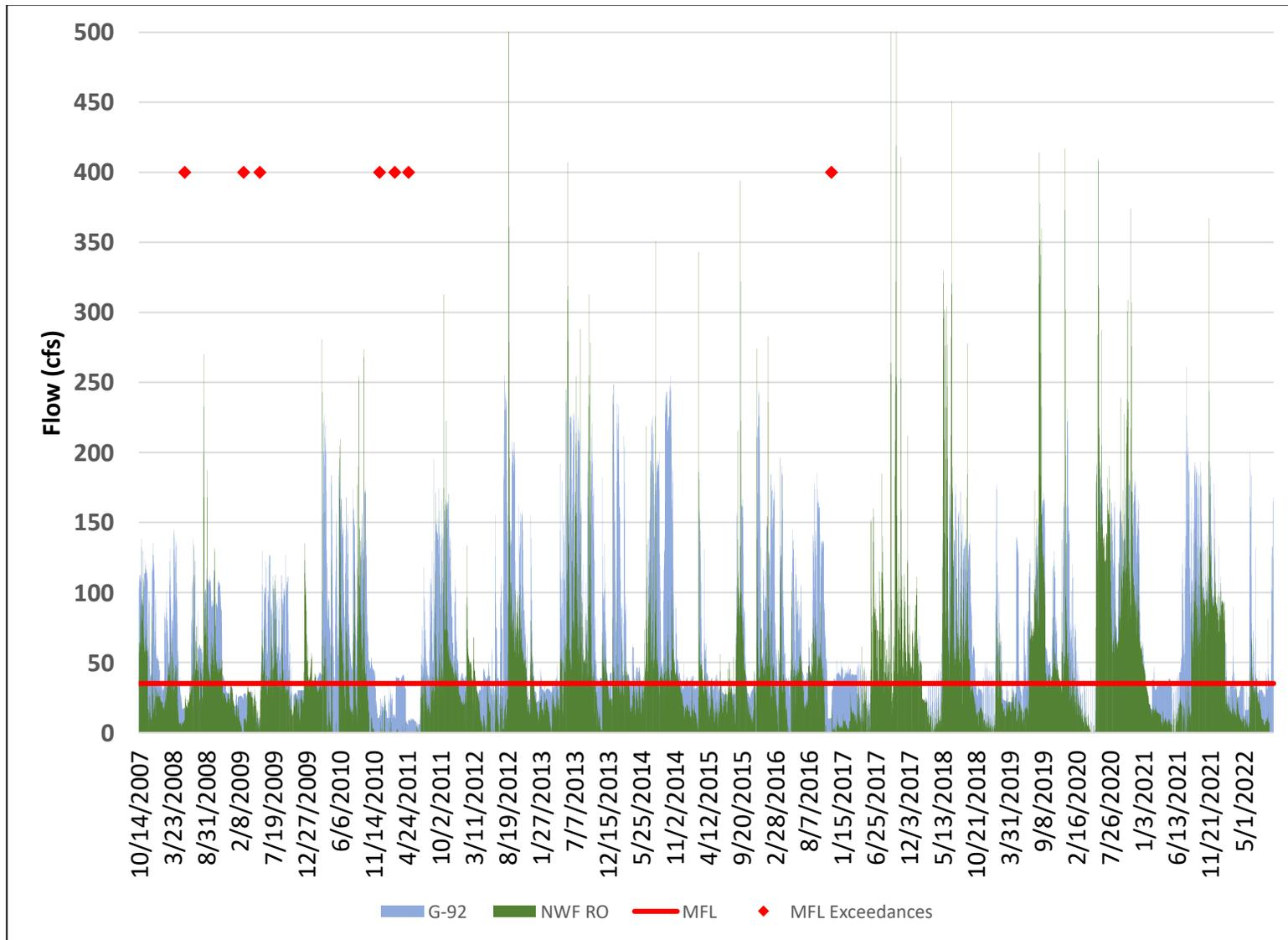
**Figure 4.** Stacked bar chart of Lainhart Dam flows by primary source. MFL exceedances are shown with diamond symbols. Vertical axis is truncated at 500 cfs to enhance clarity at lower flows.
