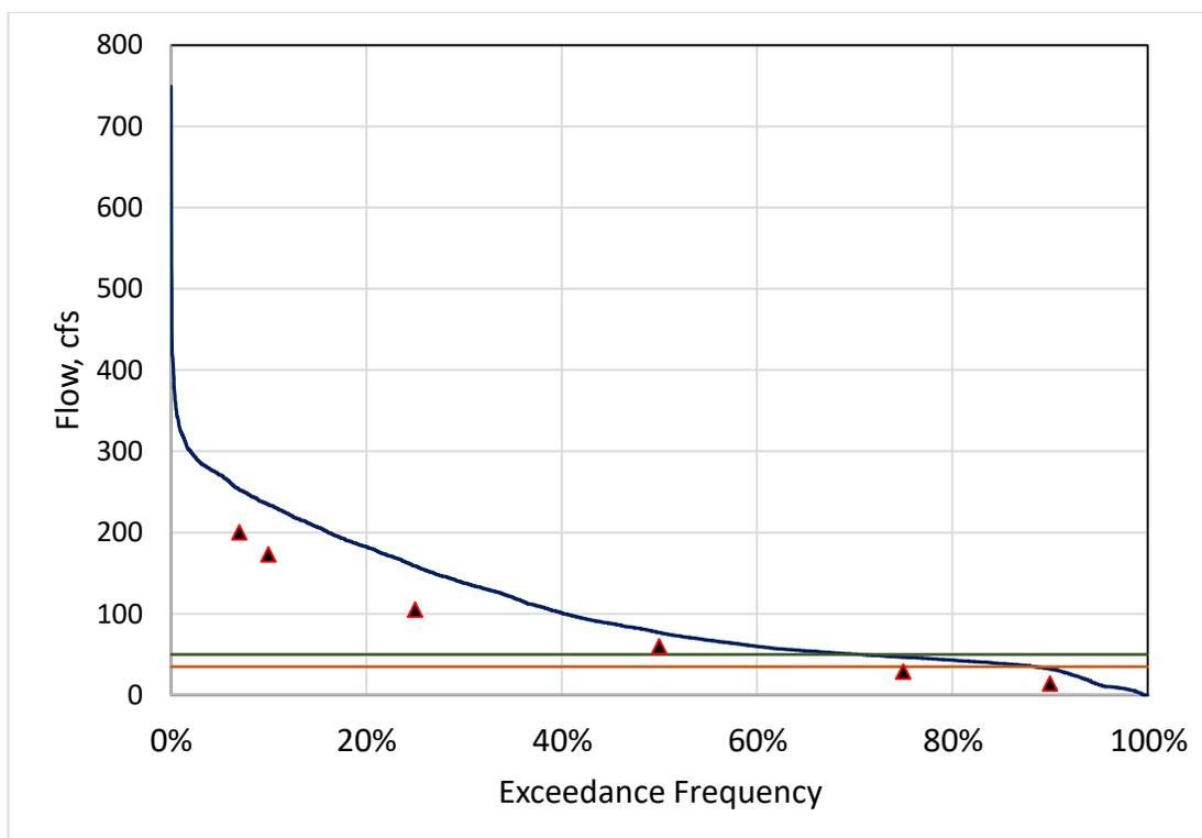
**Figure 3.** Lainhart Dam flow frequency curves from 1971–2001 (triangles) and 2007–2022 (black line). Horizontal lines reference 35 and 50 cfs.
