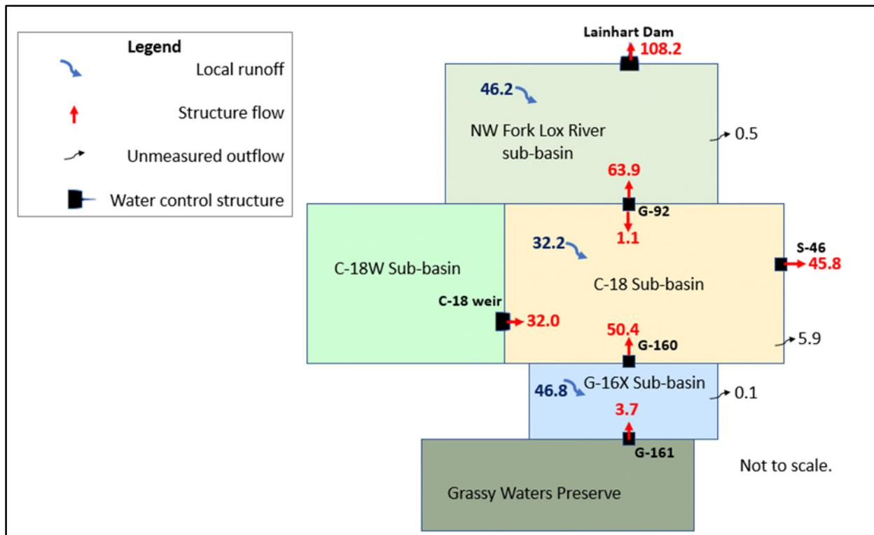
**Figure 2.** Diagram of the C-18 basin and subbasins (control volumes). Numbers are average flow rates in cubic feet per second (cfs). Inflows and outflows for each subbasin sum to nearly zero.
