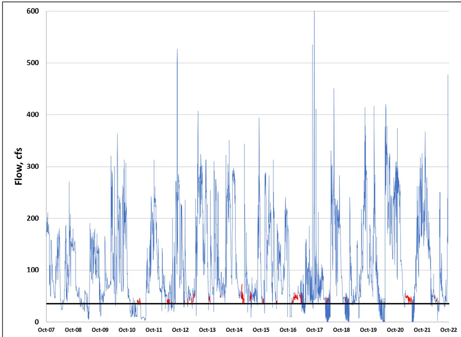
**Figure 5.** Lainhart Dam flow hydrograph (blue) with times when flow originating from G-161 raised the total flow over Lainhart Dam to 35 cfs or greater (red). Vertical axis is truncated at 600 cfs to enhance clarity at lower flows.
