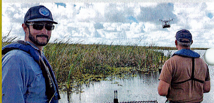
Mapping floating tussocks in an STA using a drone equipped with imaging sensors. (Photo by SFWMD)
