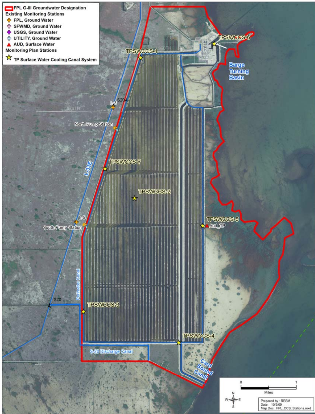
Figure 2-2. CCS monitoring stations.
