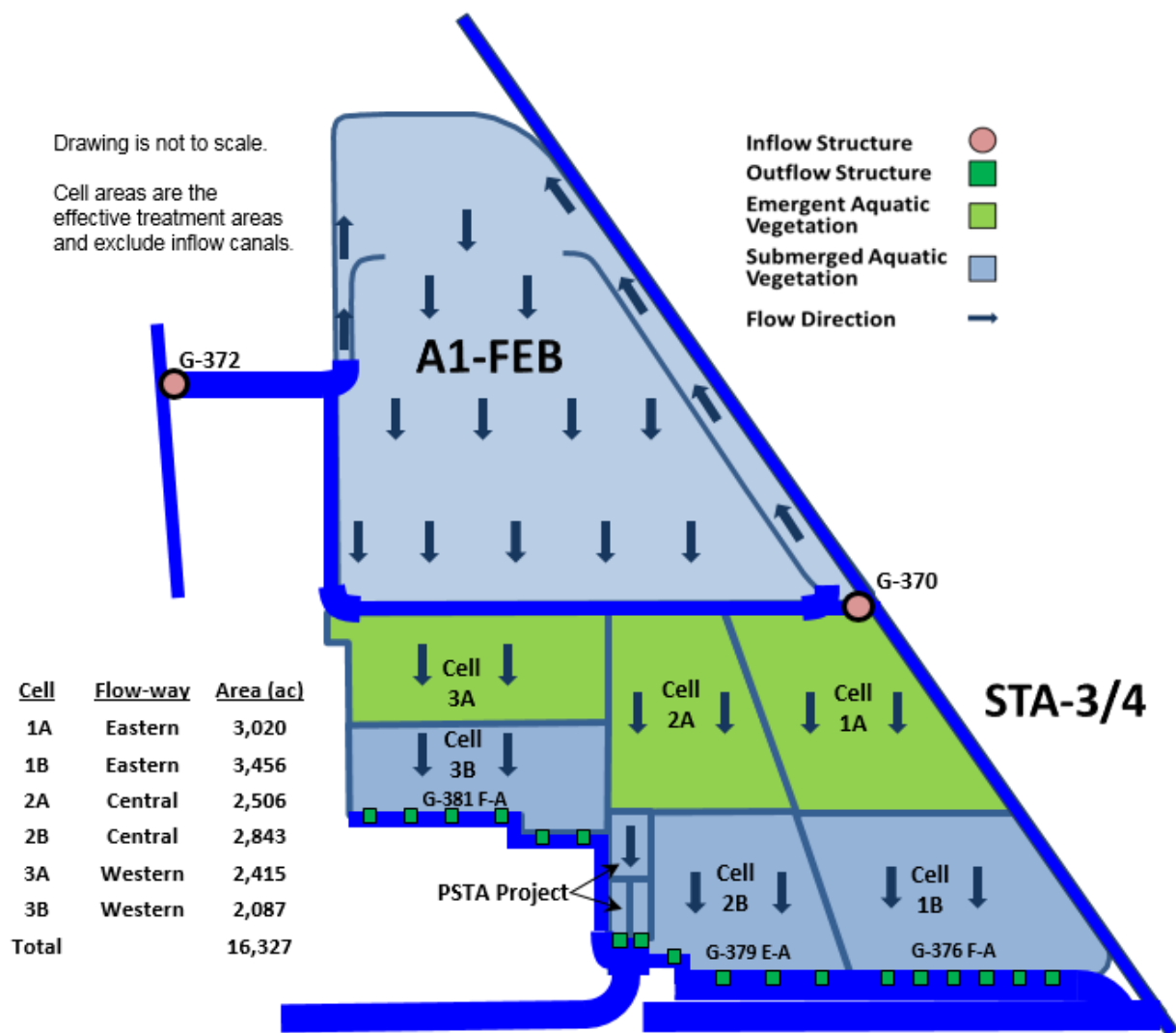
Figure 5B-10. Simplified schematic of STA-3/4 and the A-1 FEB showing major inflow and outflow water control structures, treatment area of each cell, flow direction, and dominant/target vegetation types. Treatment areas do not include pump stations, levees, roads, or other upland areas. Detailed structure maps of STA-3/4 and the A-1 FEB are provided in Appendix 5B-1 of this volume.
