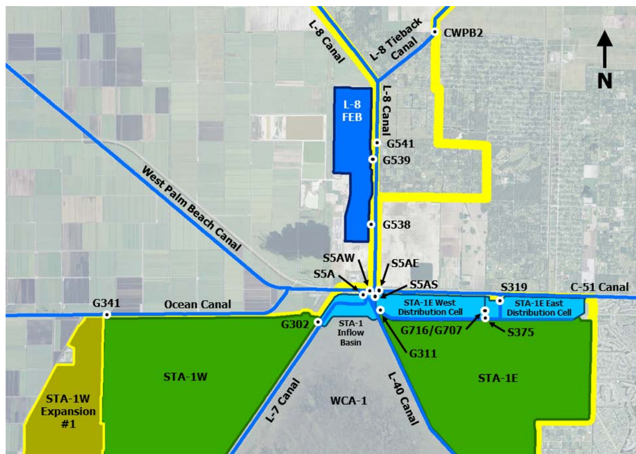
Figure 5A-2. Eastern Flow Path project components: L-8 FEB, L-8 Divide Structure (G-541), S-5AS Modifications, and STA-1W Expansion #1. Names preceded with an S denote structures constructed by the United States Army Corps of Engineers. Names preceded with a G denote structures constructed by the District. (Note: WCA-1 – Water Conservation Area 1.)
