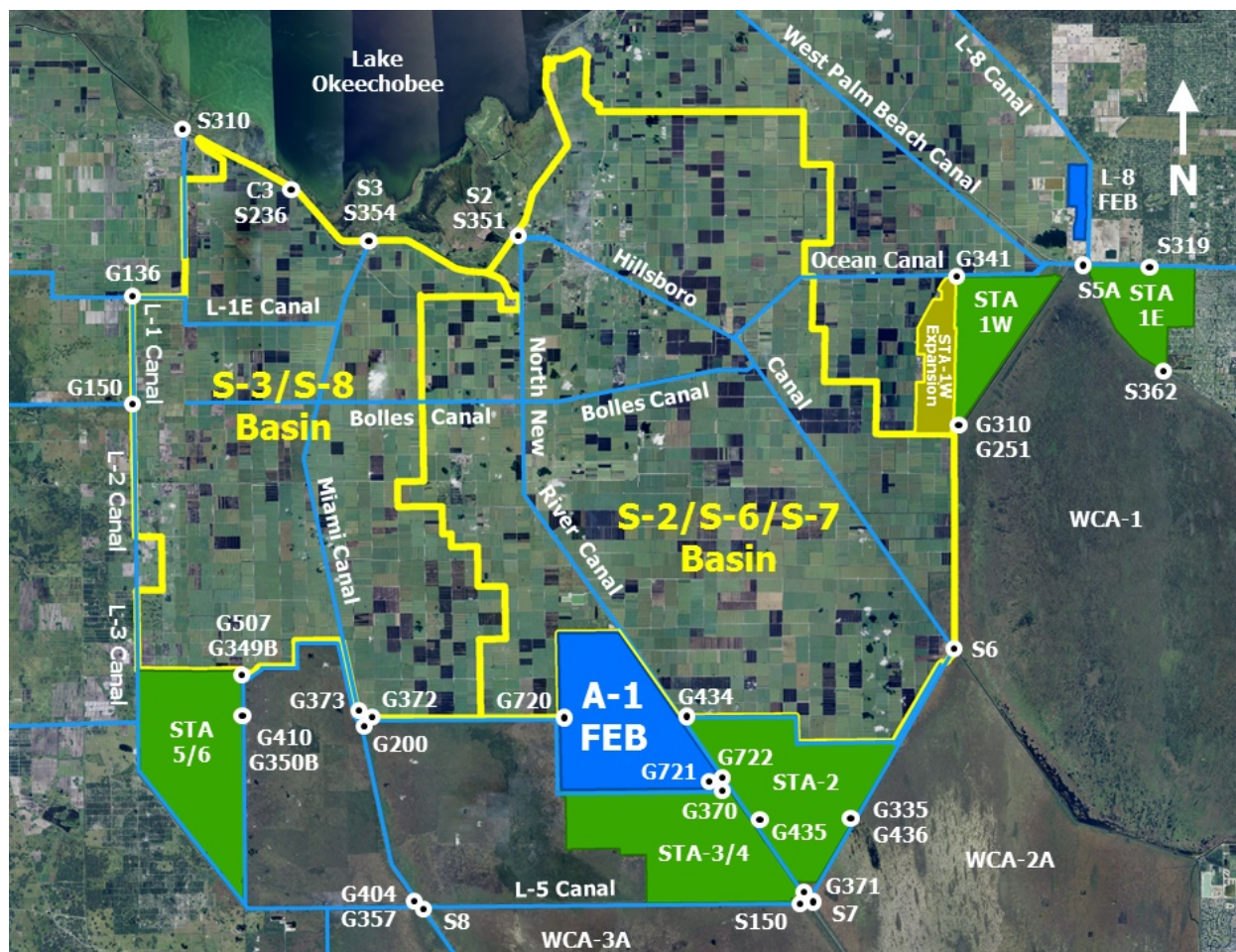
Figure 5A-9. A-1 FEB, Everglades STAs, and related canals and structures. Names preceded with an S denote structures constructed by the USACE. Names preceded with a G denote structures constructed by the District. (Note: WCA – Water Conservation Area.)
