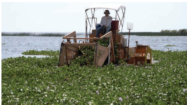
Mechanical harvesting of floating plants.
