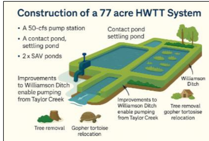
Water Treatment and Infrastructure
