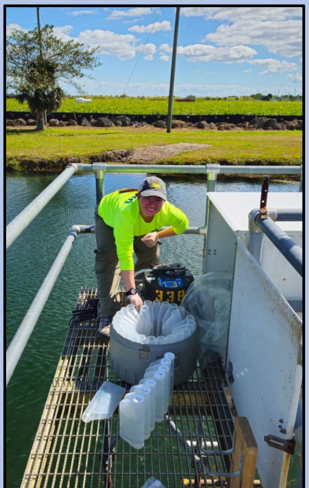
AUTOSAMPLER Station S332DX of the Everglades National Park Inflow North project.
