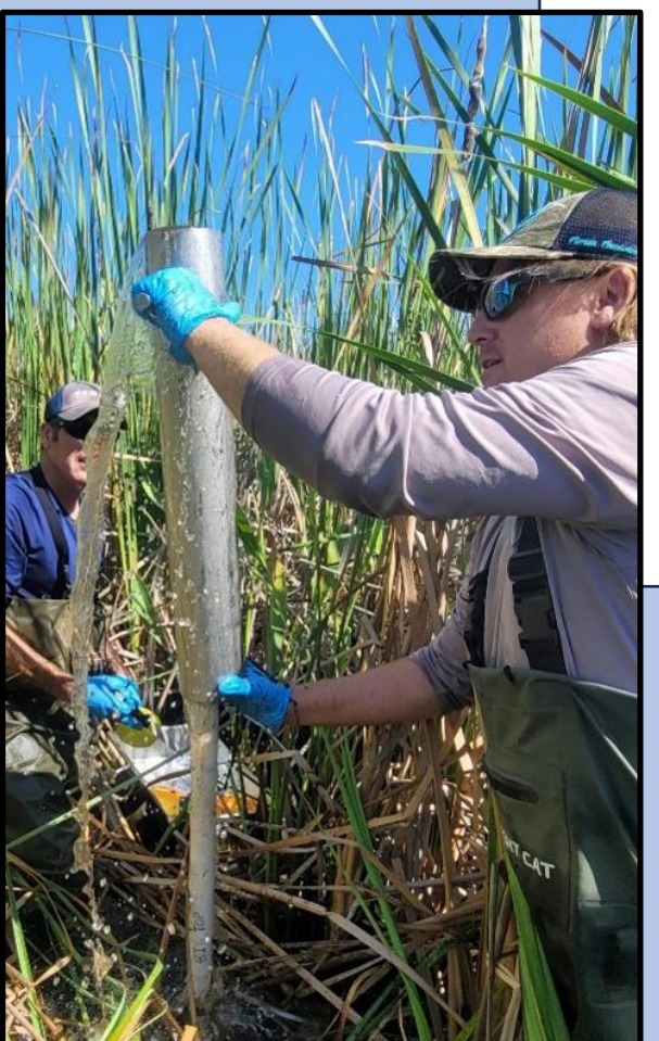
SEDIMENT Sediment sampling using coring tube at FS transect in WCA-2A.
