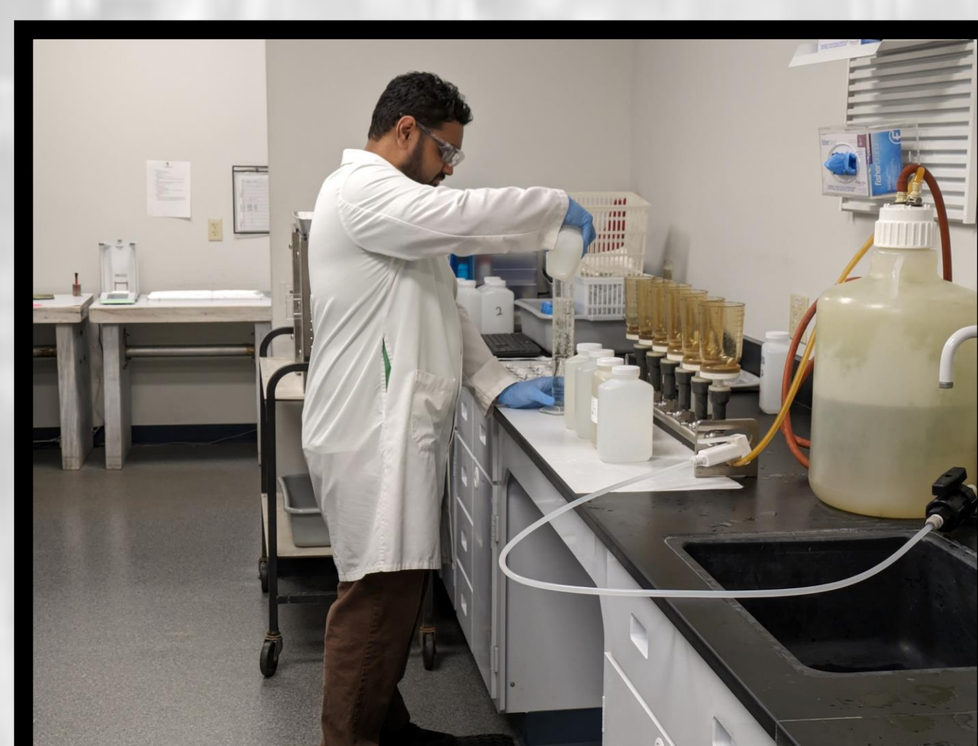
Total Suspended Solids: Chemist performing gravimetric analysis, a labor-intensive physical analysis to determine the amount of suspended matter in a fixed volume of a sample of surface water.
