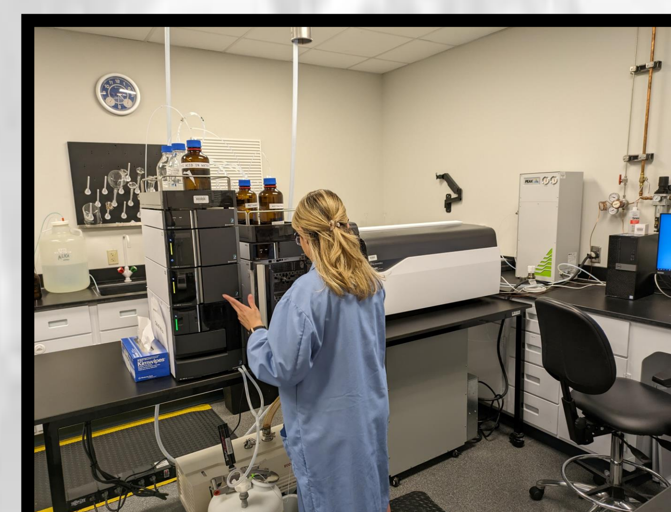
Algal Toxins: Chemist performing maintenance on a new LC MS/MS instrument used by SFWMD to analyze algal toxins.
