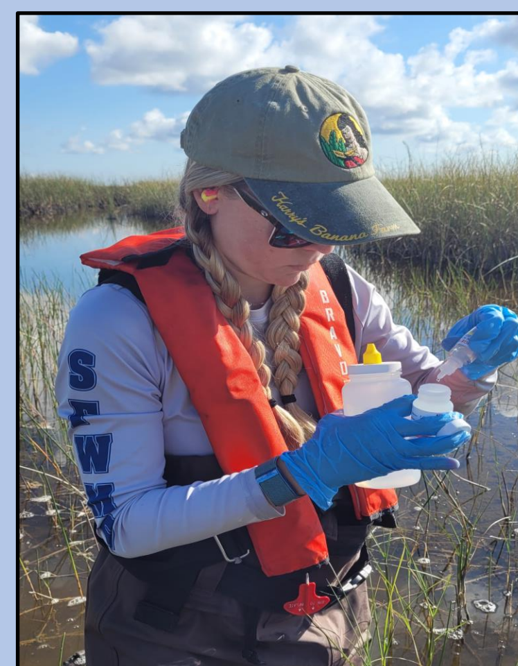
Sample preservation with acid at Station CA39 in WCA-3A.
