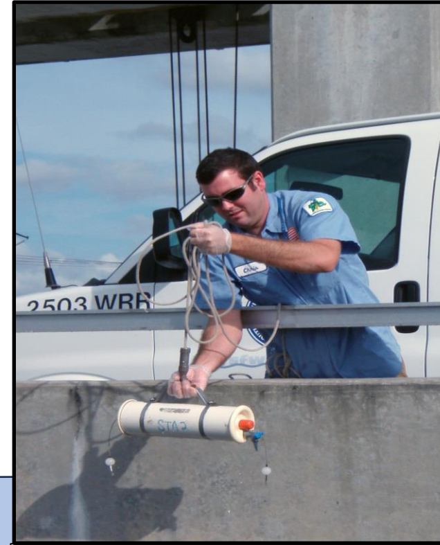
TRUCK S5A-E on the C-51 Canal. Collection of samples upstream of the gates using a Van Dorn.
