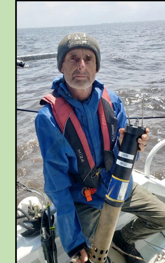
KBRN Platform in the Kissimmee River. Swapping out continuous monitoring instruments.
