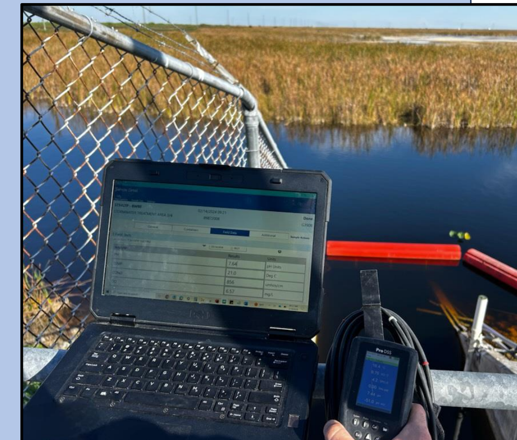
At Station G390B in STA-3/4, field observations and instrument data are entered directly into computer to maximize efficiency and minimize errors through built-in cross-checks, which then are uploaded directly into the Laboratory Information Management System (LIMS).
