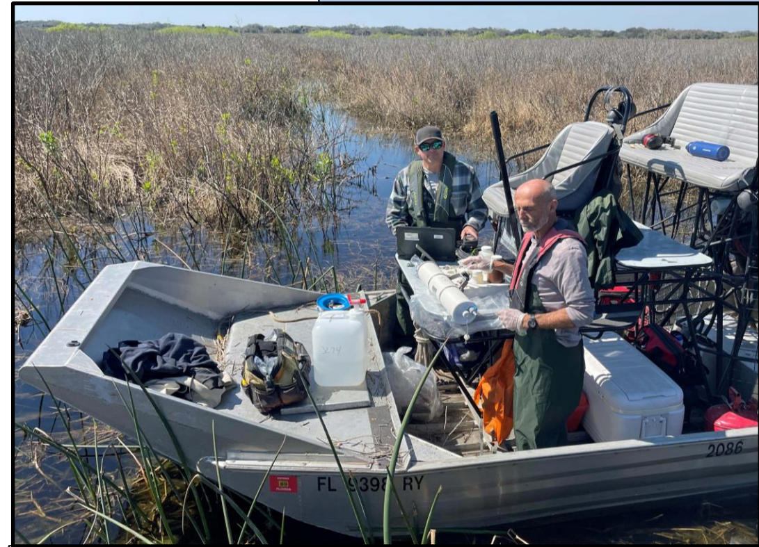
AIRBOAT Station PC34 on the Kissimmee River floodplain. Collection of surface water samples and multi-parameter sonde data.
