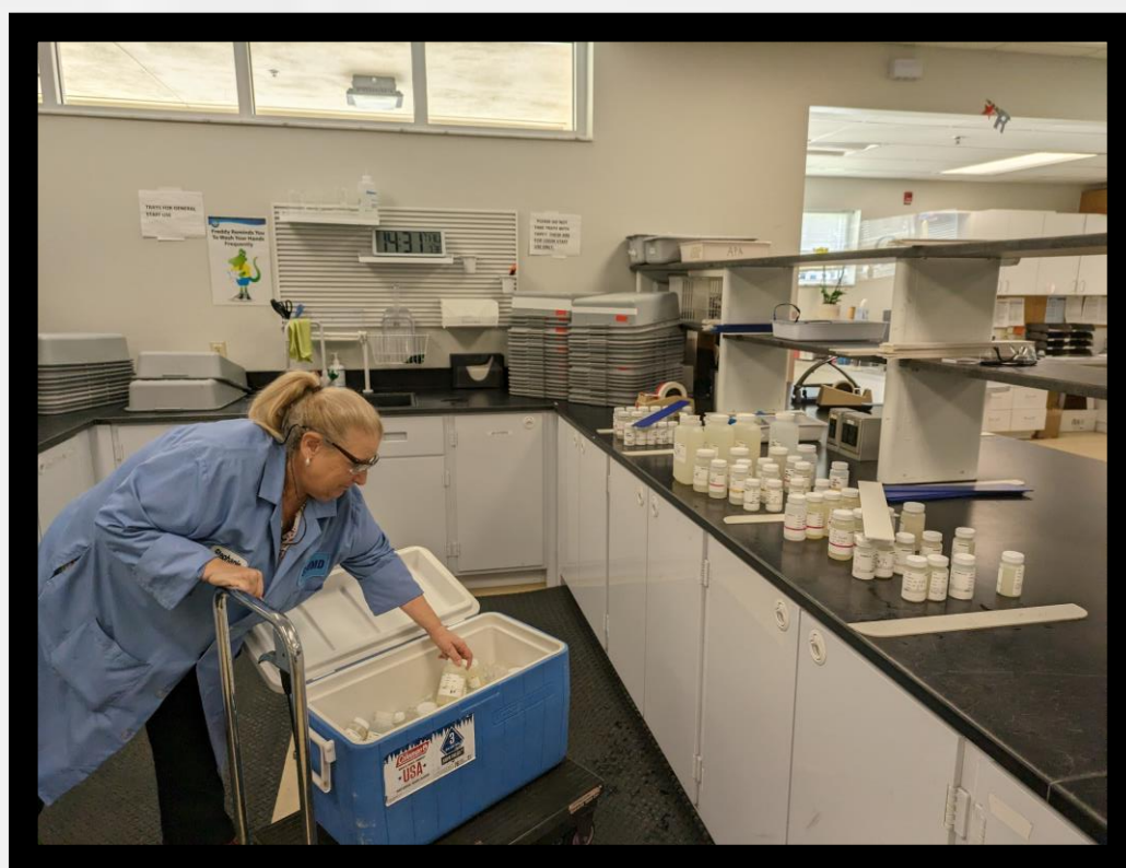
Login analyst verifying number of samples and sample pH during sample receiving.
