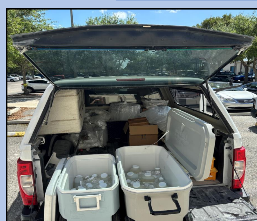
Samples are preserved (filtered, acidified, or chilled) in the field and ready for transport.
