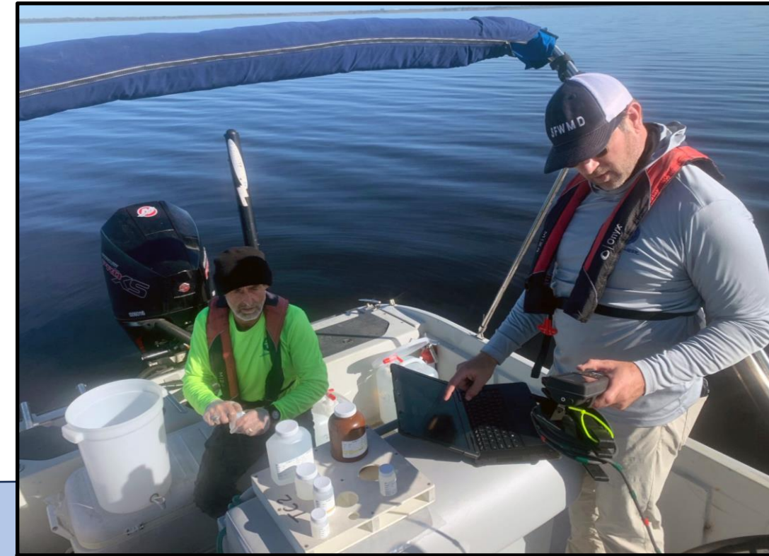
BOAT Station A03 in East Lake Tohopekaliga. Collection of surface water samples and multi-parameter sonde data.
