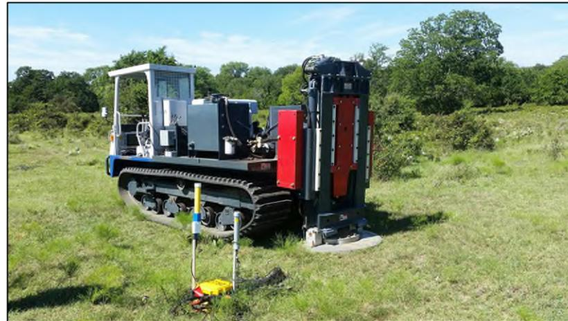
Accelerated Impact Seismic Source
