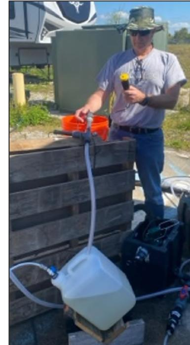
**Purging and displacement anoxic water sample collection system**
