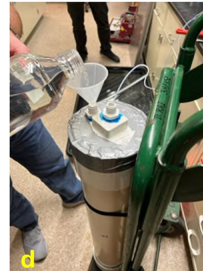
Collecting water samples (a,b), preparing and replacing headspace in core chamber prior to resealing PNNL-7 (c,d) at PNNL lab facility, Richland, WA on 28-Mar-2024.
