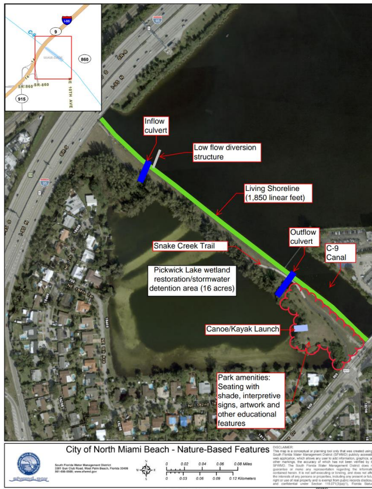
Figure 9-7: Pickwick Lake wetland restoration/stormwater detention area features.
