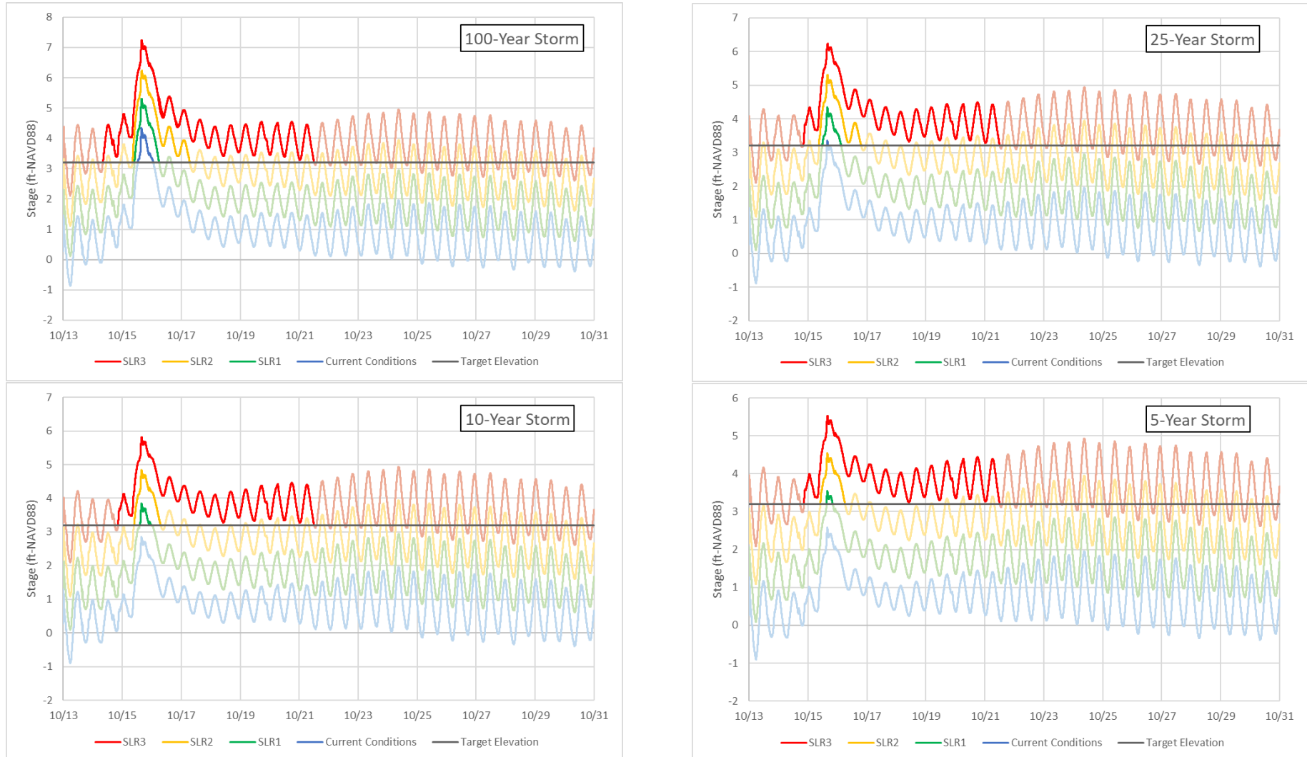
Figure 9-228. Flood Duration for the C5 Watershed as Determined at MRMS1
