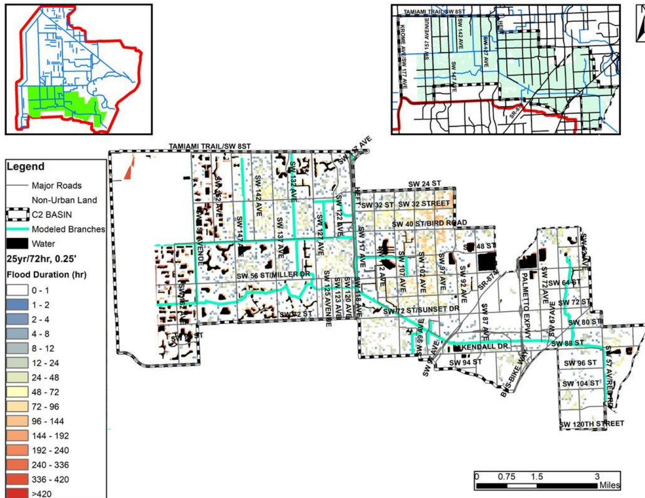
Figure 9-60. Flood Duration Map for the Current Conditions 25-year 3-day Design Storm for Urban Areas in the C2 Watershed
