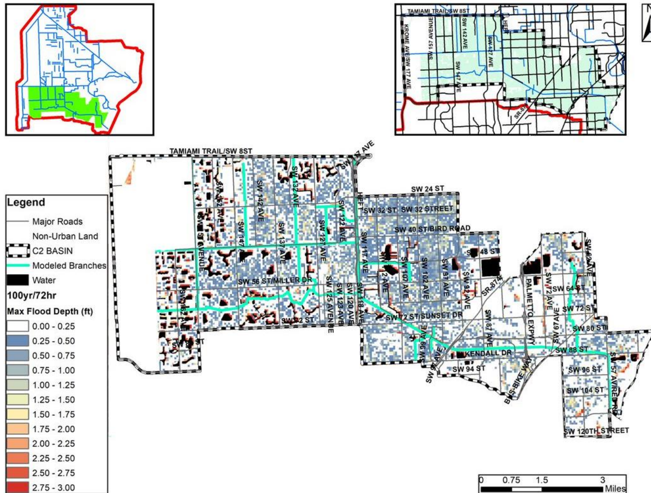
Figure 9-44. Maximum Overland Flood Depth for the Current Conditions 100-year 3-Day Design Storm for Urban Areas in the C2 Watershed
