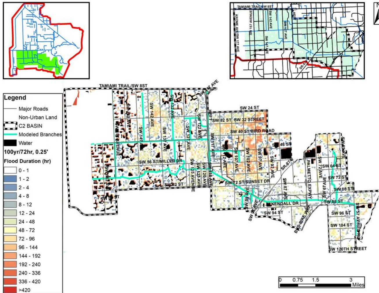
Figure 9-61. Flood Duration Map for the Current Conditions 100-year 3-day Design Storm for Urban Areas in the C2 Watershed
