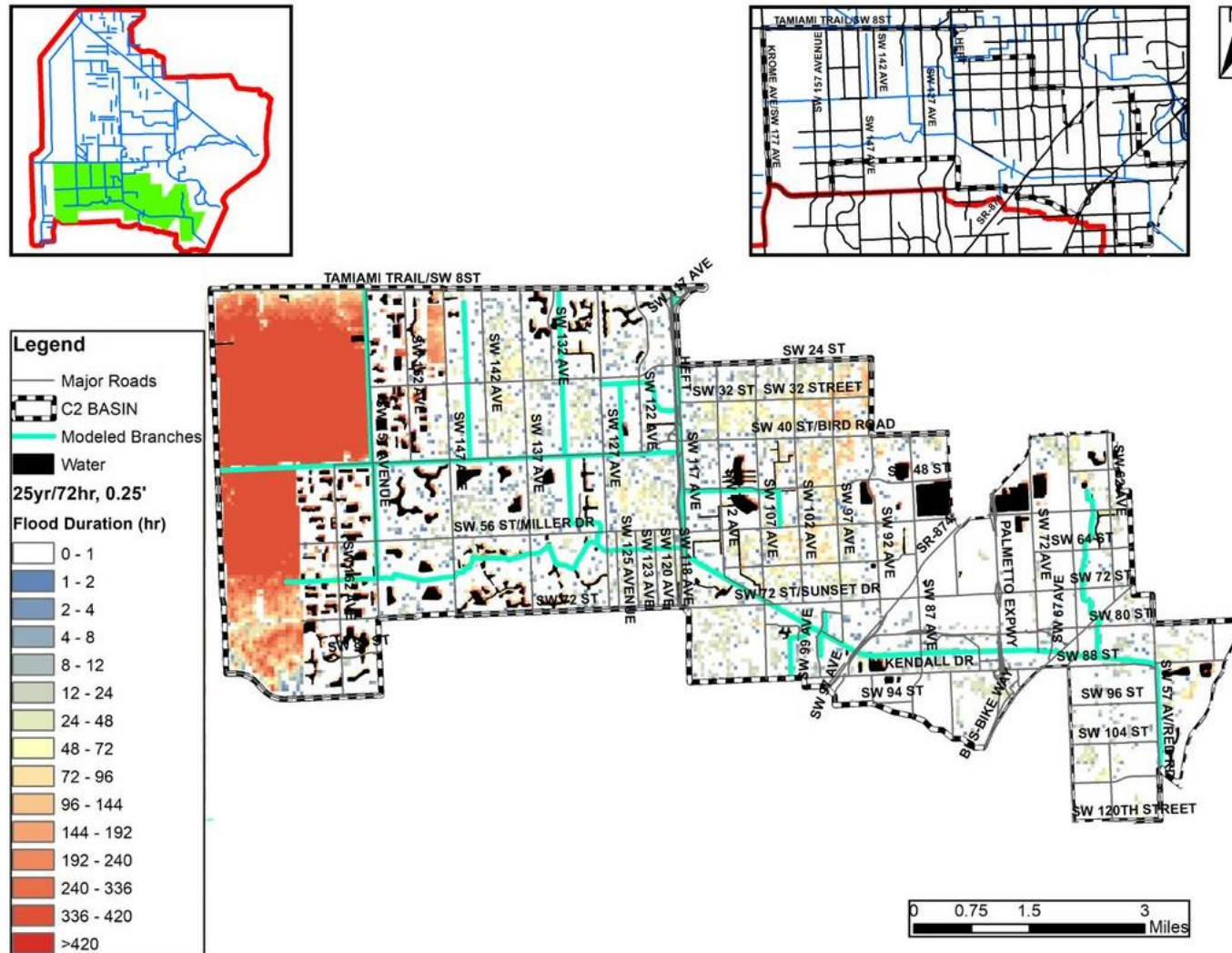
Figure 9-58. Flood Duration Map for the Current Conditions 25-year 3-day Design Storm for the C2 Watershed
