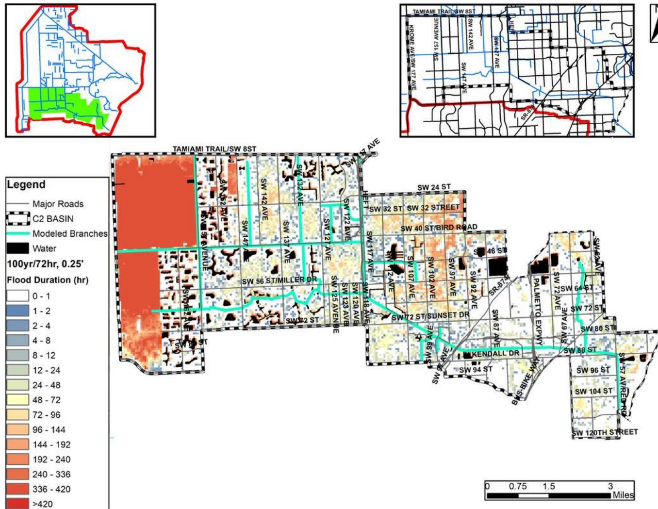
Figure 9-59. Flood Duration Map for the Current Conditions 100-year 3-day Design Storm for the C2 Watershed
