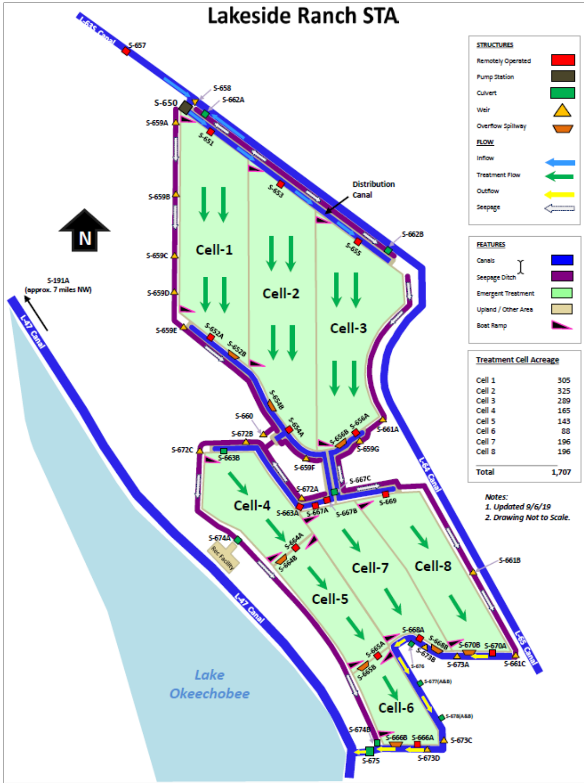
Figure 7-4. Lakeside Ranch STA structures, flows, and features.
