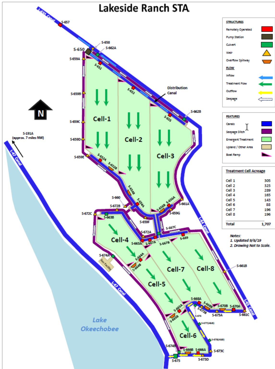
Figure 7-4. Lakeside Ranch STA structures, flows, and features.
