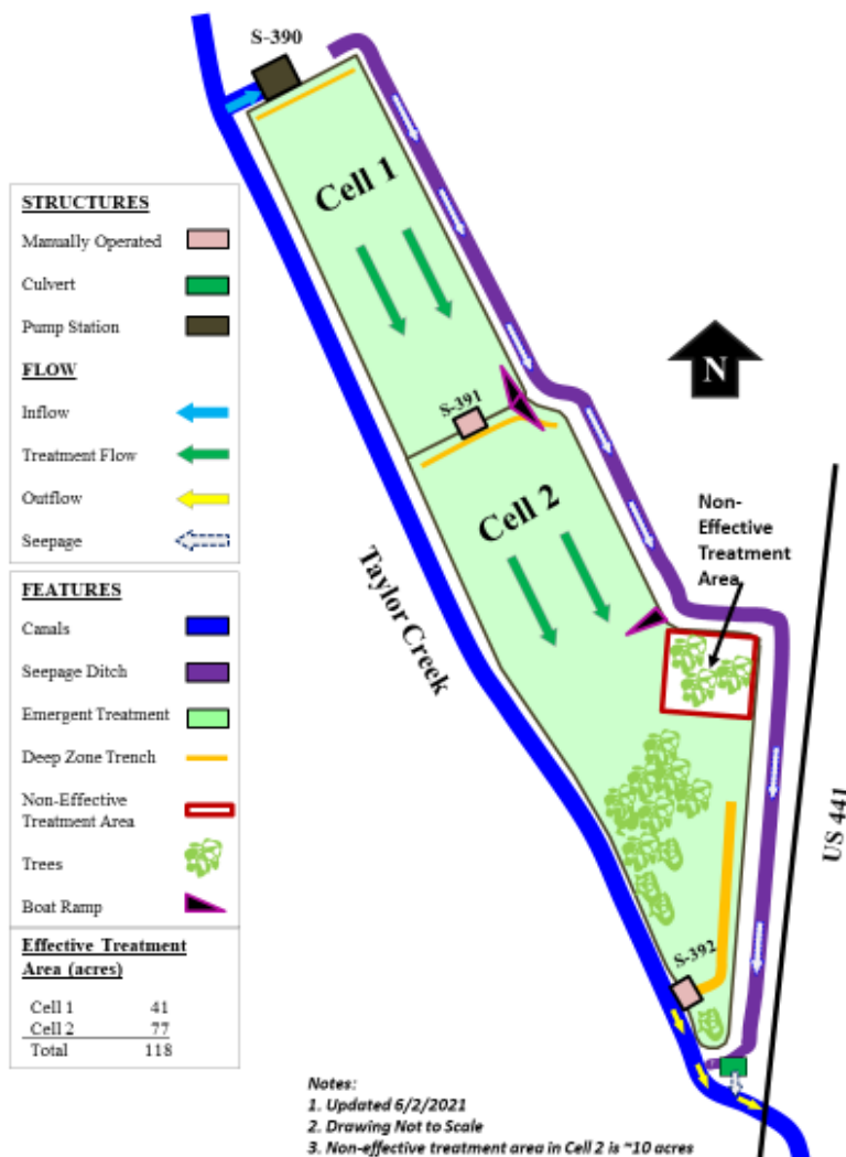
Figure 7-2. Taylor Creek STA structures, flows, and features.
