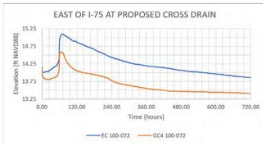
Figure 121 Comparison of Stage Hydrographs for the 100-year 72-hour Storms on the Intake Side of the Proposed I-75 Cross Drain
