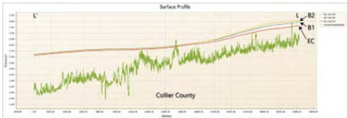
Figure 160 Comparison of Water Surface Profiles Along Flow Path L' – L for Existing Conditions (EC), and Berm Alignments B1 and B2
