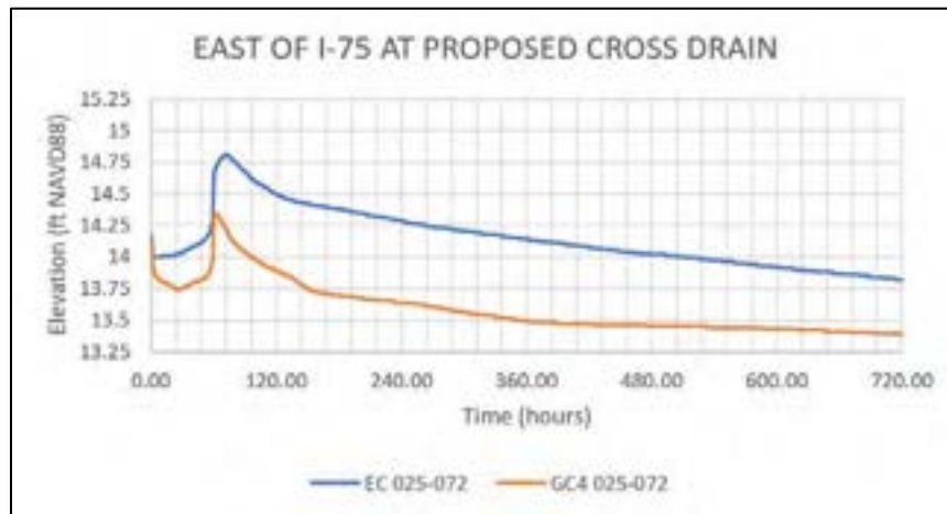
Figure 120 Comparison of Stage Hydrographs for the 25-year 72-hour Storms on the Intake Side of the Proposed I-75 Cross Drain
