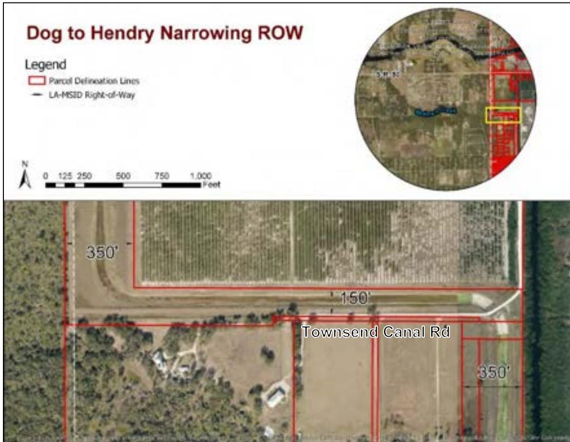
Figure 12 - Narrowing of LA-MSID Right-of-Way from 350' to 150'
