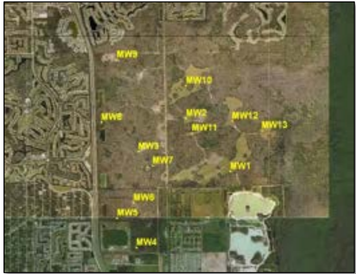
Figure 39 Hidden Cypress and Larry Kiker Preserves Groundwater Monitoring Wells
