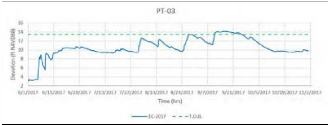
Figure 67 Existing Condition (EC) Simulated Stage Hydrograph at Location PT-03 for Calibration Period
