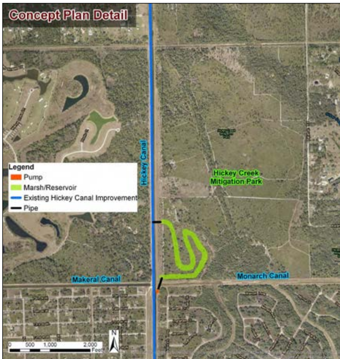
Figure 38 - Example of a water quality filter marsh area, 1.1.9 Charlie Diversion-Hickey Canal Improvement
