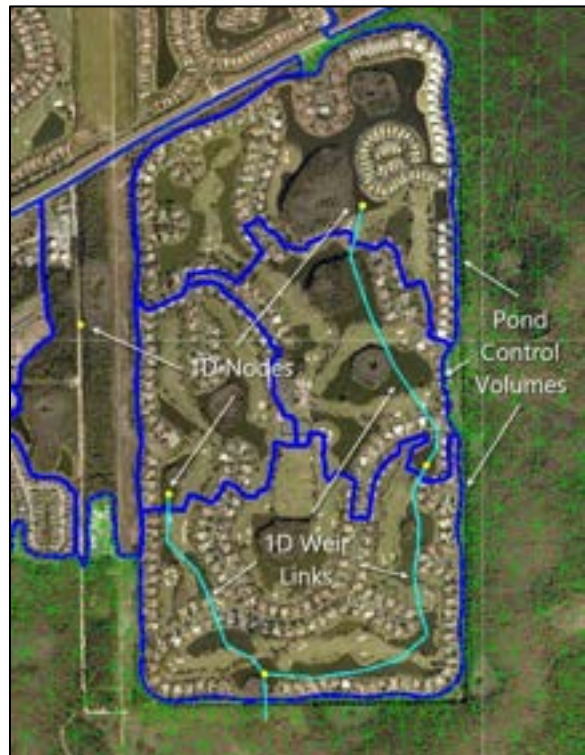
Figure 15 Example of Pond Control Volumes
