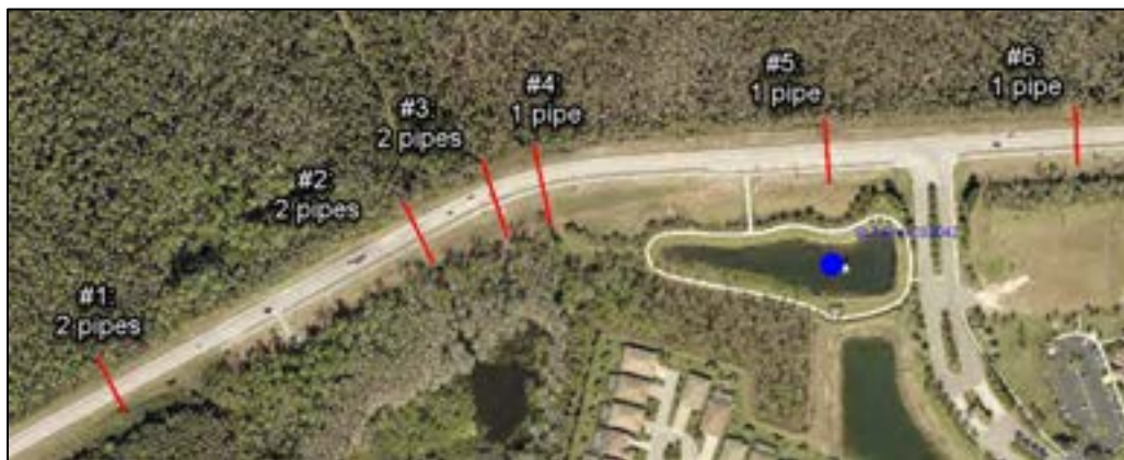
Figure 106 Existing Cross Drains Along Corkscrew Road
