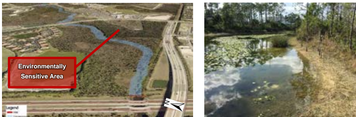
Figure 1 - Examples of winding high-capacity flow paths functioning as deep marshes during non-emergency conditions.
