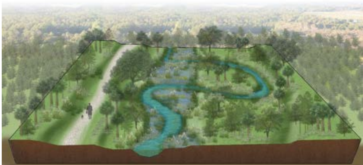
Figure 20 – Three-dimensional representation of a shallow littoral bench to provide a direct conveyance pathway with increased conveyance capacity during large storm events.
