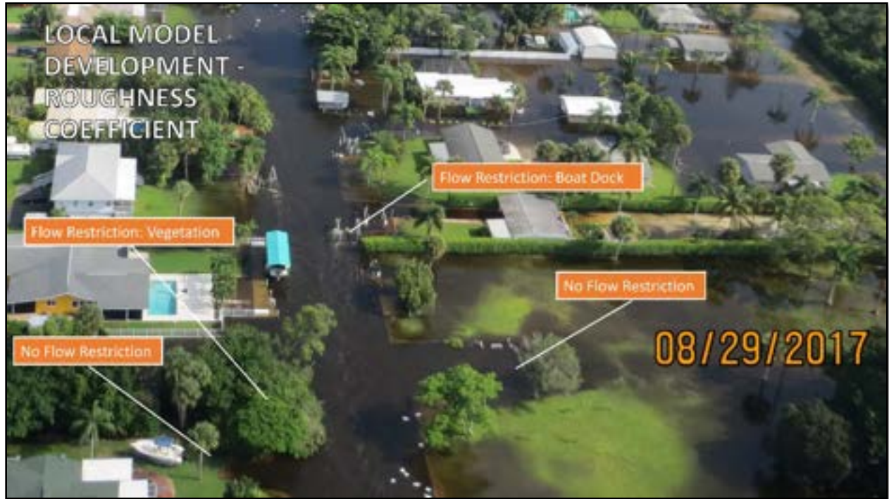
Figure 1 - Example of vegetation and boat dock obstructions within the main channel of Ten Mile Canal at STA 127+00 causing restrictions to flow. Also shown are two off-channel boat access designs that do not cause flow restrictions. Photograph taken by Mark White, SFWMD.
