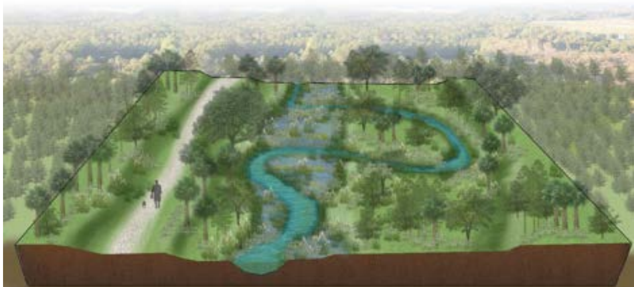
Figure 4 – Three-dimensional representation of a shallow littoral bench to provide a direct conveyance pathway with increased conveyance capacity during large storm events.
