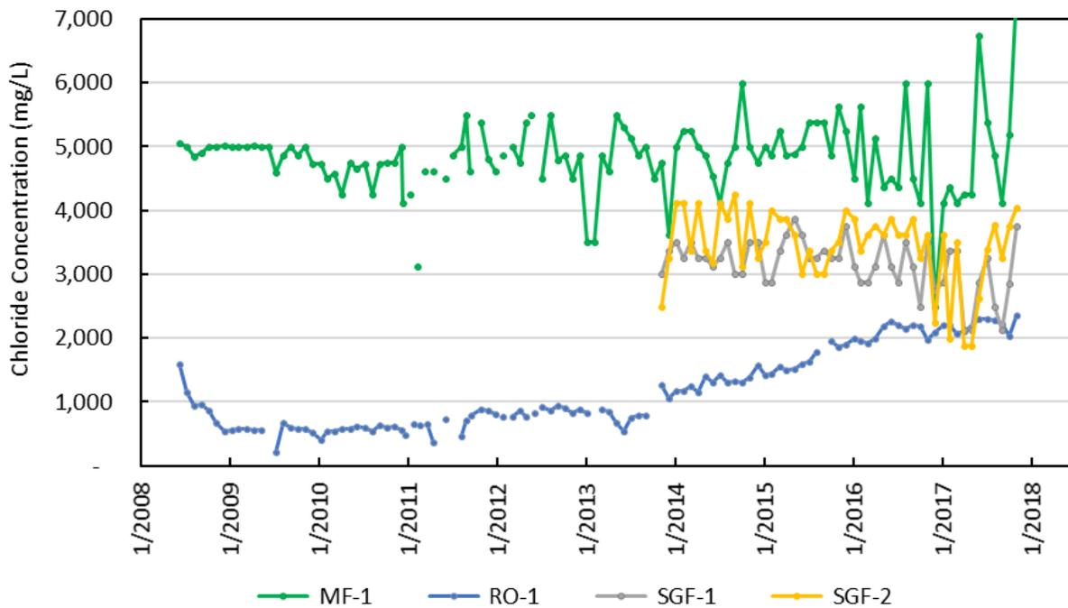
Figure D-47. Chloride concentrations in City of Sunrise Floridan aquifer system wells: MF-1 and RO-1 are completed in the Upper Floridan aquifer, while SGF-1 and SGF-2 are completed in the Upper Floridan aquifer/Avon Park Permeable Zone.
