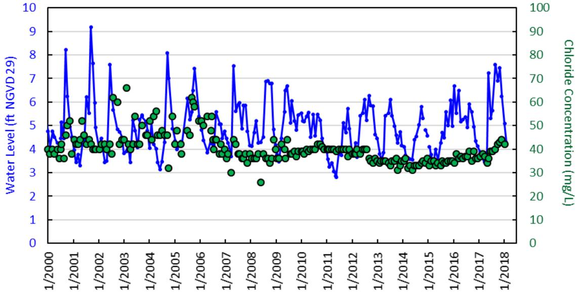
Figure D-17. Water levels and chloride concentrations in monitor well PB-1669 (131 feet deep) in Boca Raton, southeastern Palm Beach County.
