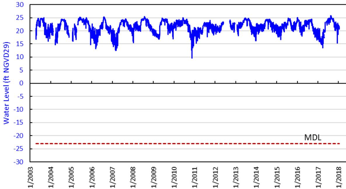
Figure D-9. Water levels in the Lower Tamiami aquifer at well HE-859 (59 feet deep) in eastern Hendry County.
