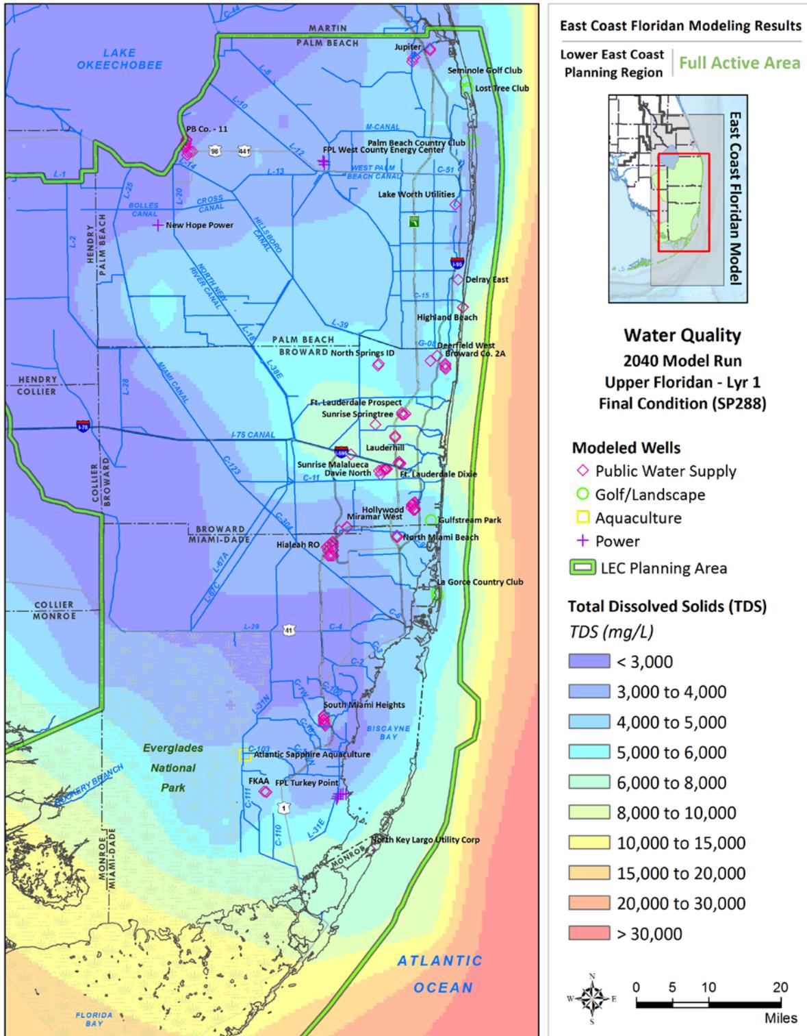
Figure D-59. Water quality (total dissolved solids) at the end of the modeling period (month 288) using 2040 demand projections in the Upper Floridan aquifer (Layer 1).
