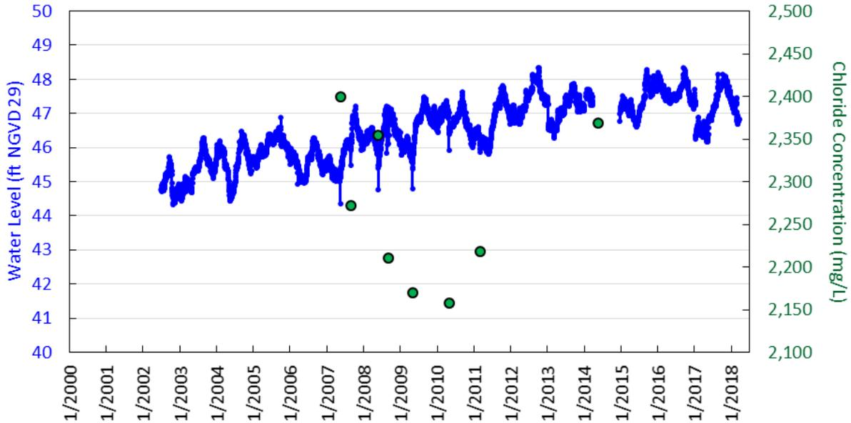
Figure D-39. Water levels and chloride concentrations in Avon Park Permeable Zone monitor well BF-4M, eastern Broward County.
