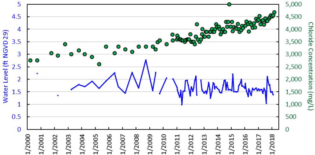
Figure D-26. Water levels and chloride concentrations in monitor well F-279 (116 feet deep) in North Miami, northeastern Miami-Dade County.
