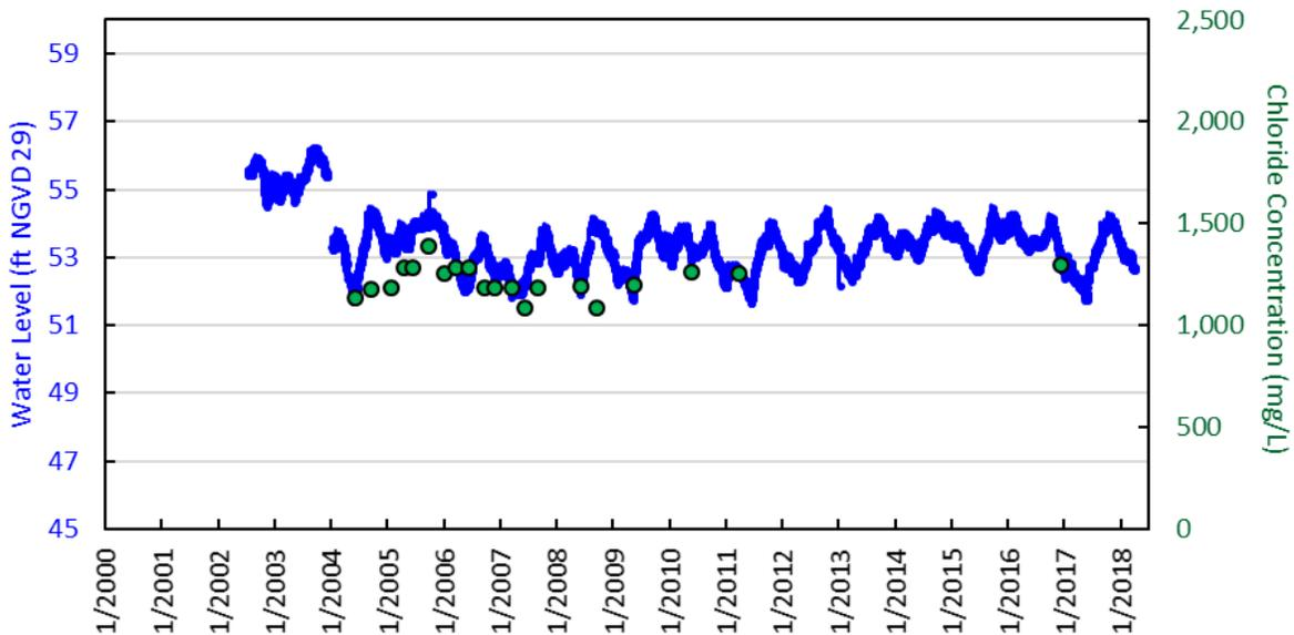
Figure D-35. Water levels and chloride concentrations in Upper Floridan aquifer monitor well PBF-7U (1,447 feet deep), western Palm Beach County.
