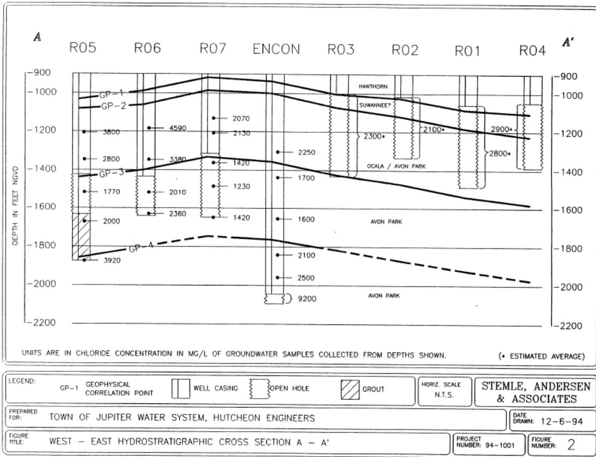
Figure D-42. Hydrogeologic cross-section of Town of Jupiter Floridan aquifer system wells R01 to R07 (From: Stemle, Andersen & Associates, Inc. 1994).
