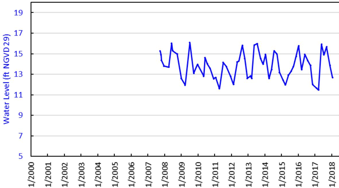
Figure D-2. Water levels in the surficial aquifer system at well PB-685 (17 feet deep) in Loxahatchee, central Palm Beach County.
