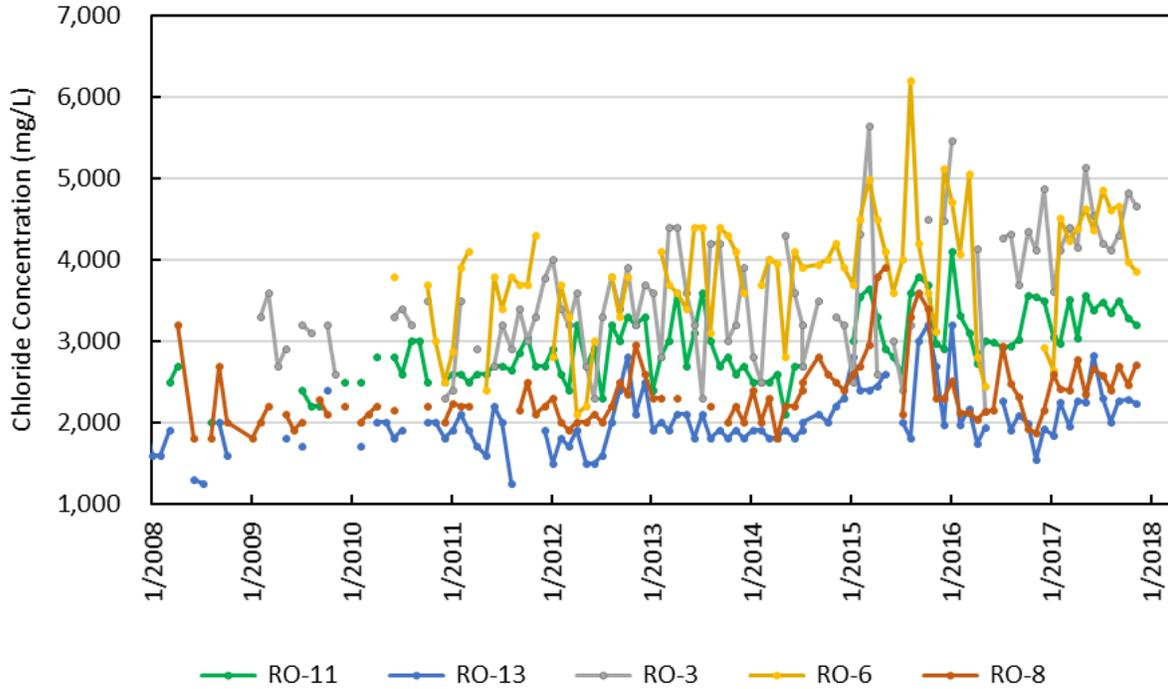
Figure D-43. Chloride concentrations in Town of Jupiter Floridan aquifer system wells RO-6 and RO-8 in the Avon Park Permeable Zone and wells RO-3, RO-11, and RO-13 in both the Upper Floridan aquifer and Avon Park Permeable Zone.
