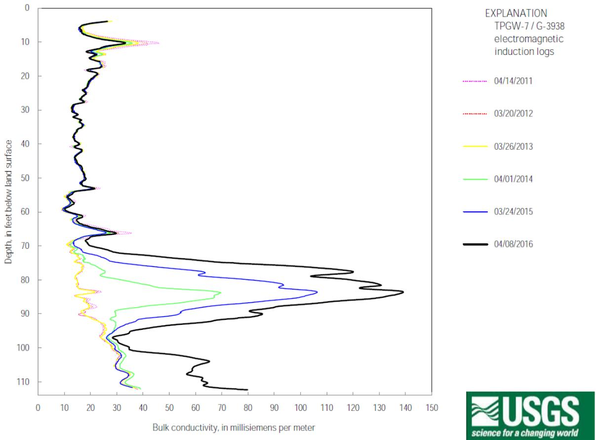
Figure D-32. Induction logs for monitor well TPGW-7D (84 feet deep) in Homestead, southeastern Miami-Dade County (From: Valderrama 2017).
