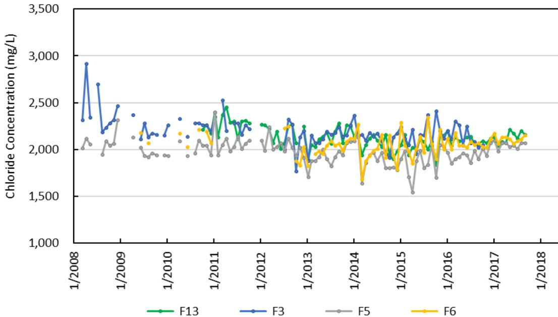
Figure D-48. Chloride concentrations in City of Hollywood Floridan aquifer system (Upper Floridan aquifer) wells 3, 5, 6, and 13.
