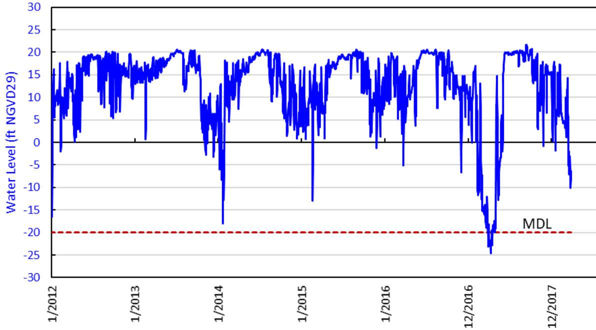
Figure D-7. Water levels in the Lower Tamiami aquifer at well HES-26D (100 feet deep) in eastern Hendry County.
