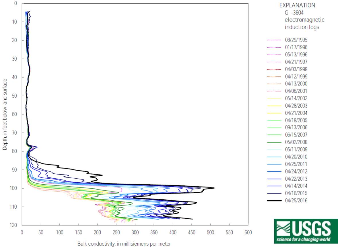
Figure D-28. Induction logs for monitor well G-3604 (120 feet deep) near Miami Springs, east-central Miami-Dade County (From: Valderrama 2017).
