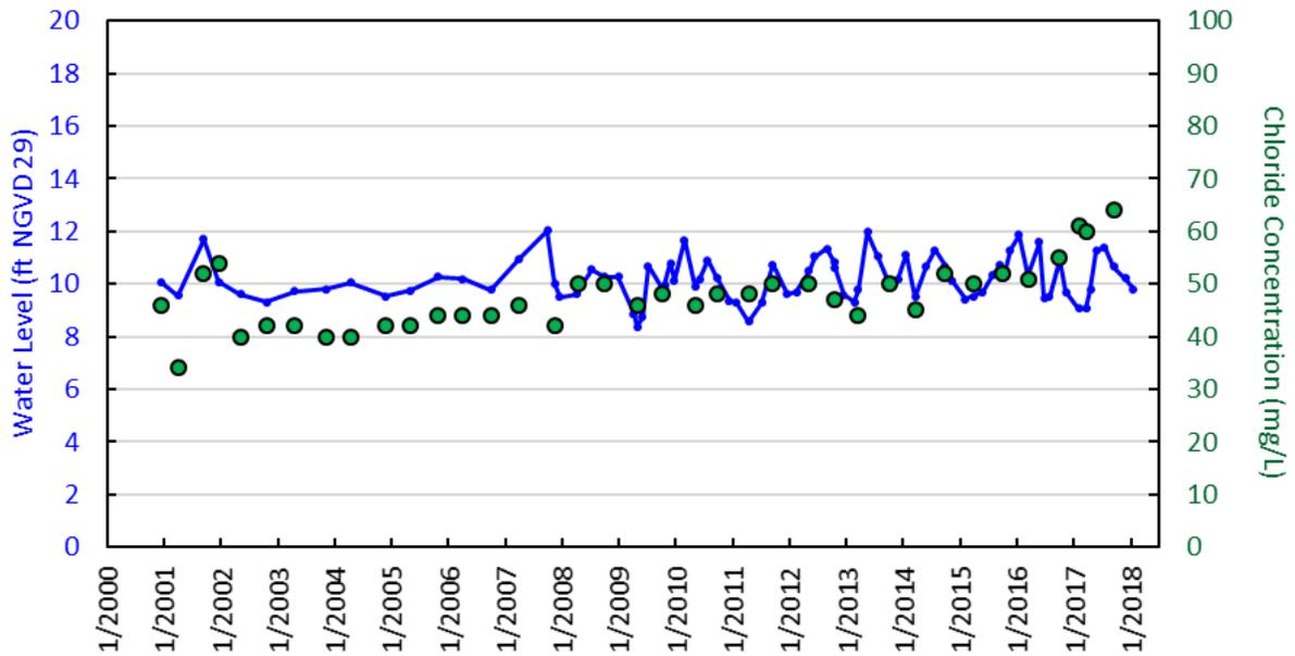
Figure D-13. Water levels and chloride concentrations in monitor well PB-809 (150 feet deep) in West Palm Beach, east-central Palm Beach County.
