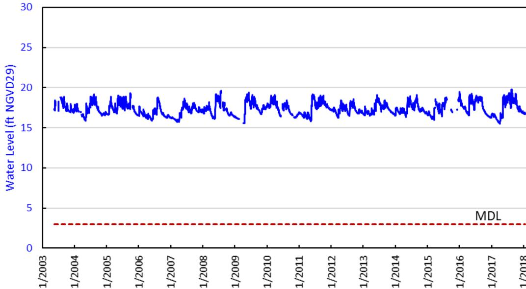
Figure D-11. Water levels in the Lower Tamiami aquifer at well HE-1068 (160 feet deep) in northeastern Hendry County.
