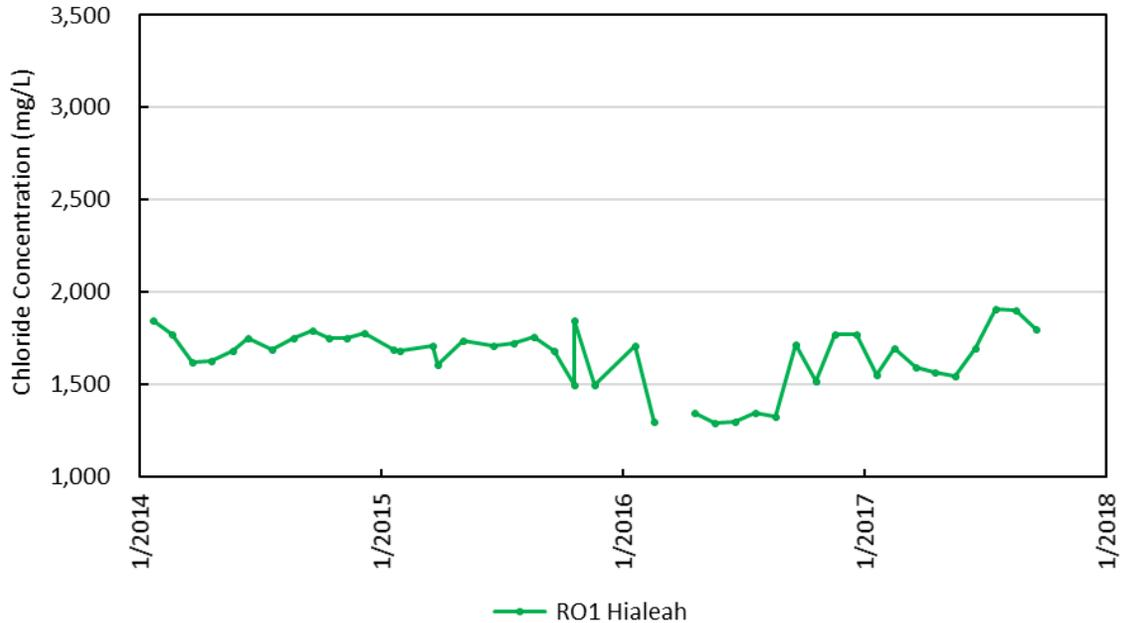
Figure D-49. Chloride concentrations in Miami-Dade Water and Sewer Department Floridan aquifer system (Upper Floridan aquifer) well RO1 Hialeah.
