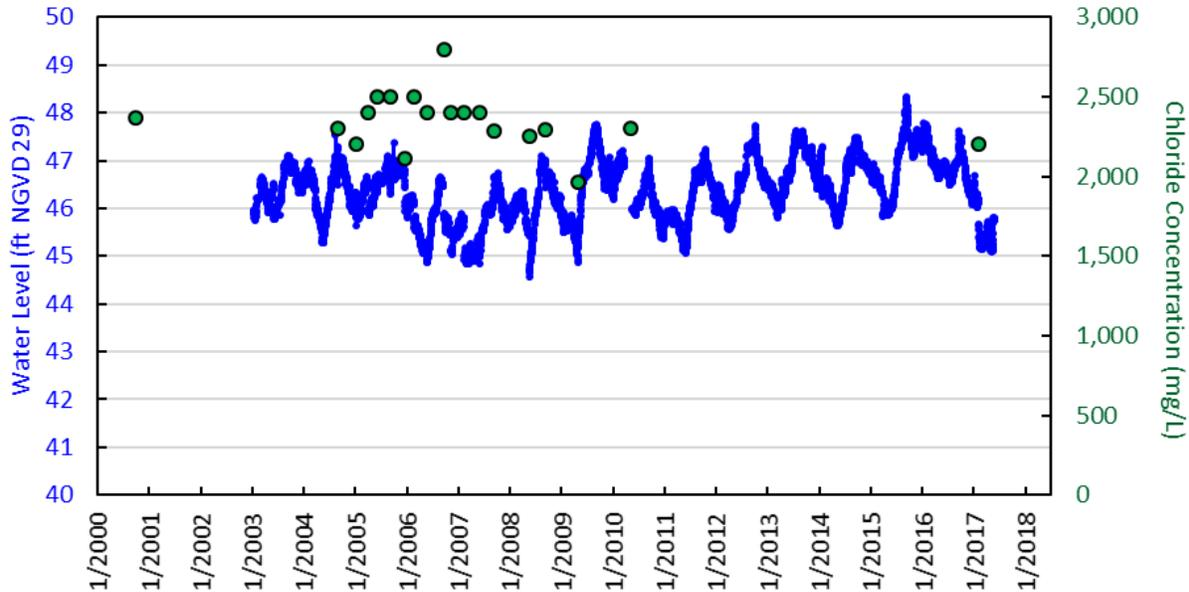
Figure D-34. Water levels and chloride concentrations in Upper Floridan aquifer monitor well PBF-3 (1,252 feet deep), eastern Palm Beach County.
