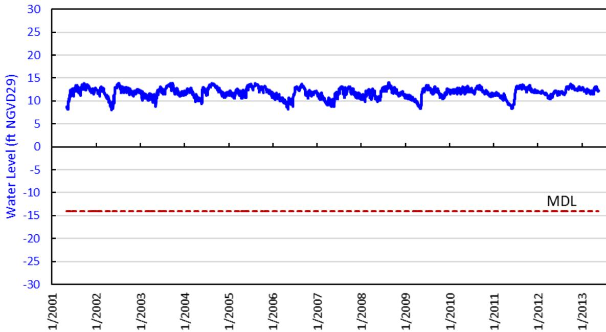
Figure D-10. Water levels in the Lower Tamiami aquifer at well HE-861 (70 feet deep) in southeastern Hendry County.
