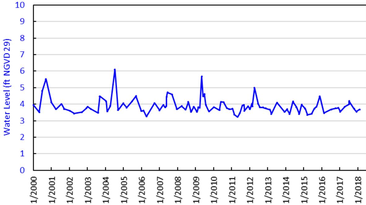
Figure D-3. Water levels in the surficial aquifer system at well G-617 (29 feet deep) in Davie, central Broward County.
