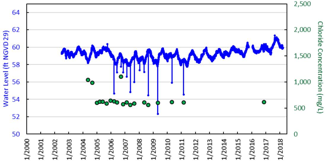
Figure D-36. Water levels and chloride concentrations in Upper Floridan aquifer monitor well G-2618 (1,164 feet deep), western Broward County.
