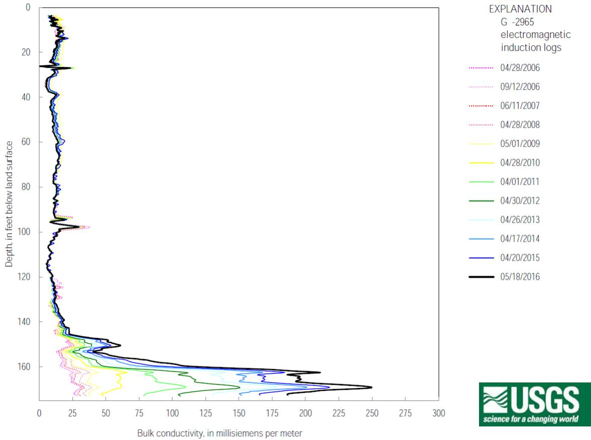
Figure D-23. Induction logs for monitor well G-2965 (175 feet deep) in Hallandale, eastern Broward County (From: Valderrama 2017).
