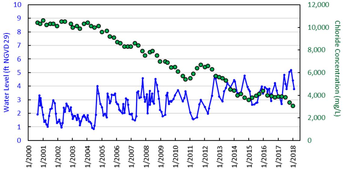
Figure D-16. Water levels and chloride concentrations in monitor well PB-1707 (183 feet deep) in Delray Beach, southeastern Palm Beach County.
