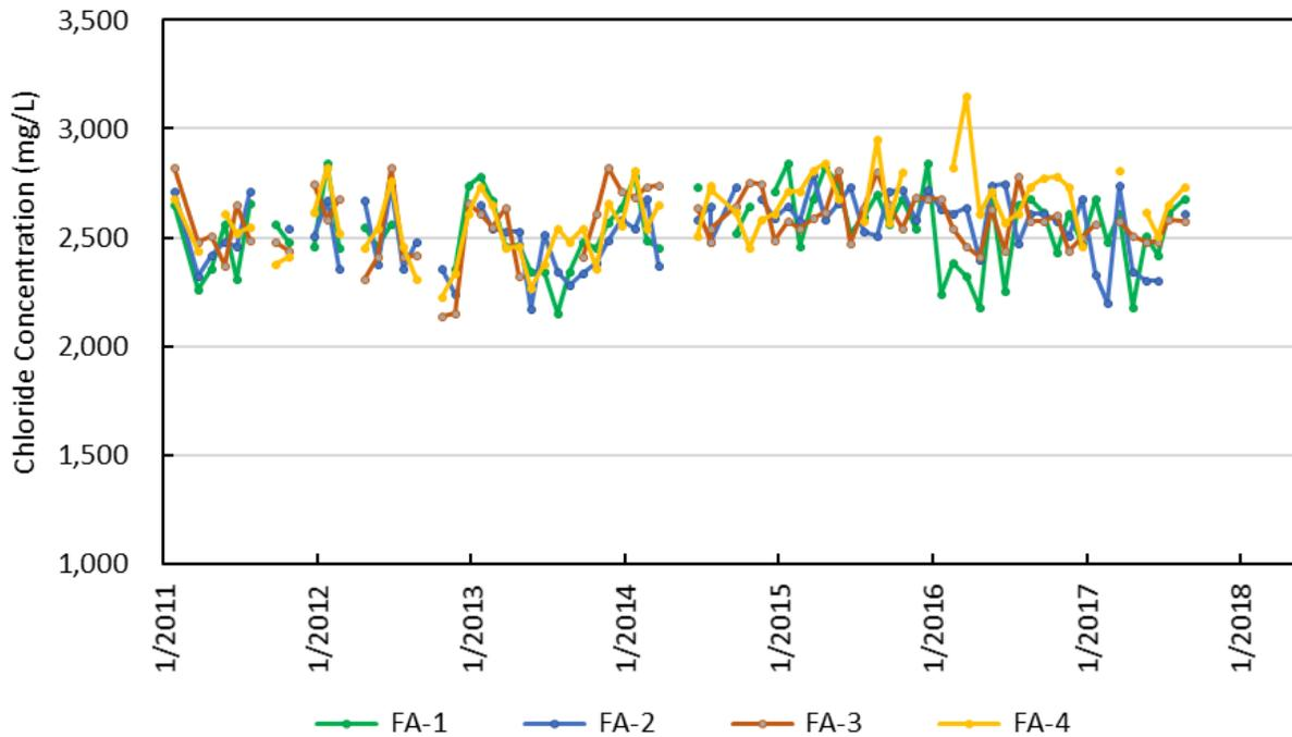
Figure D-50. Chloride concentrations in Florida Keys Aqueduct Authority Floridan aquifer system (Upper Floridan aquifer) wells FA-1 to FA-4.
