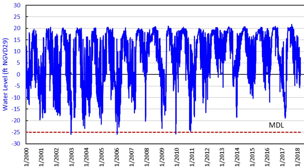
Figure D-6. Water levels in the Lower Tamiami aquifer at well USSUGAR (100 feet deep) in eastern Hendry County.
