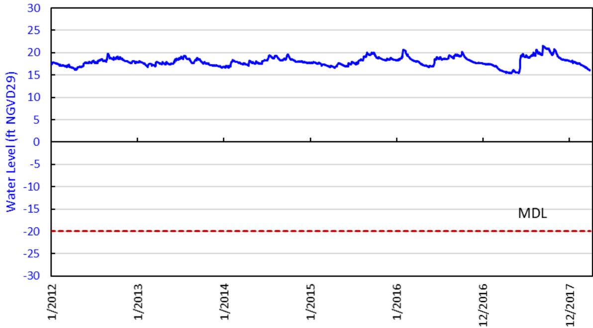
Figure D-8. Water levels in the Lower Tamiami aquifer at well HES-25D (92 feet deep) in eastern Hendry County.
