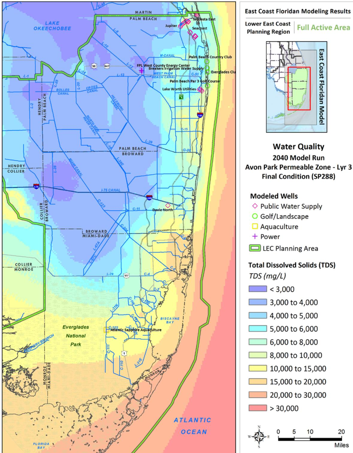
Figure D-61. Water quality (total dissolved solids) at the end of the modeling period (month 288) using 2040 demand projections in the Avon Park Permeable Zone (Layer 3).
