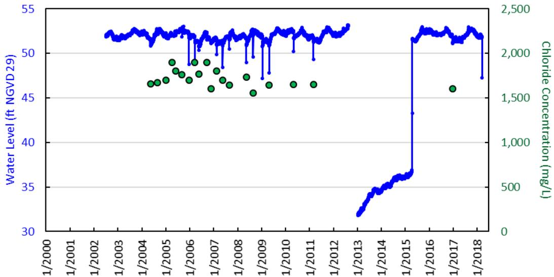
Figure D-37. Water levels and chloride concentrations in Upper Floridan aquifer monitor well DF-4 (1,230 feet deep), northern Miami-Dade County.
