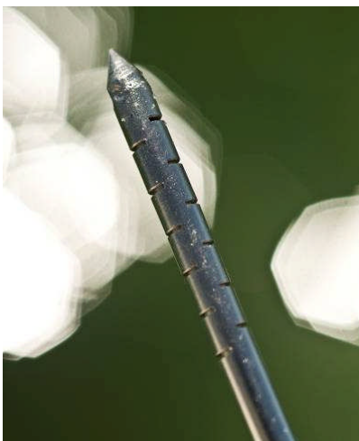
Figure 2-3. The PushPoint Sampler has a Perforated Tip.
