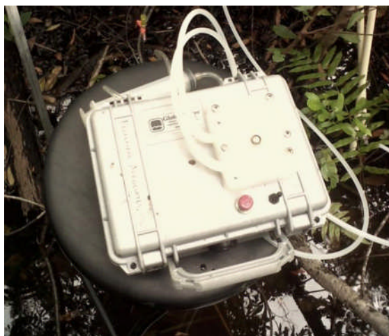
Figure 2-8. Porewater for Analytical Samples was Extracted using a Peristaltic Pump from Two Locations per Point.
