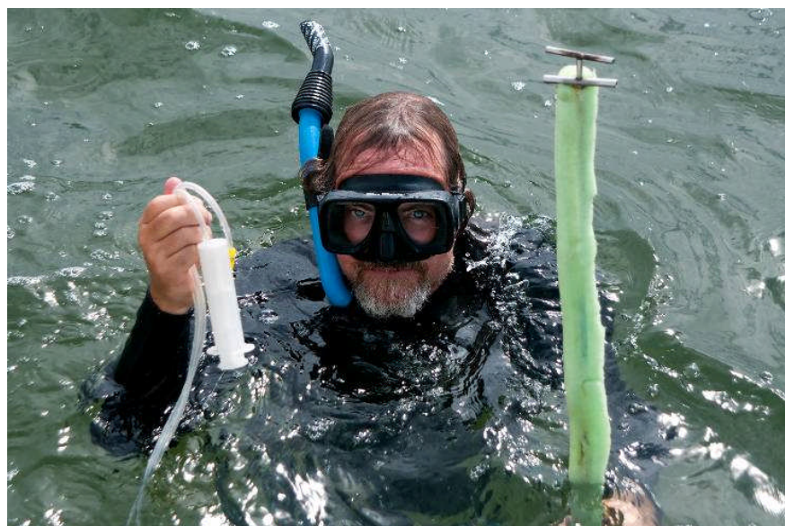
Figure 2-5. Subtidal Porewater was Collected using an Insulated Pushpoint Sampler.
