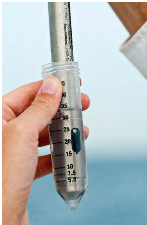
Figure 2-6. A Porewater Sample is Measured by a Technician. Porewater samples were put in a 50 mL cuvette and measured with either an AT100 or AT200 probe.
